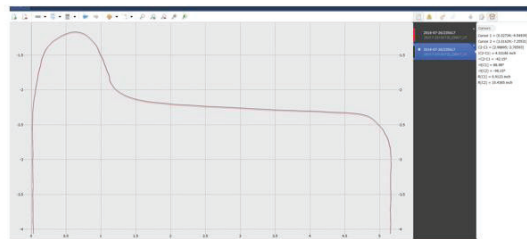
Overlay Exported WheelScan and MiniProf Wheel to Verify Calibration
