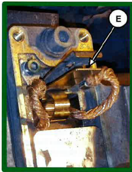
Figure 20-22: Correct Ground Brush Spring Installation E. Retaining Spring
