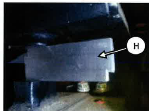
Figure 20-19: Chevron Spring (with shim) Clearance H. Parallel Gauge
