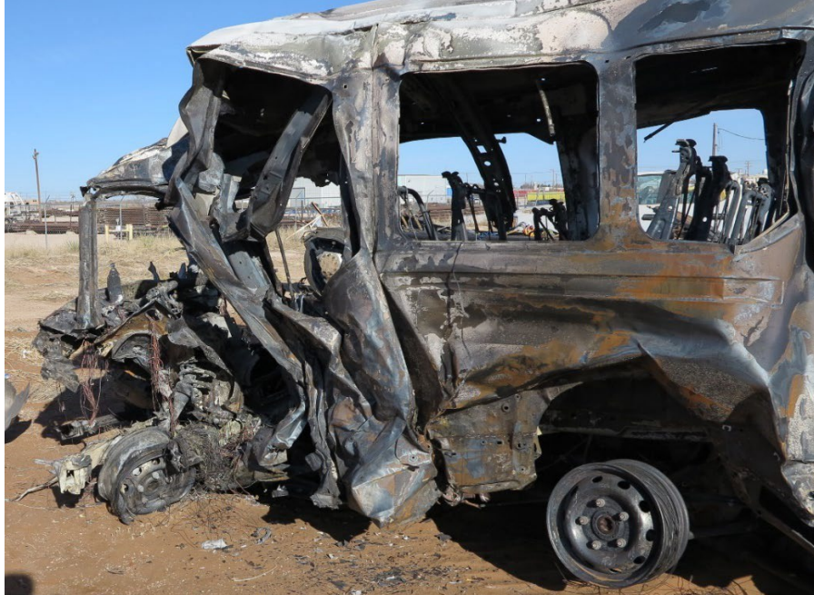
Figure 3: Left-side view of the transit van showing the extensive damage crash and post-crash fire damage.
