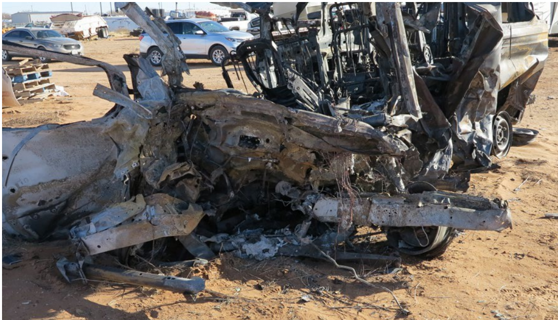
Figure 2: A front view of the 2017 Ford Transit Van showing the extensive crash and post-crash fire damage.
