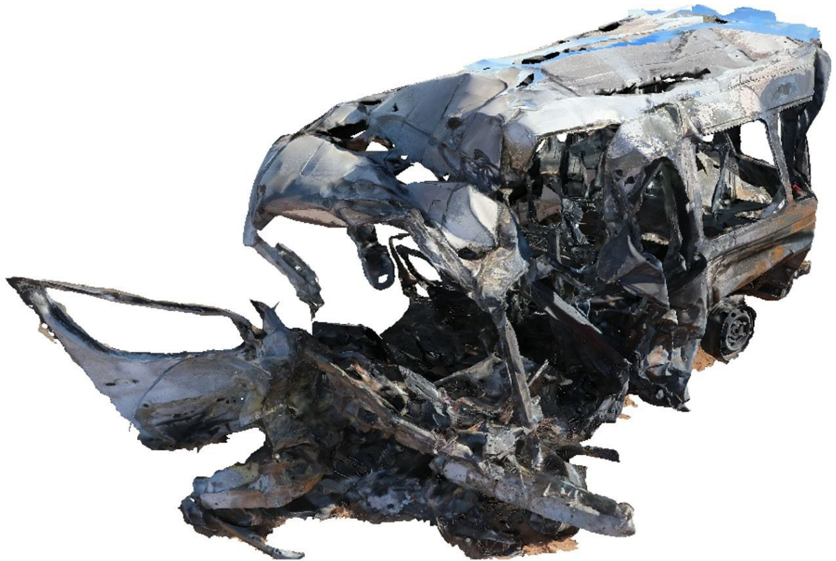
Figure 3. The image shows a 3D view of the Ford looking at the left front of the vehicle where the damage was concentrated.
