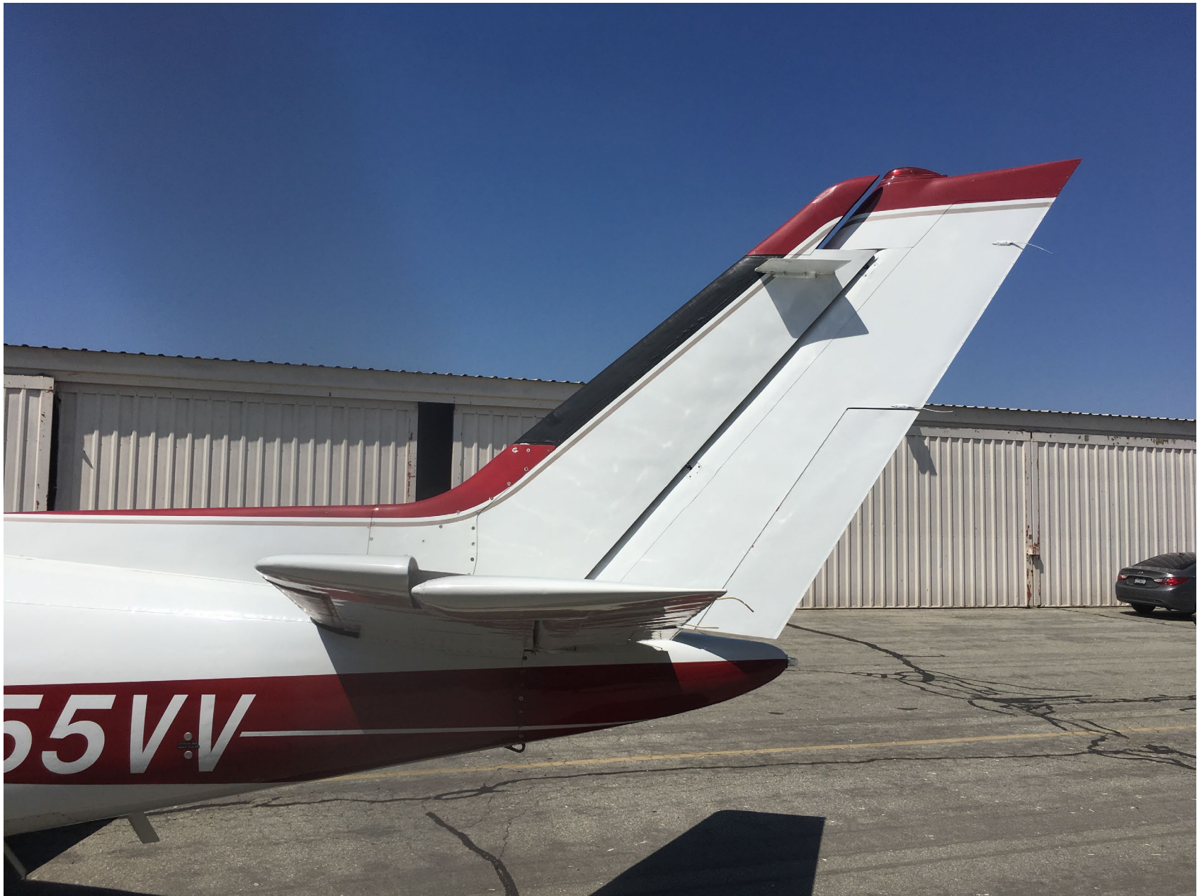
Photo 2 – Exemplar B60 Elevator with Control Lock Installed
