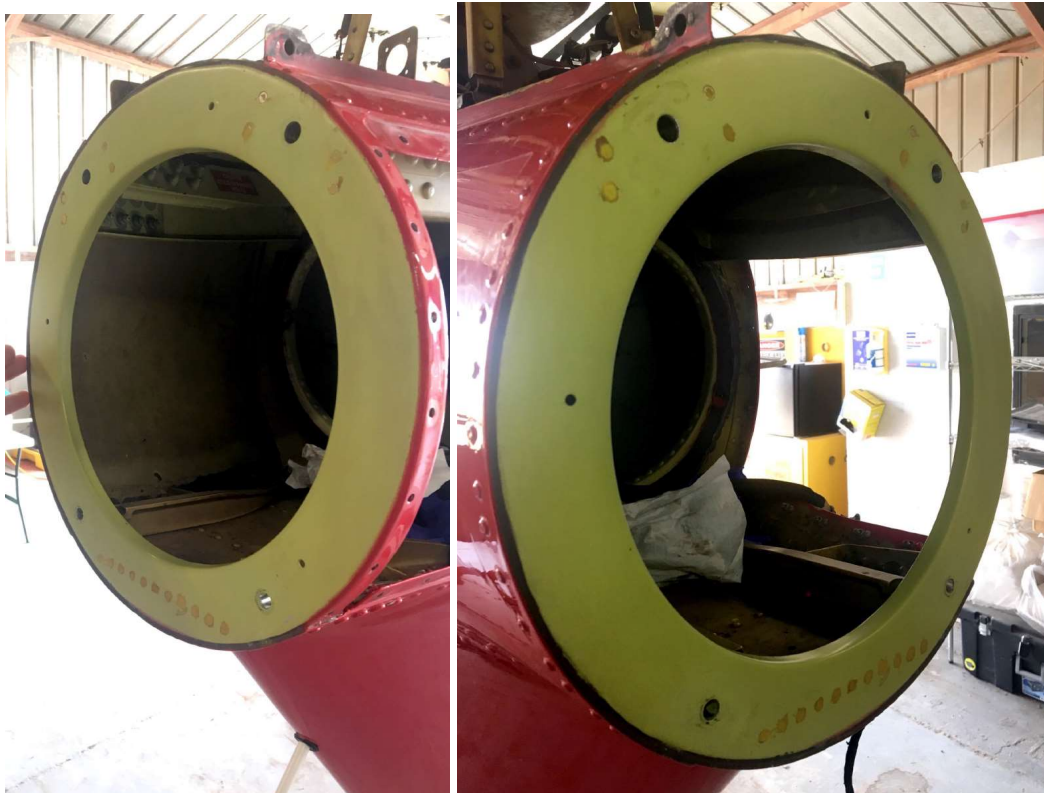
Figure A-1. Two views of the aft fuselage bulkhead. (Image courtesy of Arrow Aviation)
