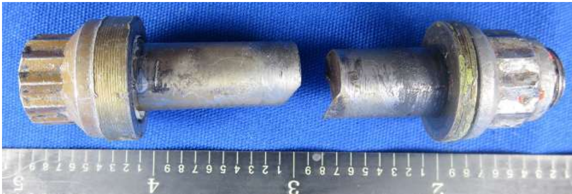
Figure 13. The fractured bolt found on Bell 407 S/N 53563. (Image courtesy of Bell)
