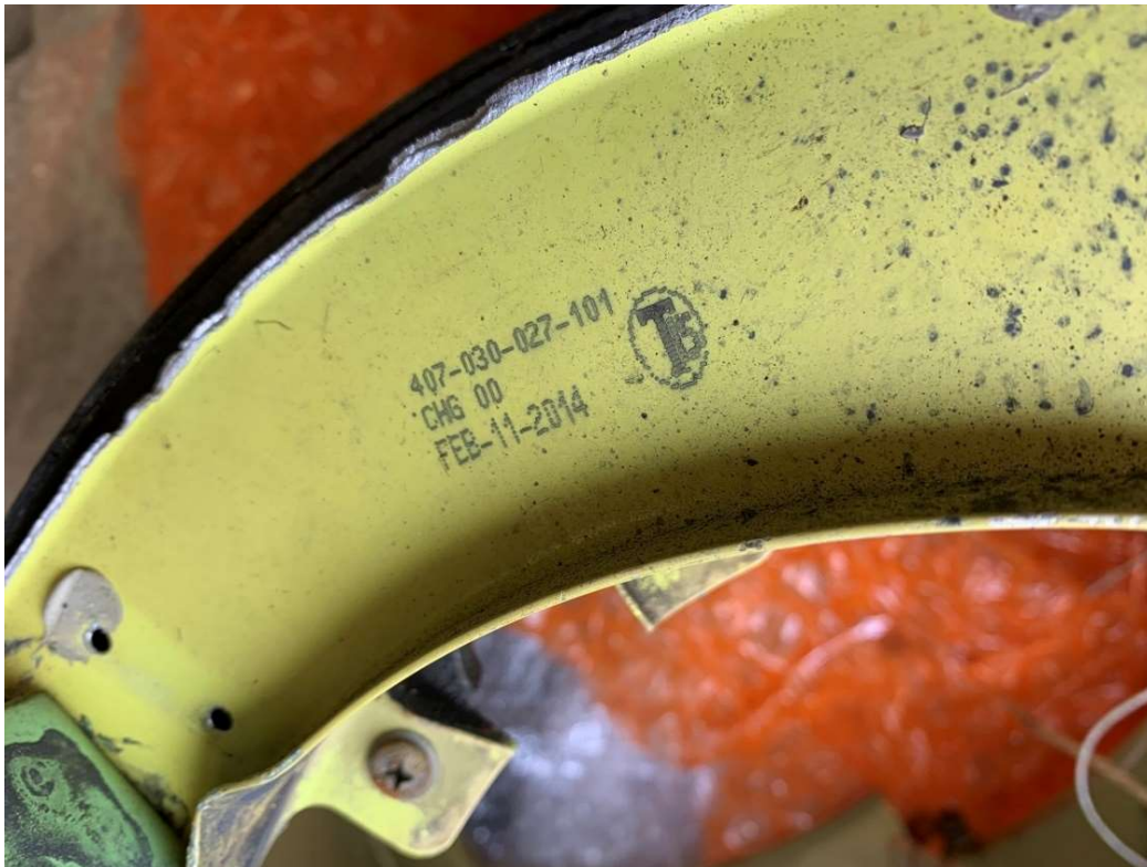
Figure 5. Part markings seen on the aft fuselage bulkhead.
