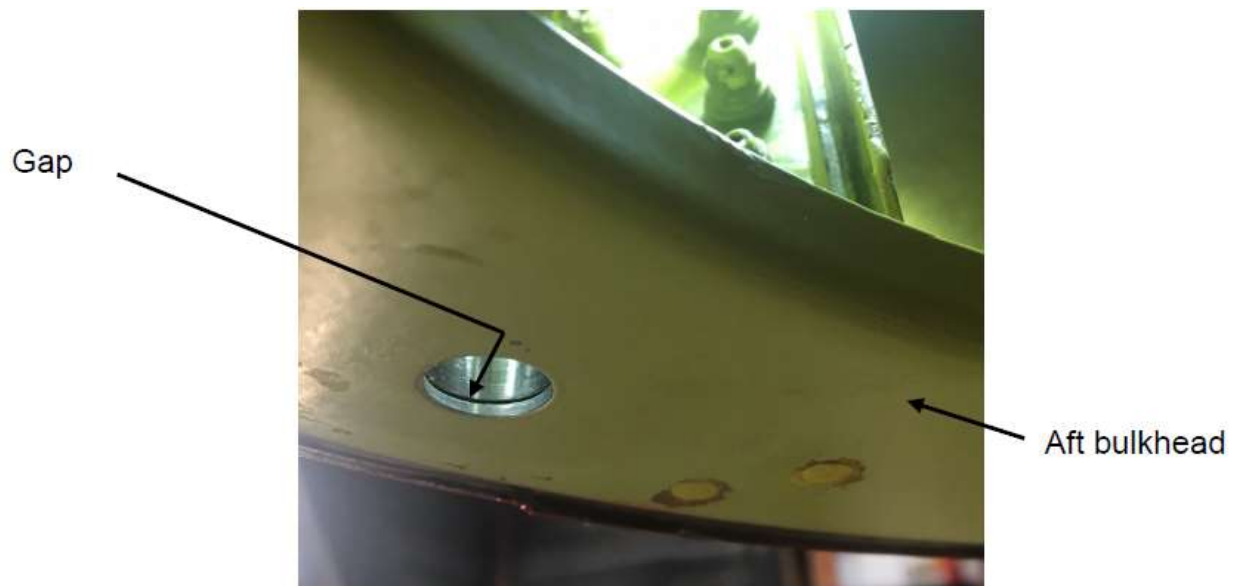
Figure A-2. A gap, measured to be about 0.008 inches, identified between the upper-left longeron and aft fuselage bulkhead. (Image courtesy of Arrow Aviation)
