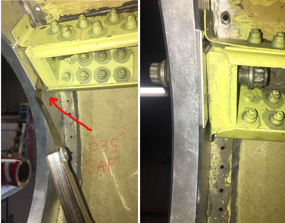
Figure A-3. A gap, measured to be about 0.035 inches, identified between the drill plate and the upper-left longeron attachment fitting. (Image courtesy of Arrow Aviation)
