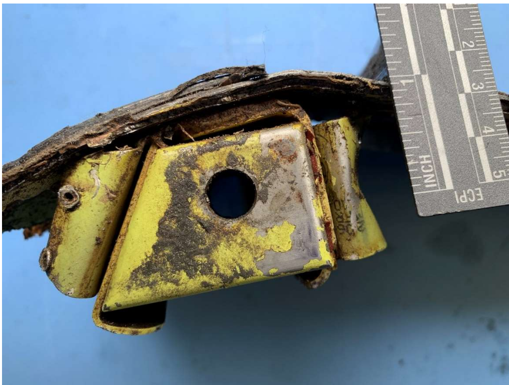
Figure 4. The upper-left longeron fitting's aft face.
