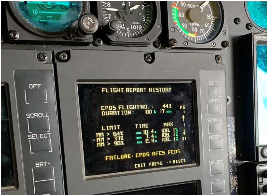
Figure 7. Flight No. 443 mast moment exceedance information on the VEMD.
