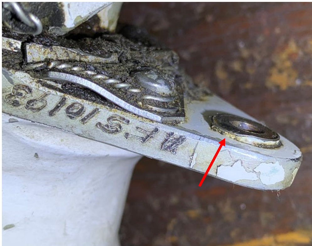
Figure 11. The red arrow points to the visible indentation on the metal boss of the pitch link connection to tail rotor blade S/N ATR72106.
