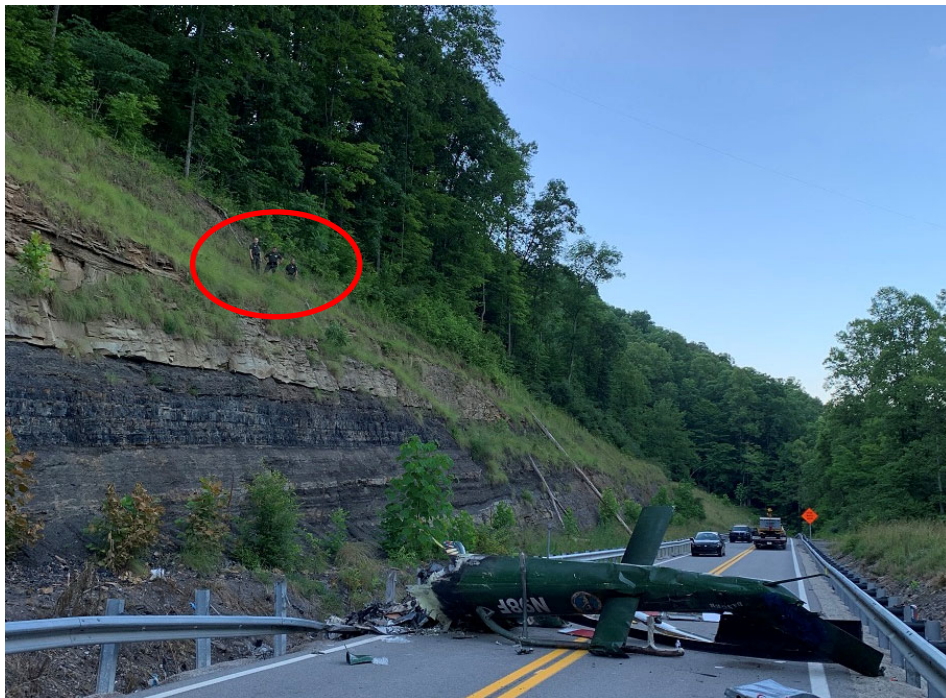
Figure 2. The red circle denotes the area where pieces of Plexiglas, the aft cap of the left skid, a tail rotor blade segment, and a green paint transfer onto a rock.
