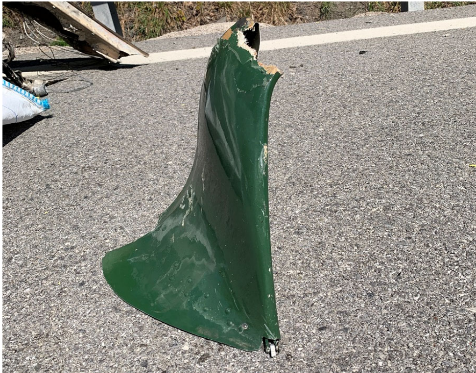
Figure 7. A fractured piece of the main gearbox forward fairing found about 225 feet northeast of the main wreckage.
