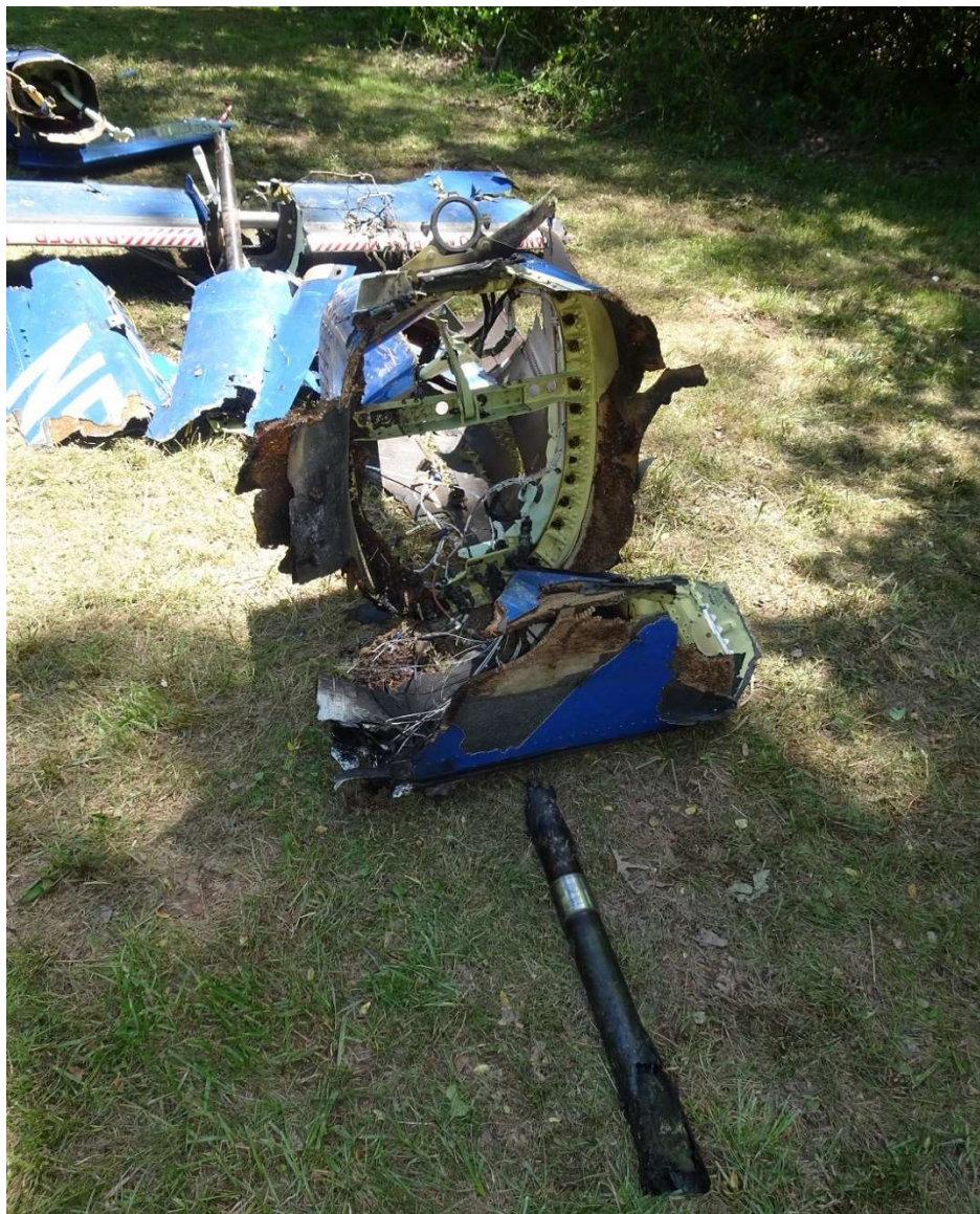
Figure 8. The midsection of the forward segmented drive shaft and the forward snubber installed on a piece of the tail boom.
