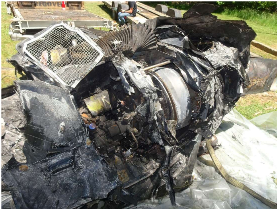
Figure 10. The No. 1 engine on the engine deck after removal from the main wreckage site. The inlet screen and barrier filter were removed by investigators.
