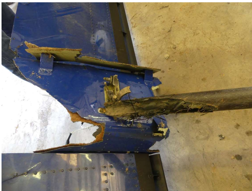
Figure 7. The 34-inch long section of the aft segmented drive shaft, the aft end of which exhibited the angular cut.
