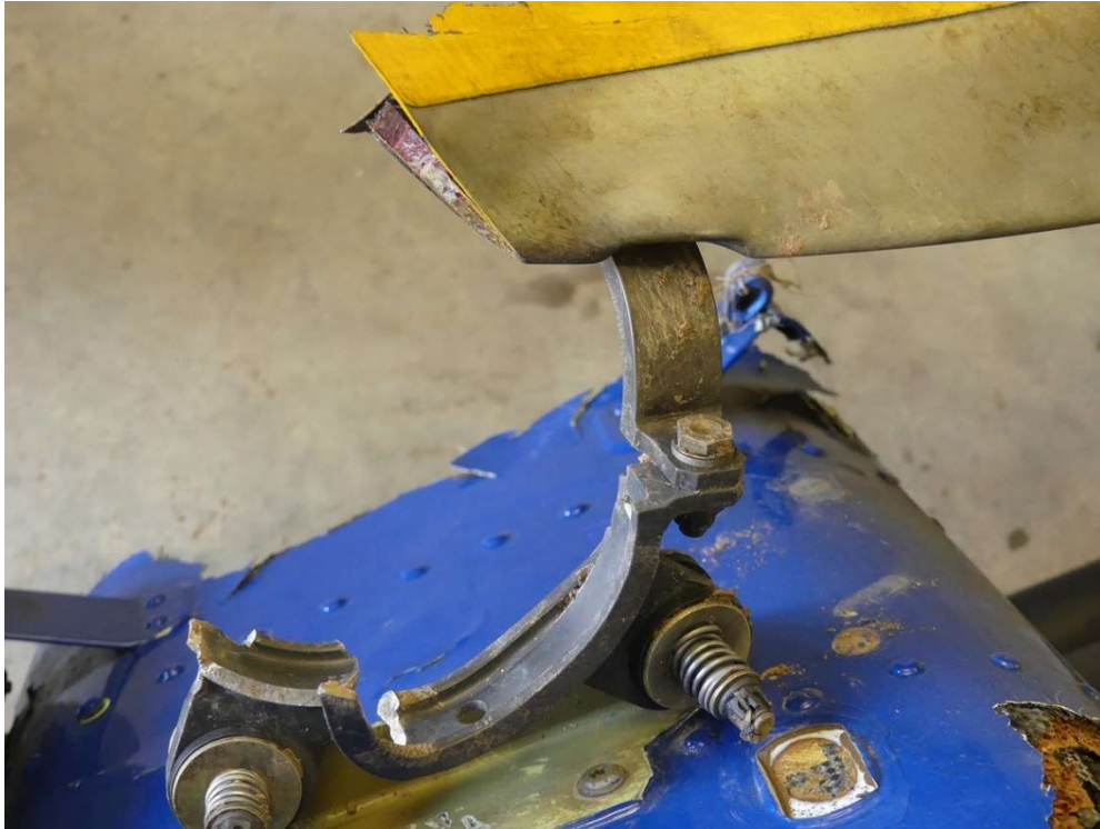
Figure 5. A leading edge impact mark on the tip end of the 'red' main rotor blade matched to the aft snubber. (Image courtesy of Bell.)
