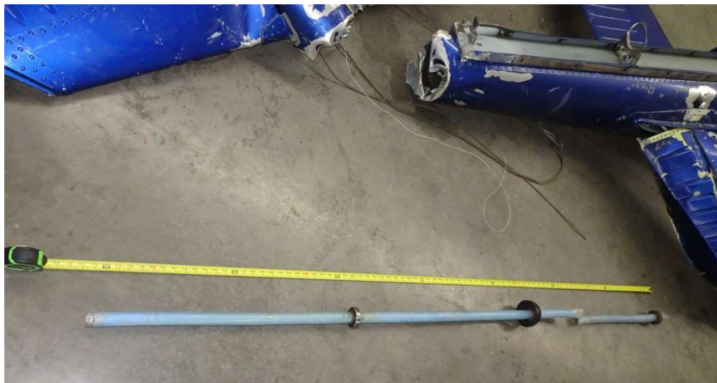
Figure 10. The 62-inch (left) and 22-inch (right) segments of the tail rotor drive shaft.
