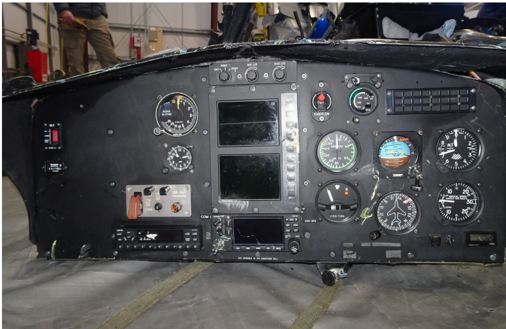
Figure 24. The recovered instrument panel. The VEMD is composed of the two screens at the center of the instrument panel.
