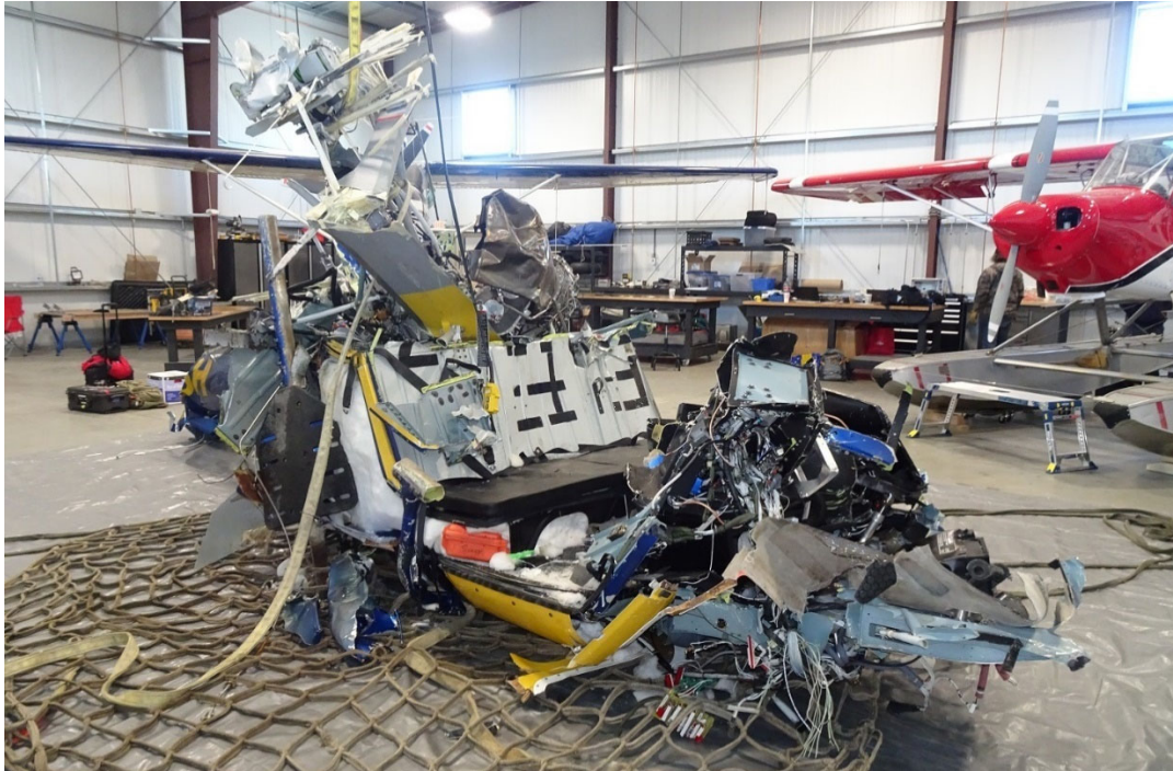
Figure 4. The recovered main fuselage wreckage.
