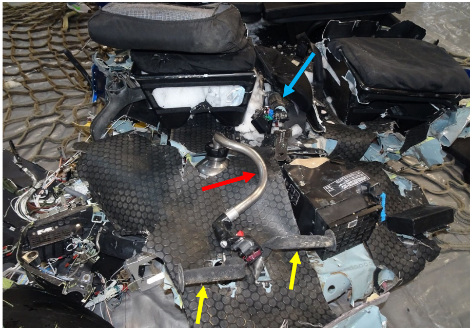
Figure 13. The pilot's cyclic control (red arrow), collective control (blue arrow), and pedals (yellow arrows).
