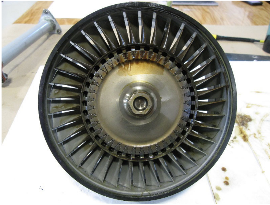
Figure 22. A view of the leading edge of the power turbine blades (after removal from the engine).
