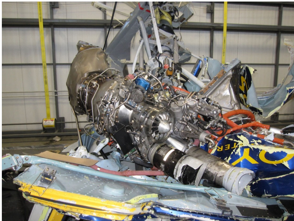
Figure 20. The engine resting on the recovered wreckage.
