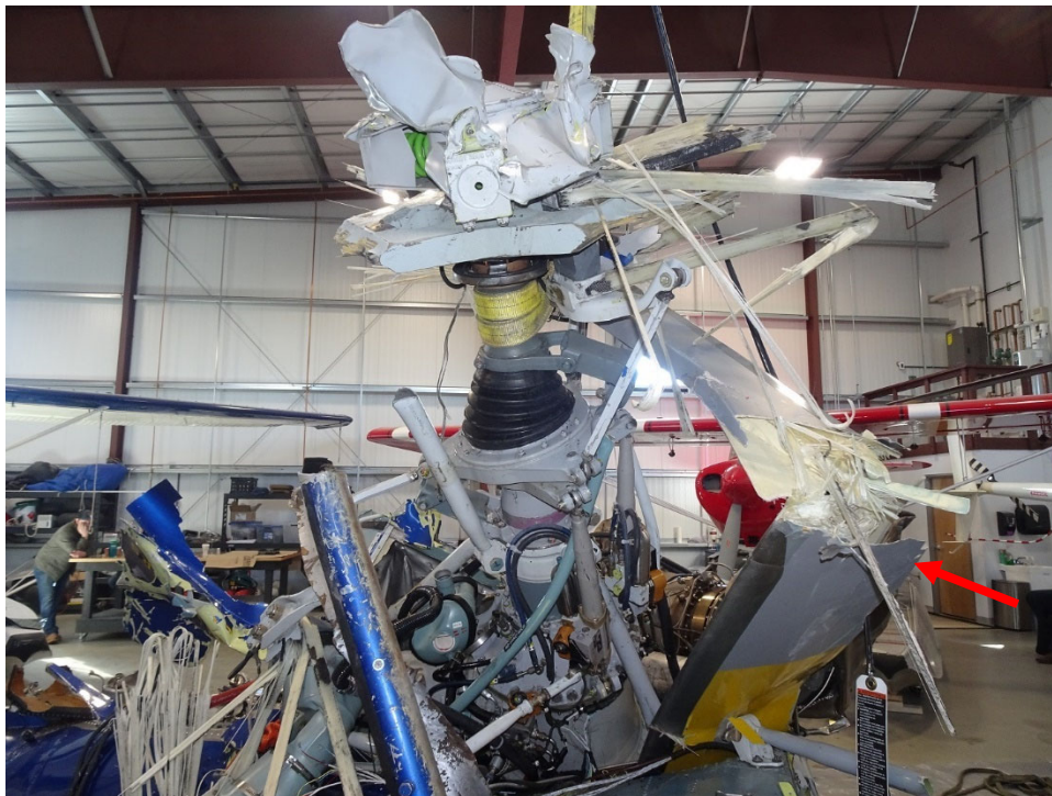
Figure 9. The main rotor head, shaft, and main transmission. The red arrow points to the inboard portion of the ‘red’ main rotor blade.
