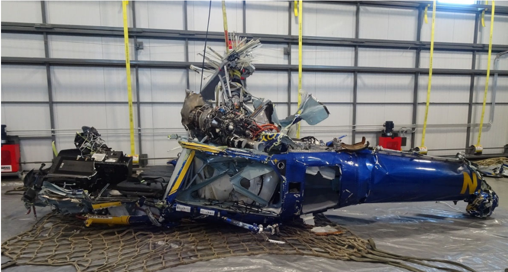
Figure 5. The left side of the main fuselage wreckage.
