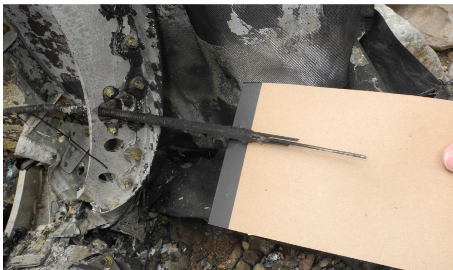
Figure 6. The fenestron control cable near the aft end of the main fuselage.
