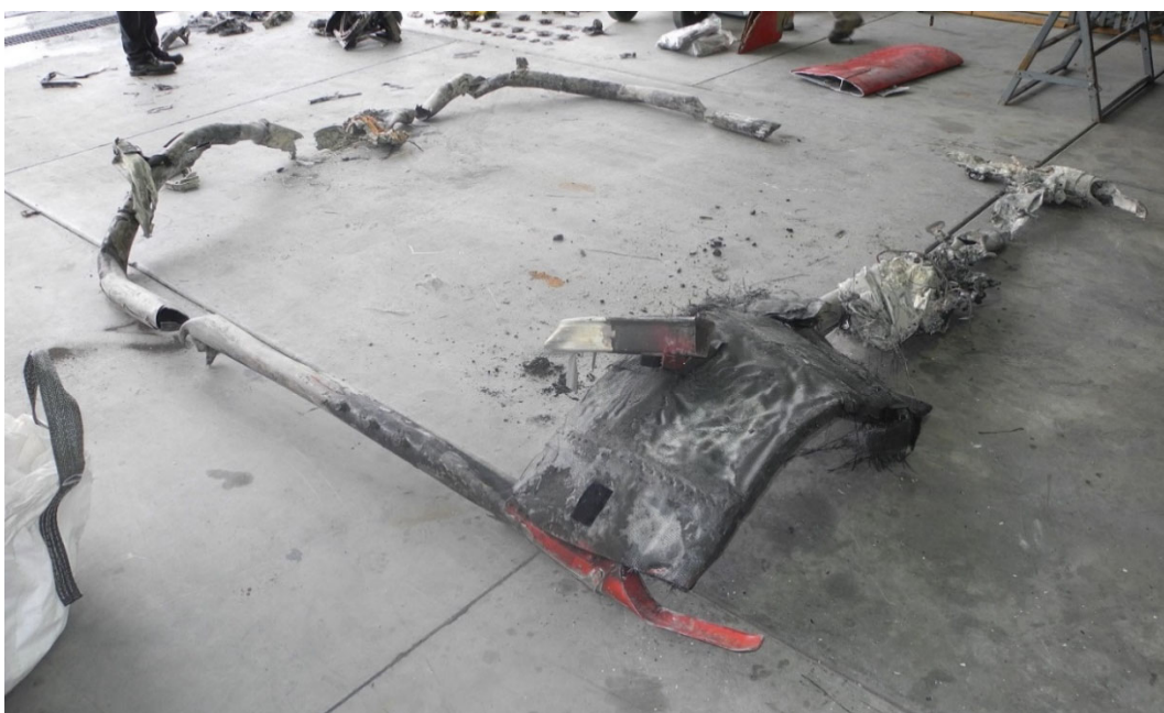
Figure 2. A reconstruction of the landing gear.
