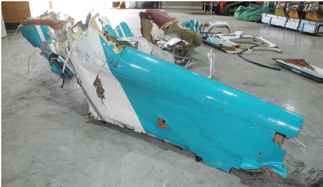
Figure 4. The vertical fin attached to the aft end of the tail boom.
