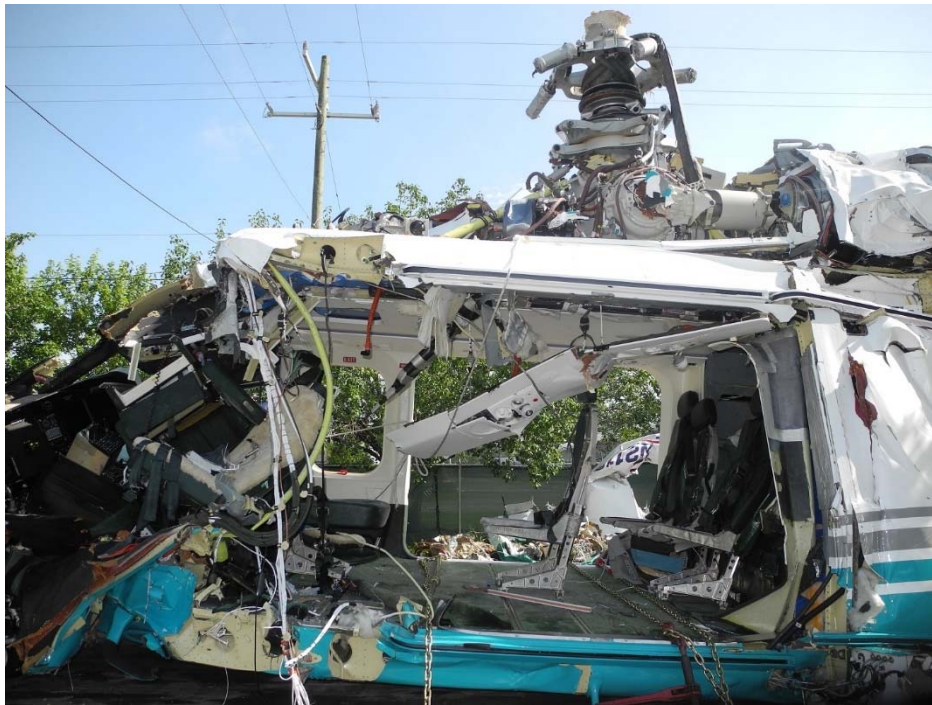
Figure 5. A view of the cabin showing the passenger seats that remained installed.
