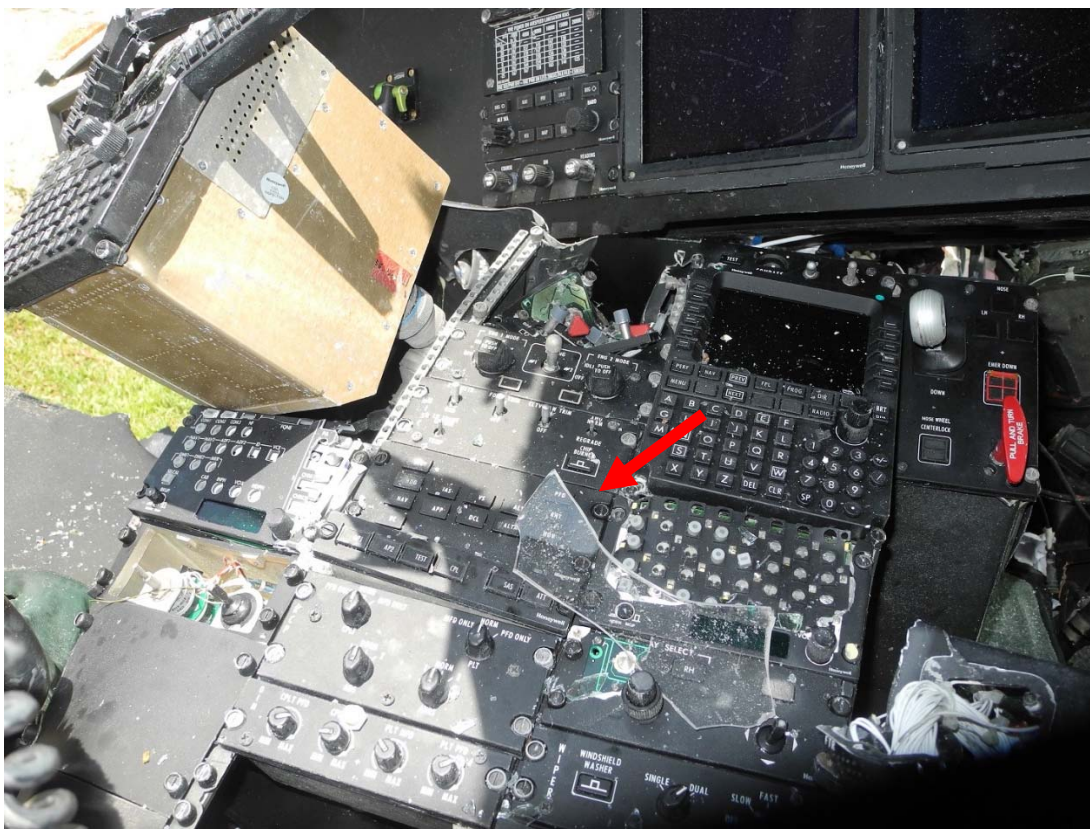
Figure 10. The center console of the cockpit. The red arrow points to the guidance controller and AP control panel.
