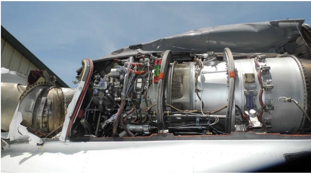
Figure 12. The No. 2 engine installed on the accident helicopter.
