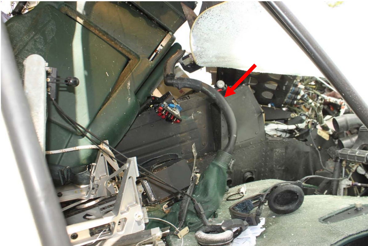
Figure 9. The red arrow points to the right-seat cyclic control. The head of the collective control and a portion of the pedals are also visible.
