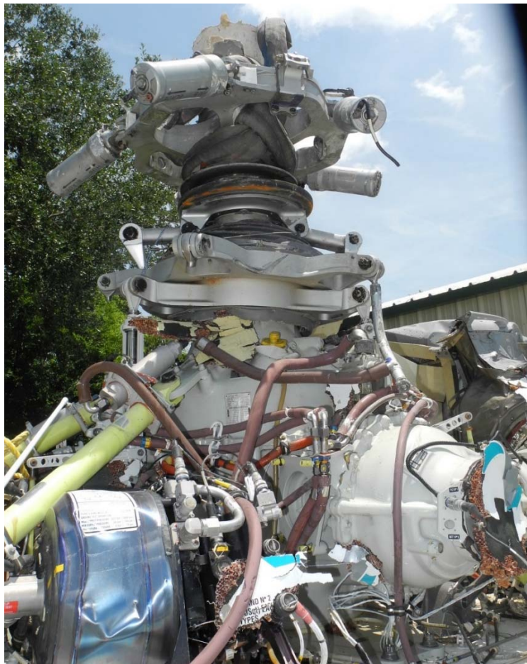
Figure 7. The main gearbox, swashplate assembly, and main rotor hub.
