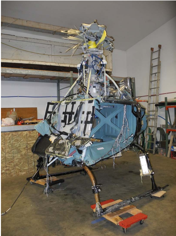
Photo 3. The recovered main fuselage with the main transmission and main rotor head attached. The fuel tank was previously separated for the recovery effort and remained uninstalled.
