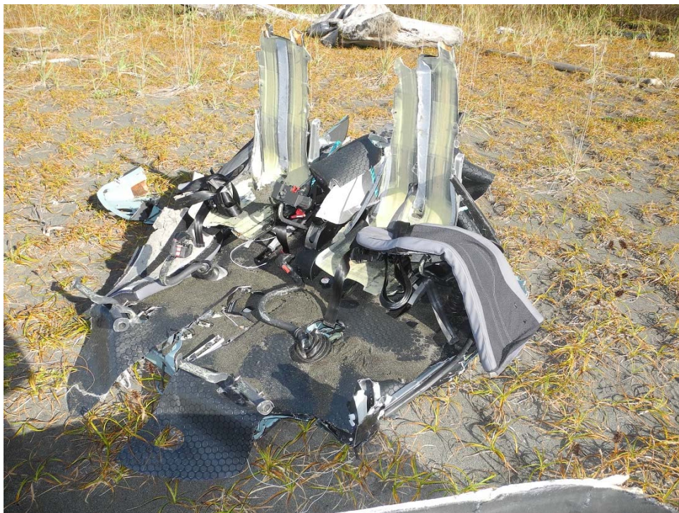
Photo 4. The separated cockpit with front seats still attached.
