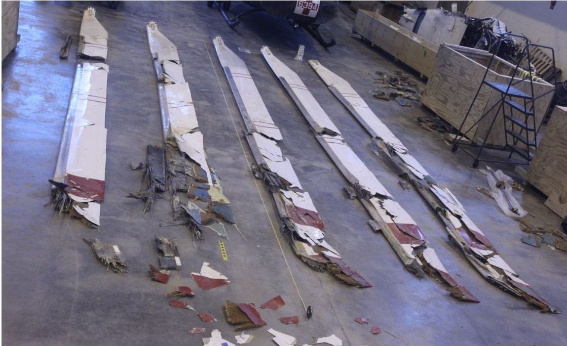
Figure 21. The reconstructed main rotor blades.
