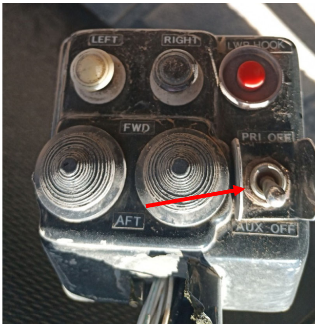
Figure 6. The left pilot's collective-mounted hydraulics switch. (Image courtesy of CHI Aviation)
