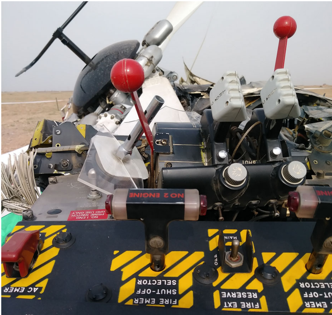
Figure 4. The engine speed selector levers and emergency shut-off T-handles. Note the cockpit roof appears upside-down due to its partial separation during the postcrash rescue of the crewmembers. (Image courtesy of CHI Aviation)
