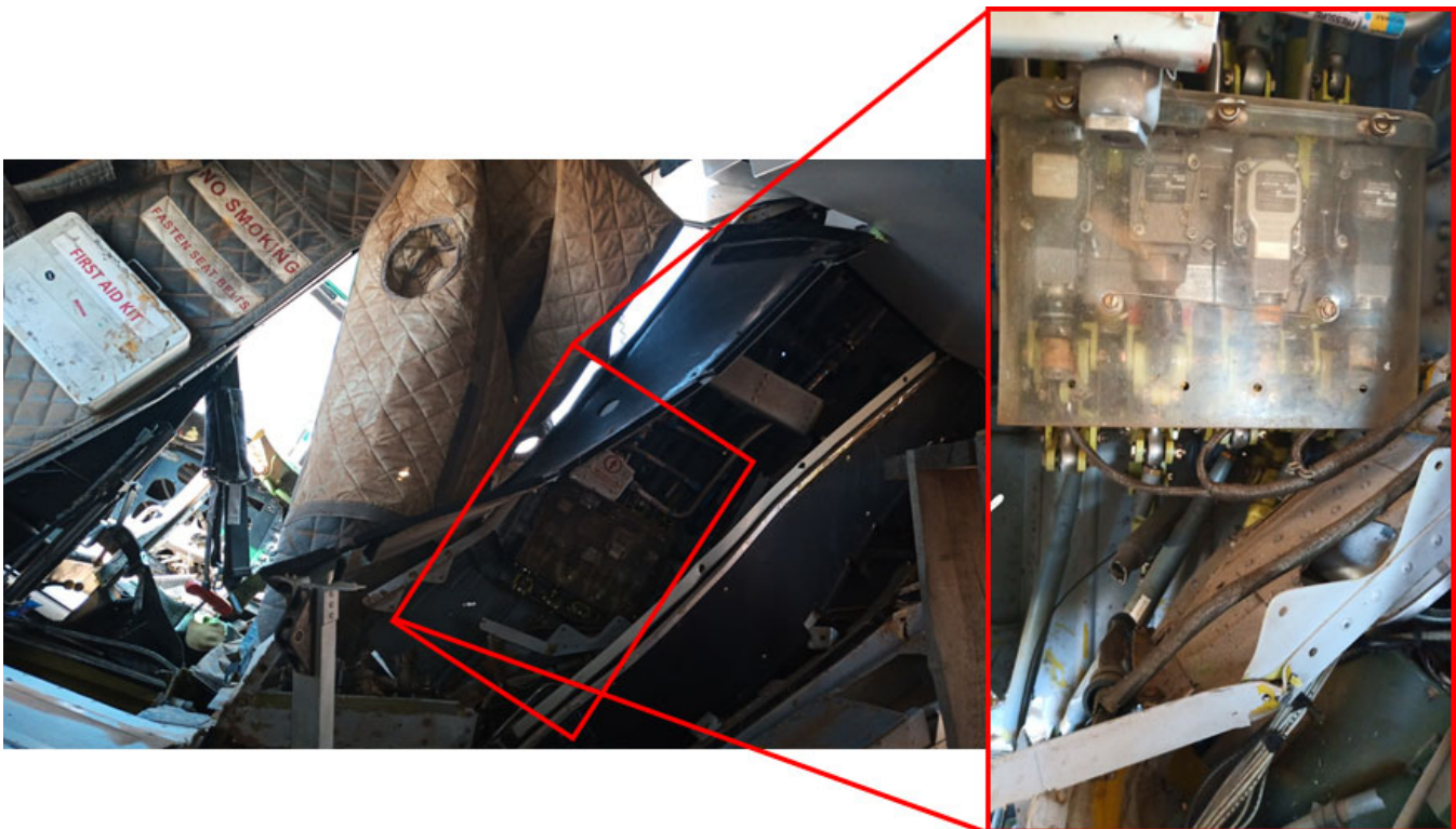
Figure 8. The auxiliary servocylinder installation. (Image courtesy of CHI Aviation)
