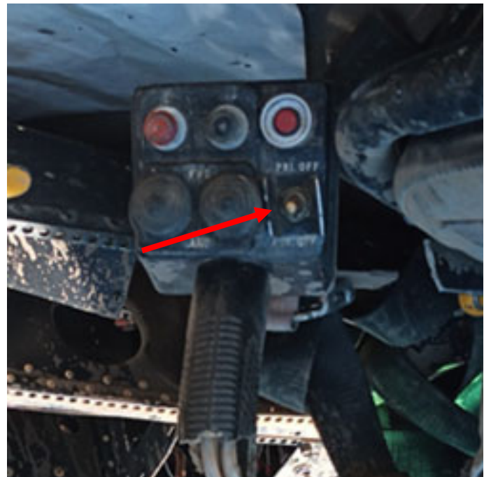
Figure 7. The right pilot's collective-mounted hydraulics switch. (Image courtesy of CHI Aviation)
