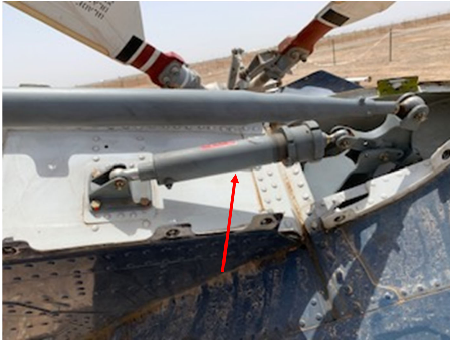
Figure 11. The negative force gradient spring (red arrow) installation on the vertical fin. (Image courtesy of CHI Aviation)
