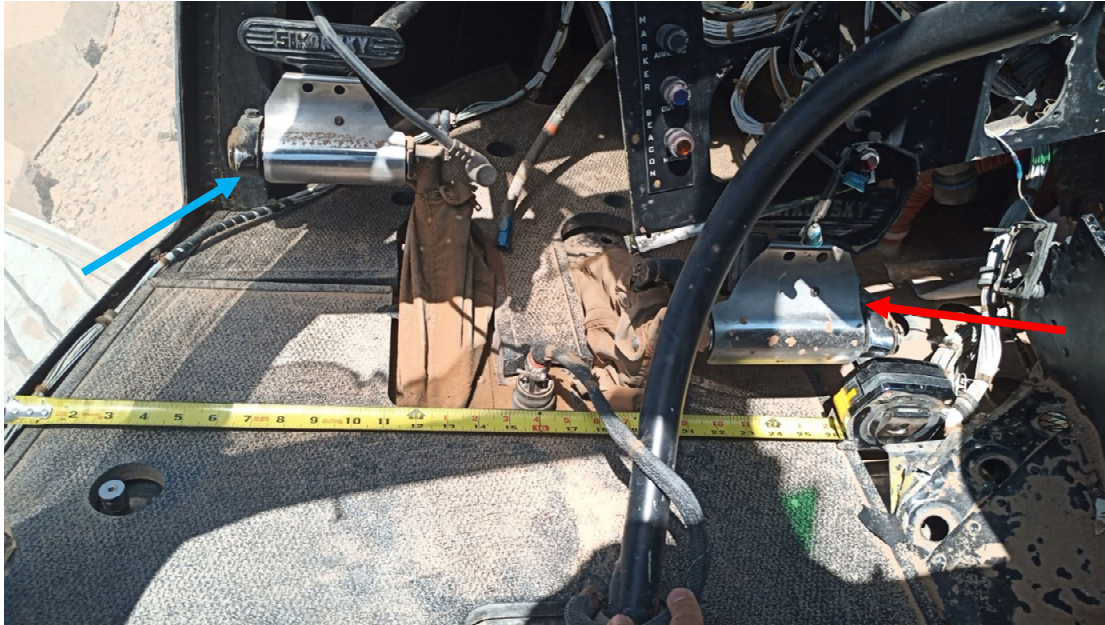
Figure 5. The left pilot's pedals. The left pedal (blue arrow) was displaced forward of neutral while the right pedal (red arrow) was displaced aft of neutral. (Image courtesy of CHI Aviation)
