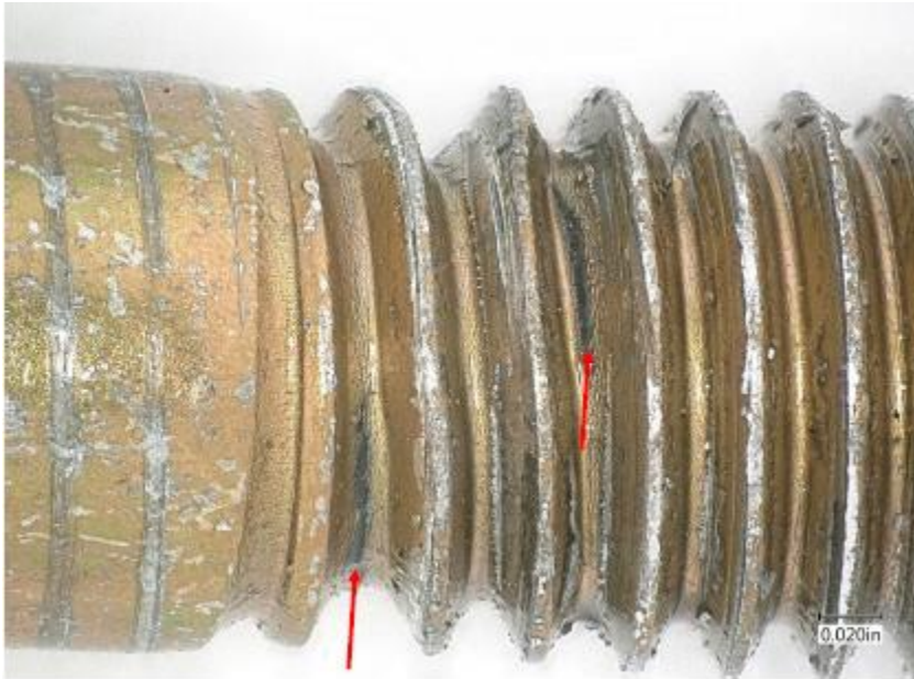
Figure 14 Opposite side of the cracked bolt again showing the cracks in the first engaged thread and an additional crack in the third engaged thread.
