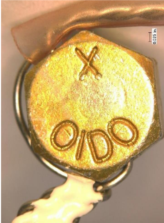
Figure 4 Fractured bolt part markings indicate that the manufacturer was Mac Fasteners. (Cracked bolt had identical markings)
