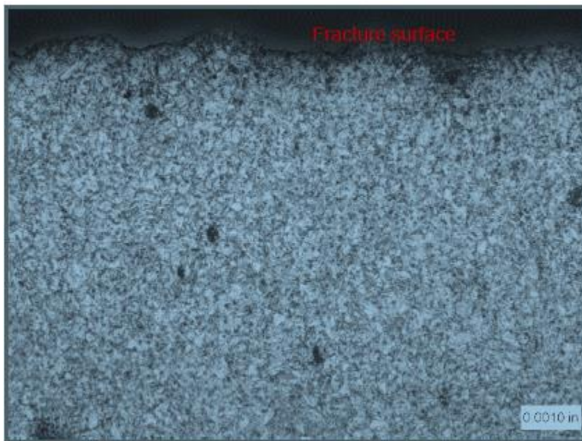
Figure 9 Metallographic cross section of the fractured bolt etched in nital at higher magnification.
