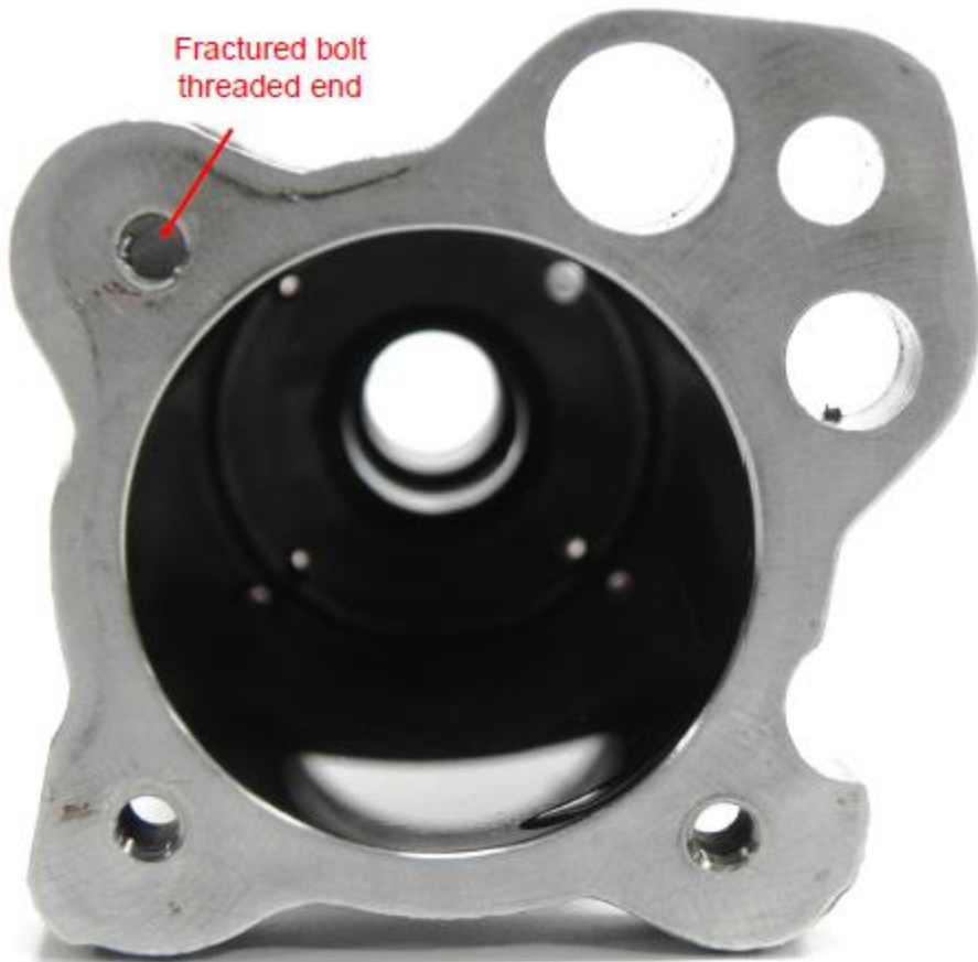
Figure 10 Hydraulic servo cylinder with remaining portion of fractured bolt threads still inside.
