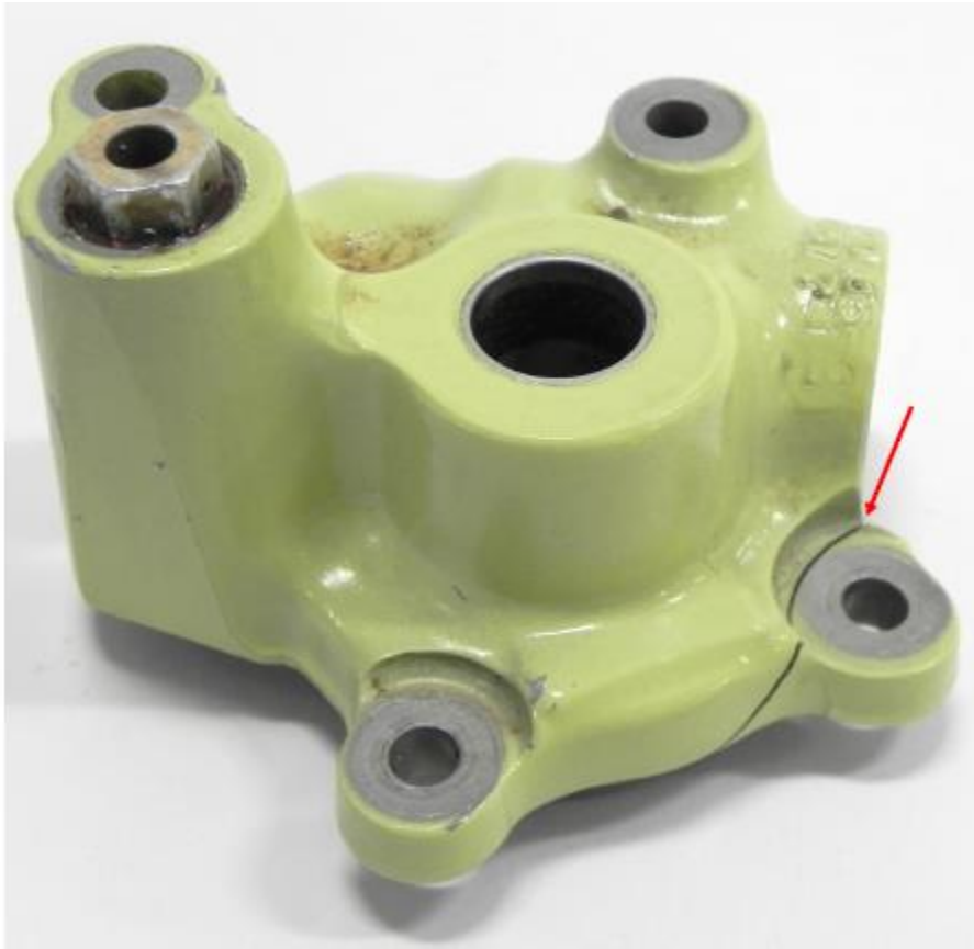
Figure 18 Check valve housing with red arrow indicating fatigue origin.
