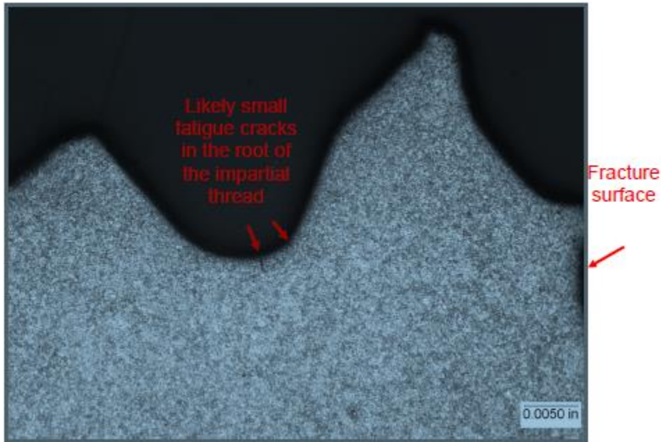
Figure 8 Metallographic cross section of the fractured bolt etched in nital. Likely small fatigue cracks in the root of the impartal thread. Microstructure is typical of martensitic steel. The thread roots do not exhibit elongated grains.
