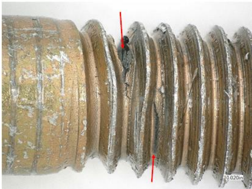
Figure 13 Cracks visible in the first and second engaged threads.
