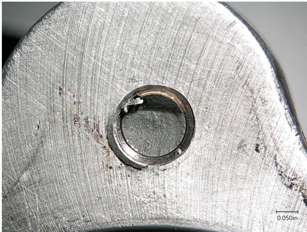
Figure 11 Hydraulic servo cylinder lug with remaining portion of fractured bolt threads still inside.
