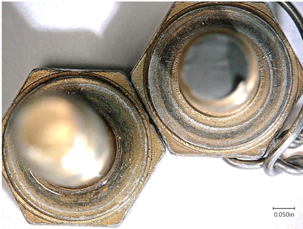
Figure 17 Underside of heads on the cracked bolt(left) and fractured bolt(right).
