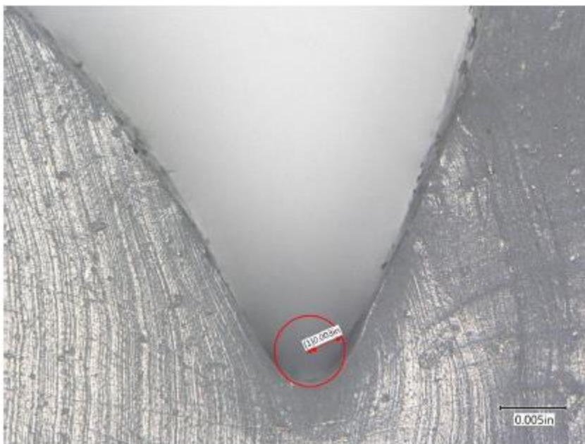
Figure 23 Replica cross section near housing origin. Radius measures about .003".
