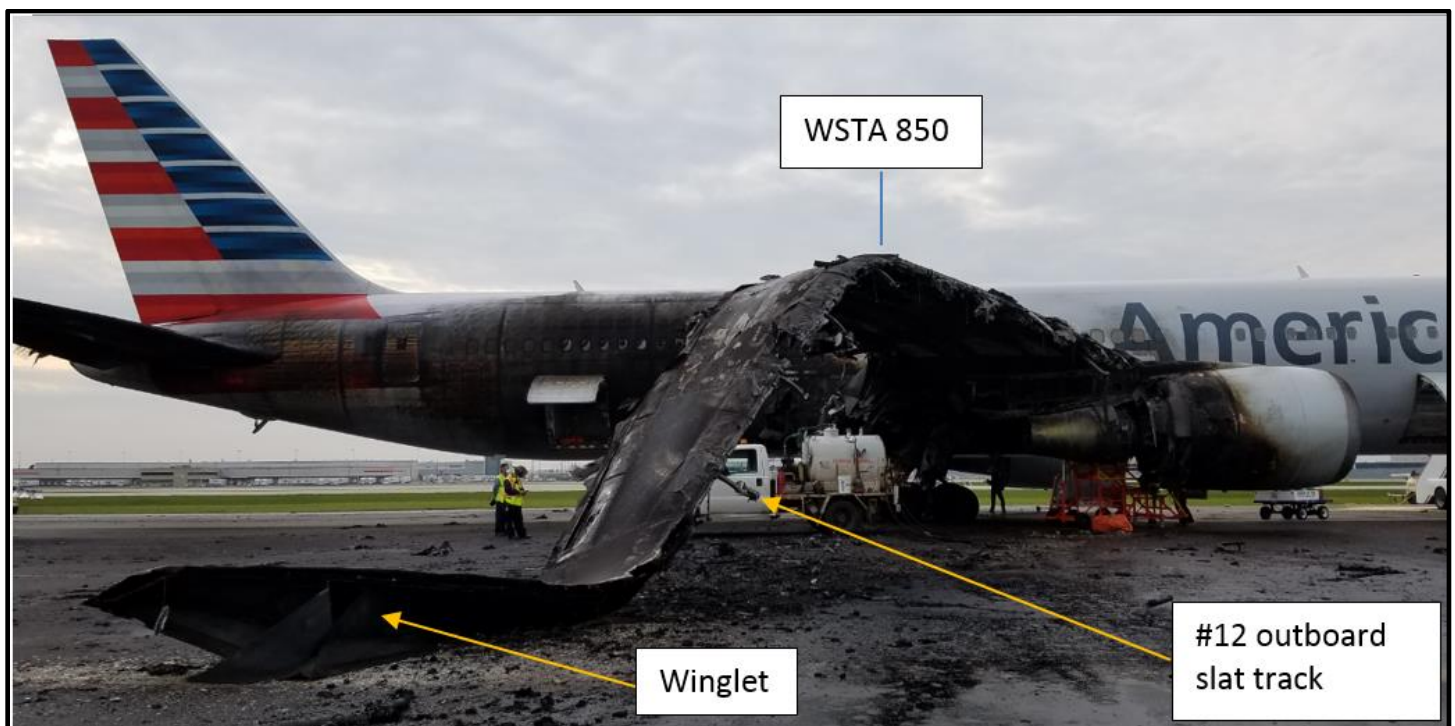
Figure 46 View looking inboard at right wing bent down and contacting the tarmac
