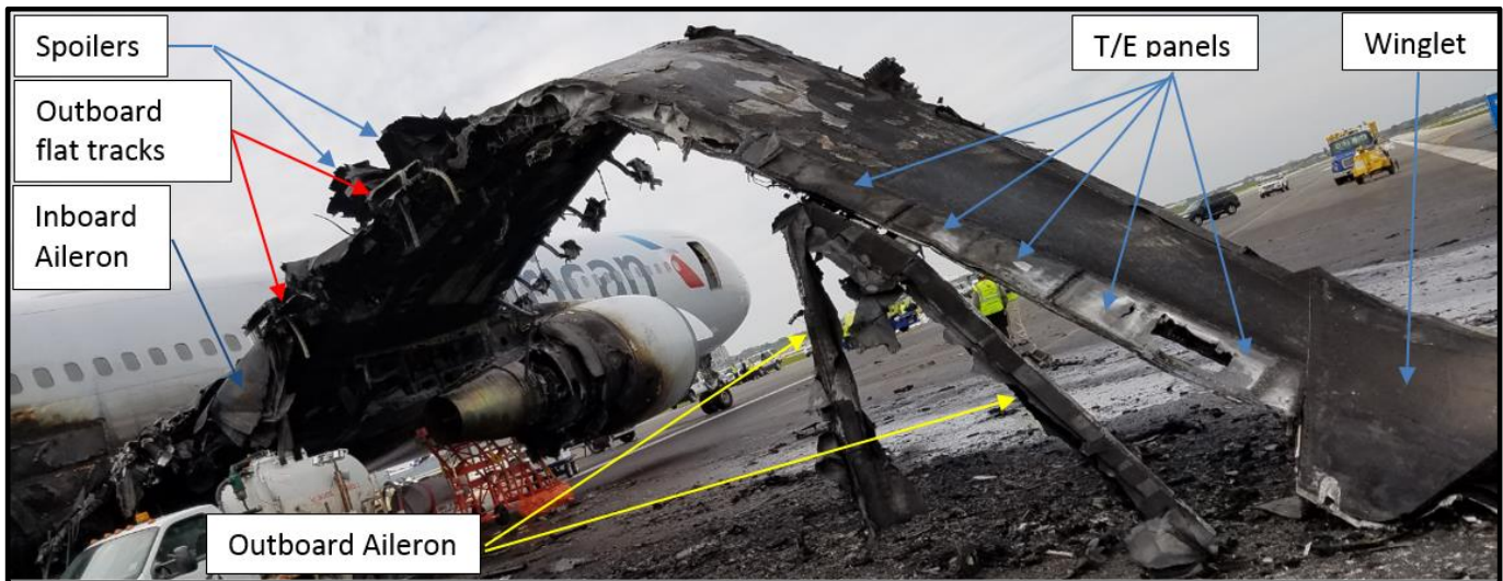
Figure 49 View of right wing looking forward and inboard at outboard bend section
