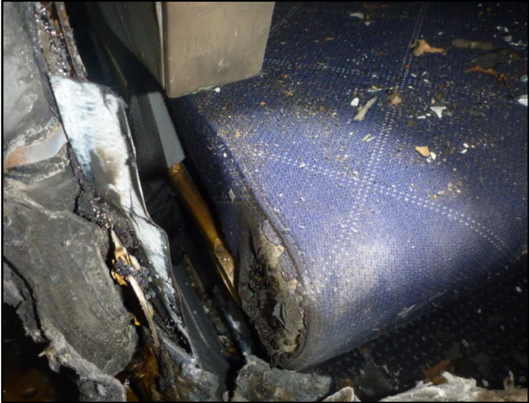
Figure 57 Seat 34 charred seat cushion
