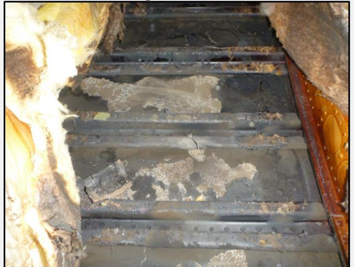
Cracked stringer 25R at STA 1197+120
