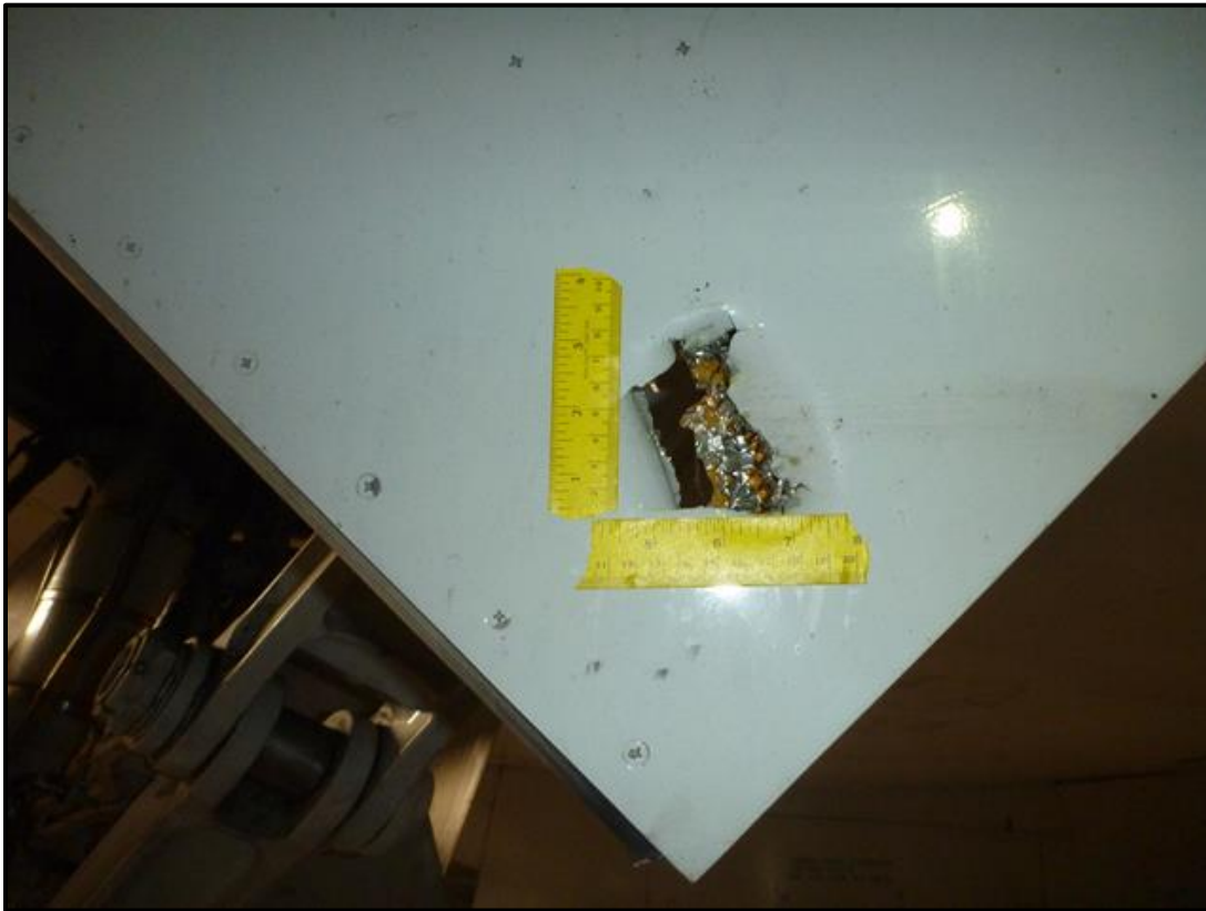
Figure 38 Impact L, left main gear drag strut door
