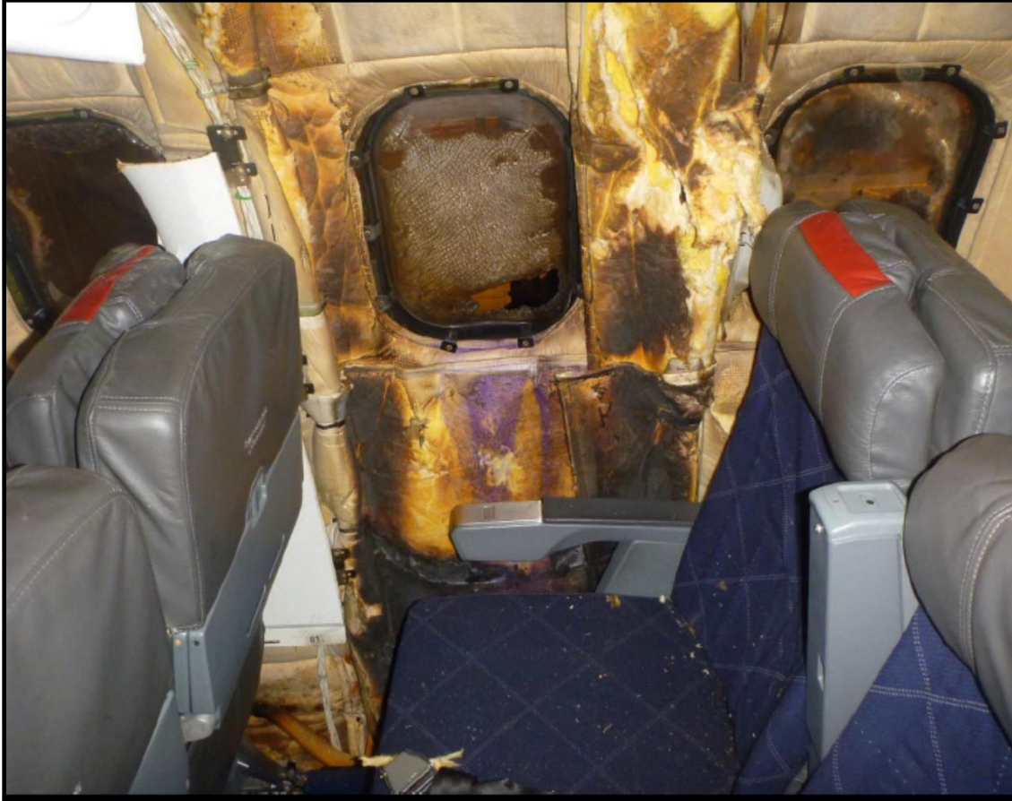
Figure 59 Charred insulation blankets and melted window at seat 30
