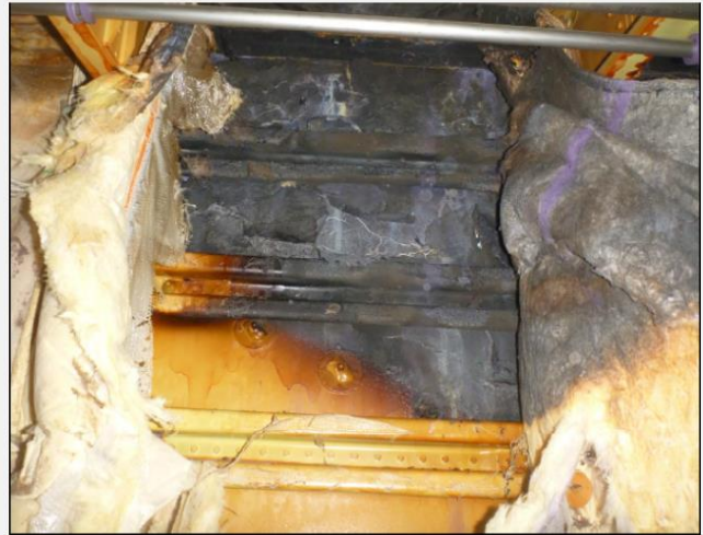
STA 1197+22 to 1197+44 (note hole/cracks)
