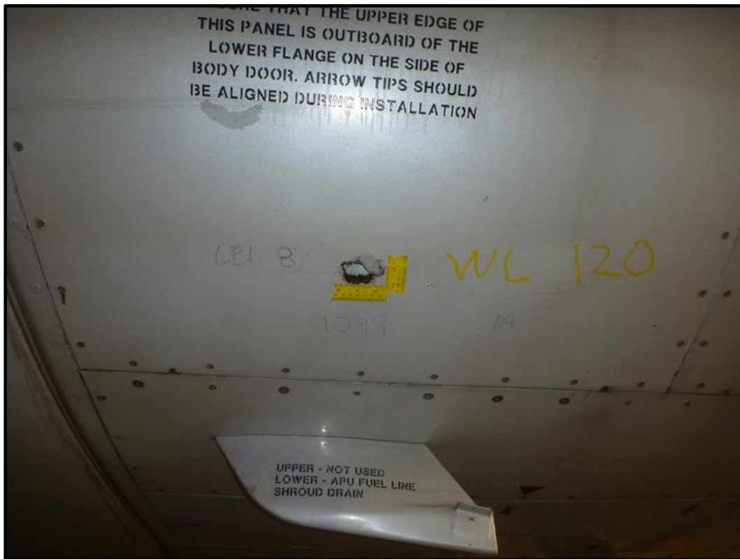
Figure 36 Impact K, Left side of body door
