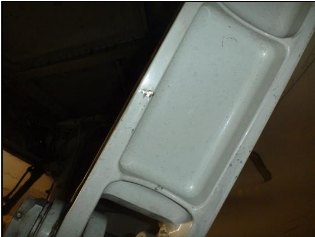
Figure 39 Impact M, left main gear drag strut link
