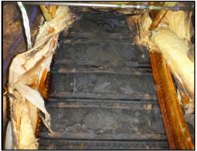
Cracked stringer 25R at STA 1197+120
