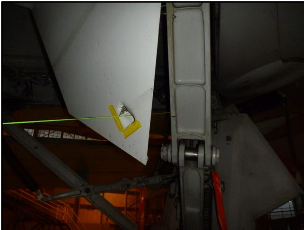
Figure 37 Impact L, Left main gear drag strut door
