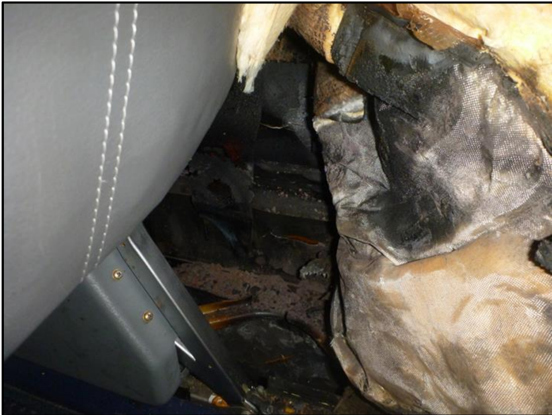
Figure 62 Charred insulation and crack in skin at seat 31
