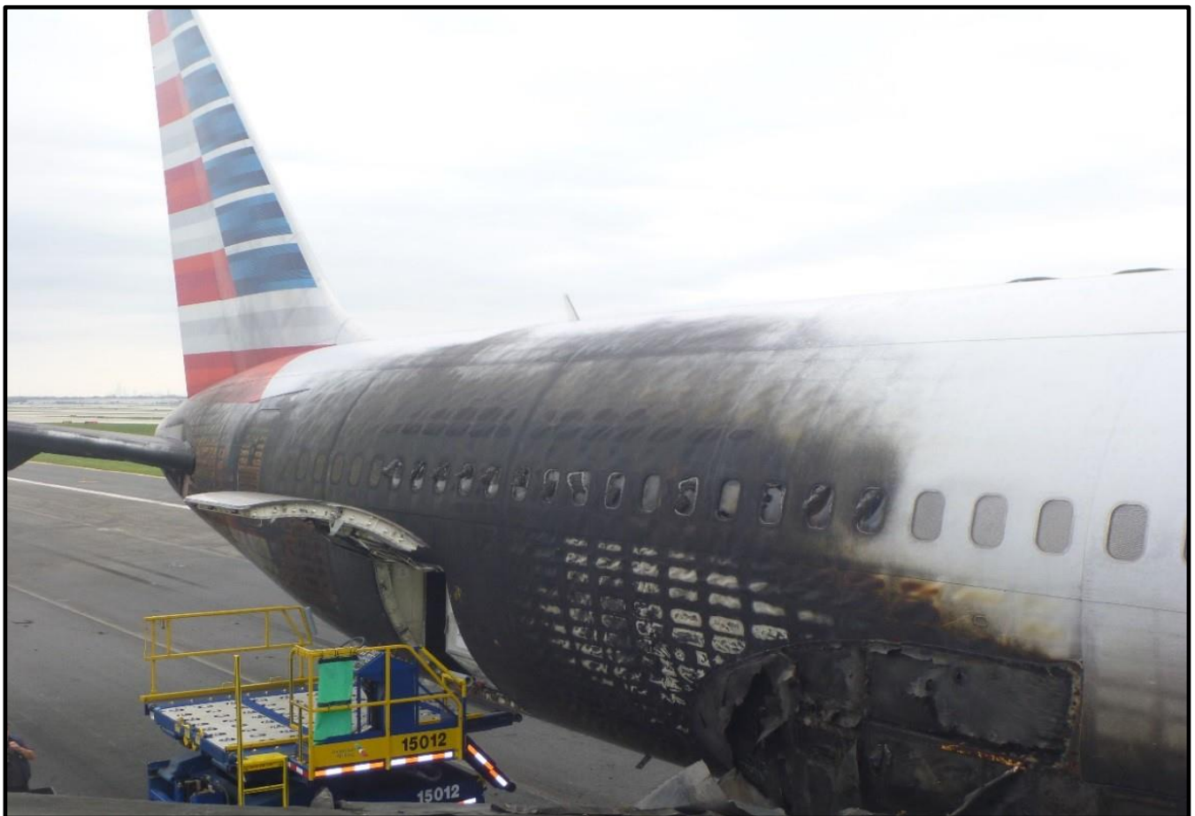
Figure 43 Thermal damage to the right side of the fuselage
