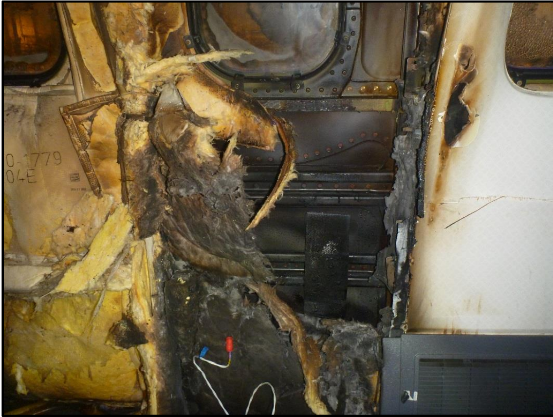
Figure 62 Charred insulation and crack in skin at seat 31
