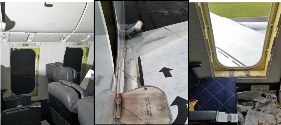
Figure 71 Doors 2L/3L Over Wing Exits (OWE) open
