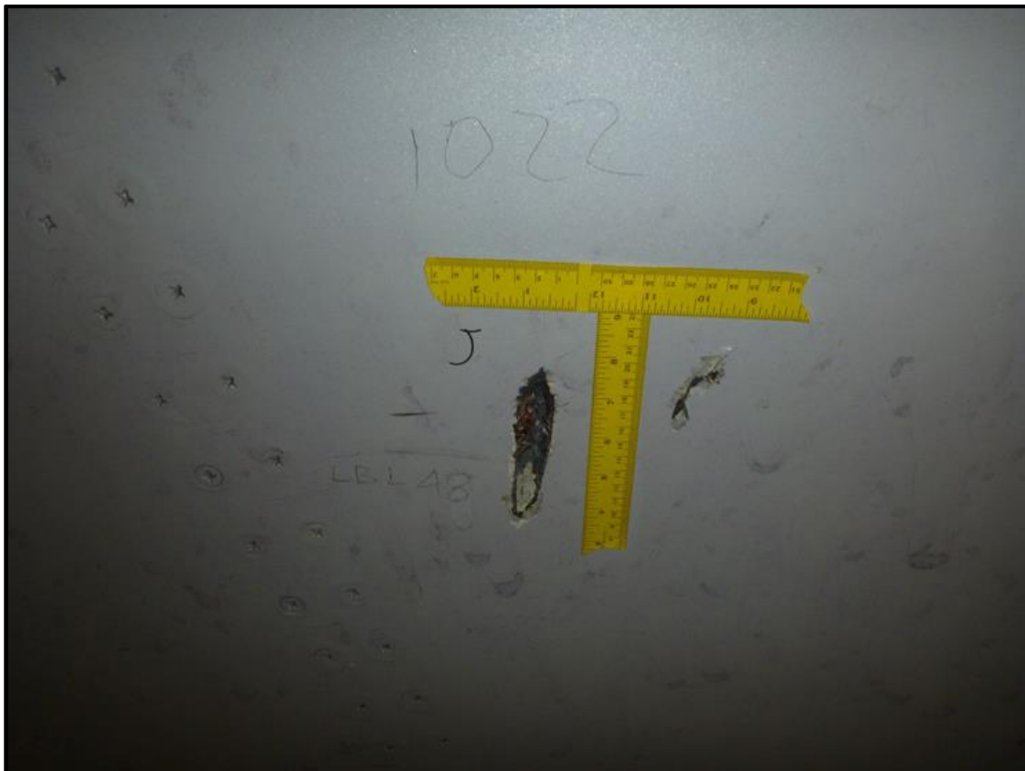
Figure 35 Impact J, Main gear door left side
