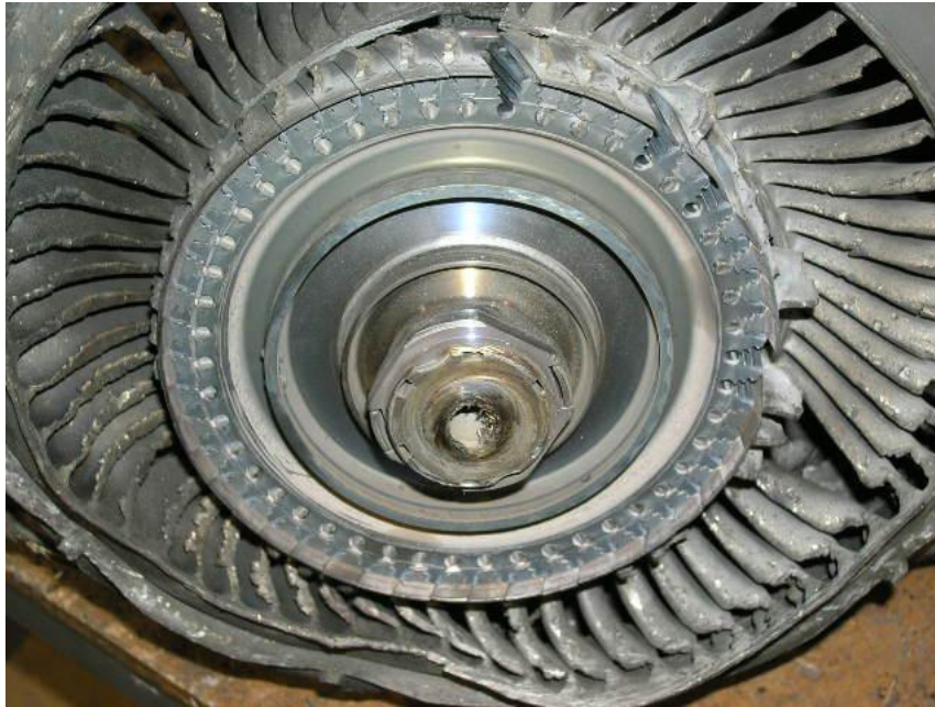
Figure 30 - Photo of First Stage Power Turbine
