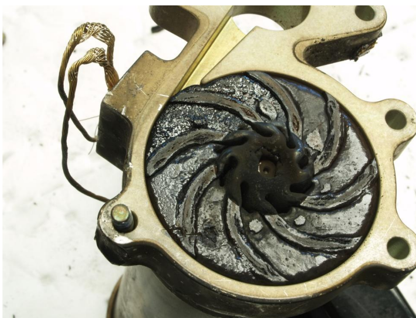
Figure 20 - Melted Right Fuel Boost Pump Impeller
