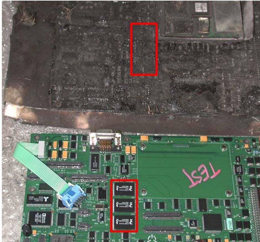
Figure 10 - Exemplar PCB and memory chips (below) and accident PCB with missing memory chips (above)
