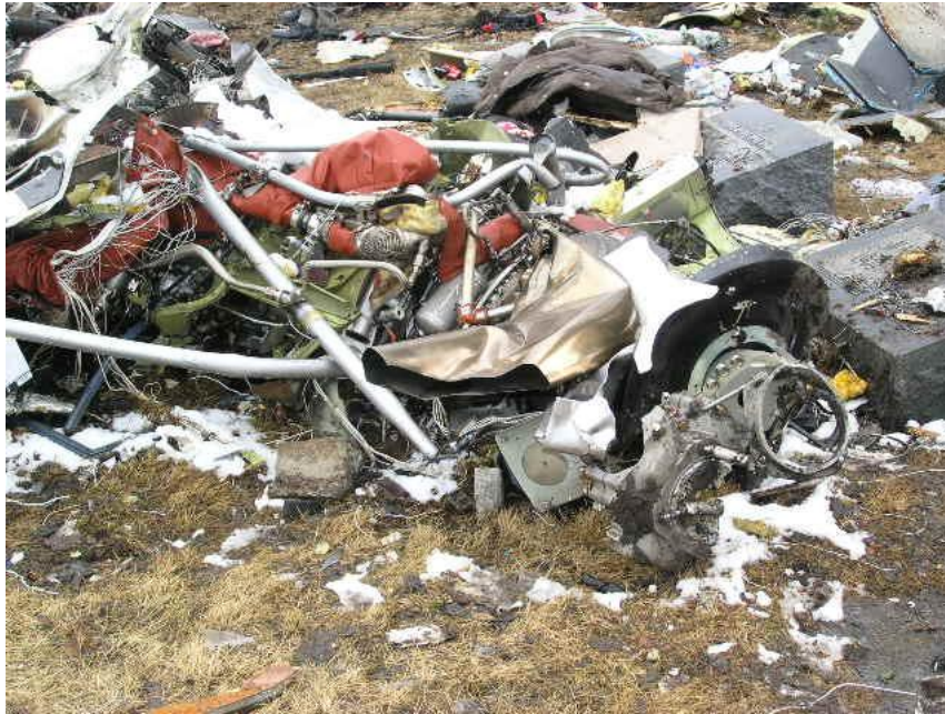
Figure 25 - Photo of Engine and Nacelle, Right Hand Forward View
