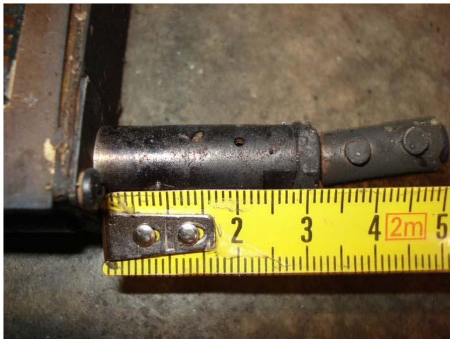
Figure 7 - Photo Visible Extension of the Aileron Trim Actuator
