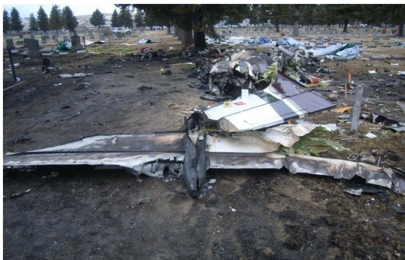
Figure 6 - Photo of Horizontal and Vertical Stabilizers (from rear)
