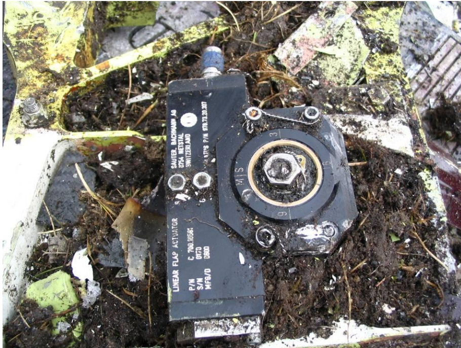
Figure 8 - Photo Showing One of Four Fully Retracted Flap Actuators (left inboard shown)
