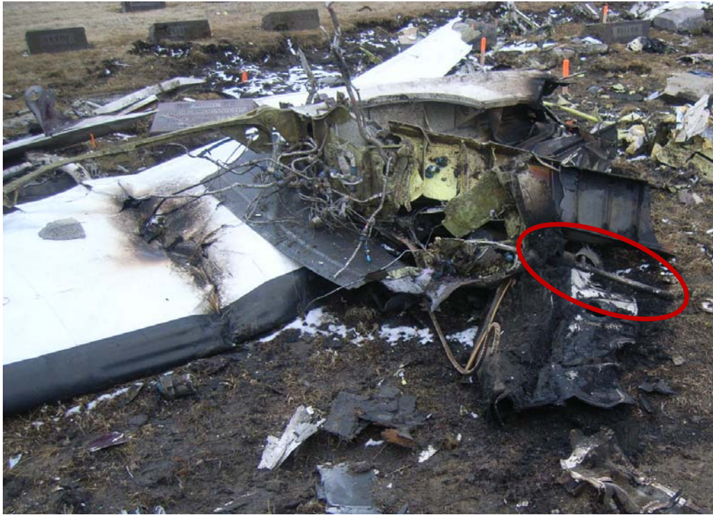
Figure 1 – Photo of right main landing gear actuator (extended)
