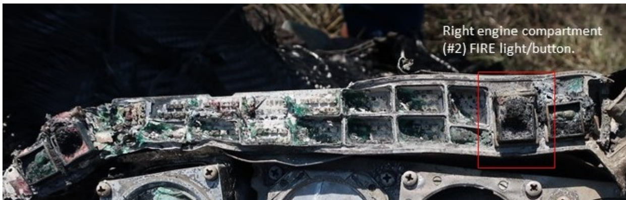
Photo 12- Cockpit warning panel, #2 fire light identified.
