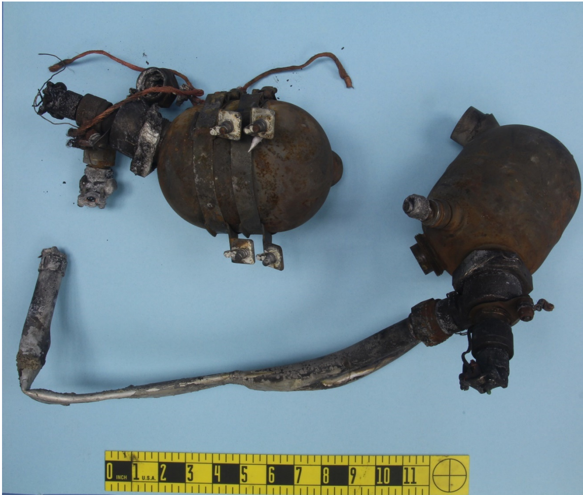
Photo 11 - Fire Suppressant Bottles.
