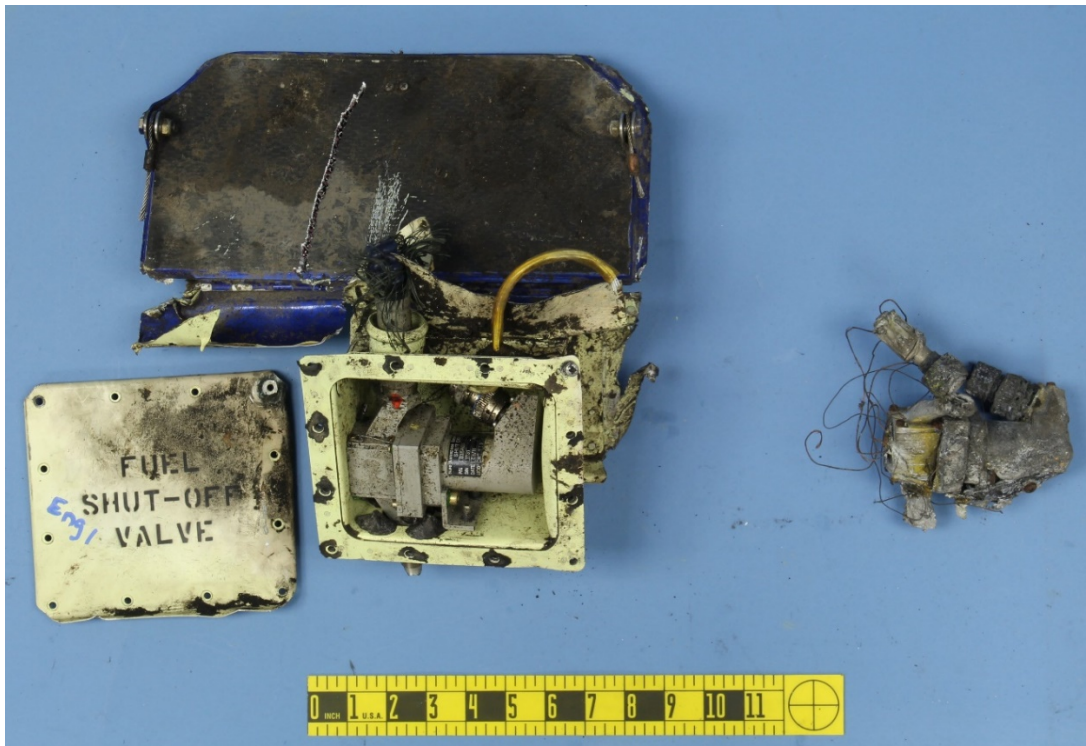
Photo 9 - Fuel Shutoff Valves
