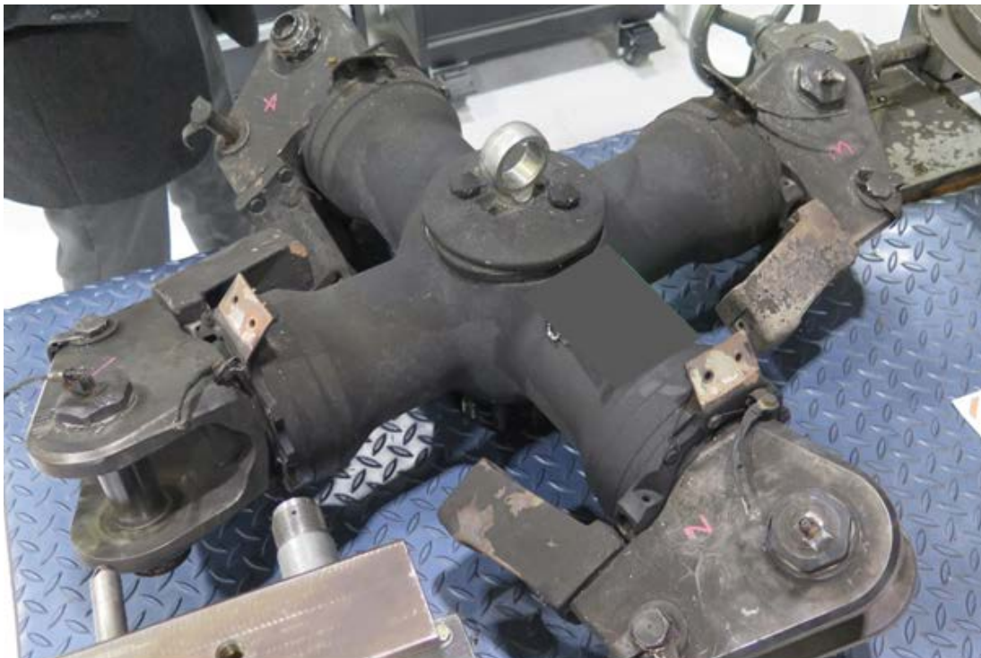
Photo 6 - Rotor head removed from rotor mast for examination 4 .
