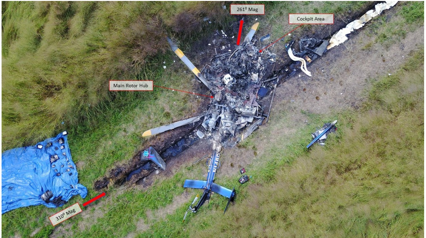
Photo 3 - Wreckage overhead view.
