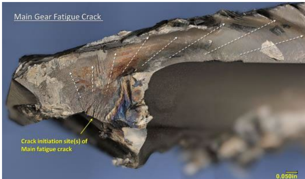
PHOTO 34: MAIN FRACTURE IN THE ZEROL GEAR
