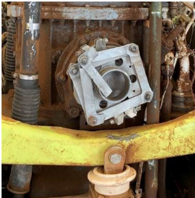
PHOTO 16: END FITTING AND FLEX FRAMES ATTACHED TO THE HELICOPTER MAIN TRANSMISSION GEARBOX
