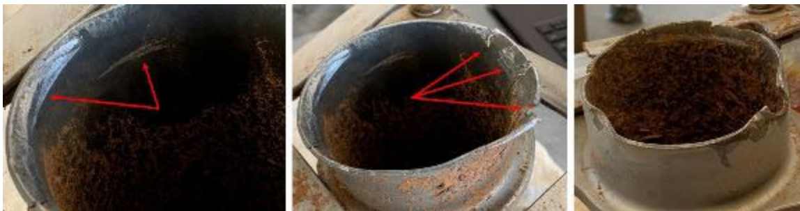
PHOTO 19: INTERCONNECT SHAFT DEFORMATION
