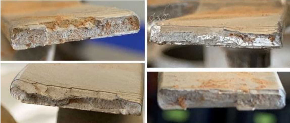
PHOTO 17: BROKEN FLEX FRAMES AT THE HELICOPTER MAIN TRANSMISSION GEARBOX END FITTING
