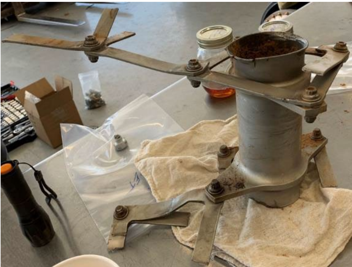
PHOTO 18: INTERCONNECT SHAFT WITH FLEX FRAMES STILL ATTACHED
