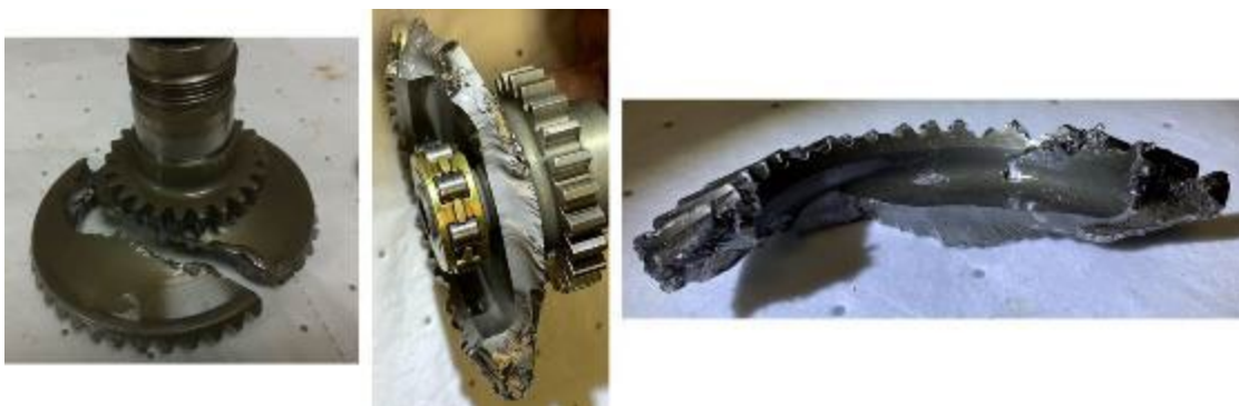
PHOTO 26: FRACTURED ZEROL GEAR (STARTER/GENERATOR GEAR ASSEMBLY)
