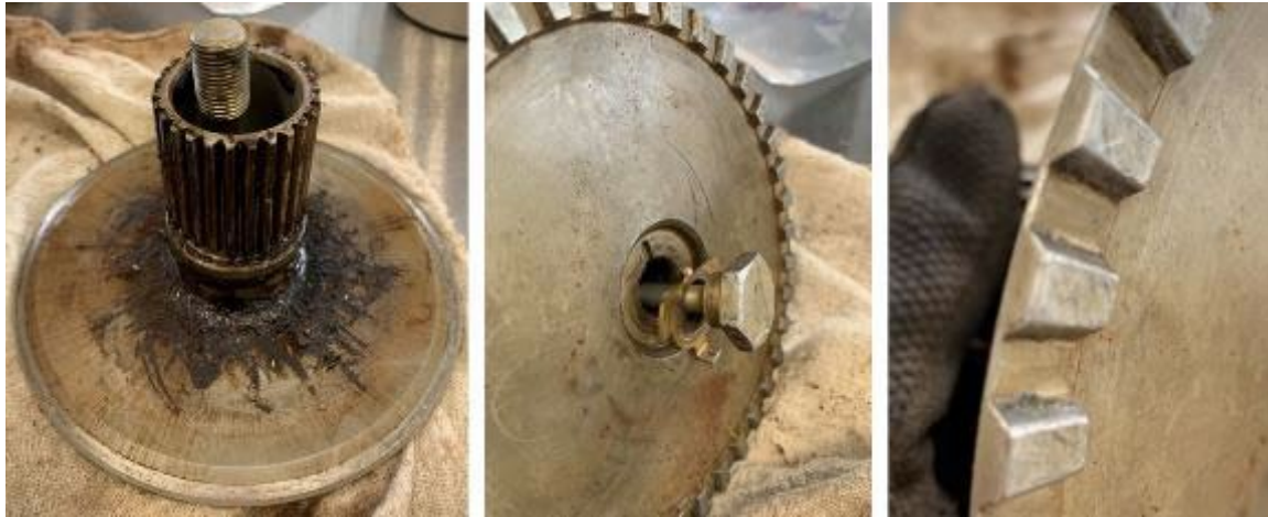
PHOTO 15: ENGINE-KAFLEX COUPLING ADAPTER PLATE
