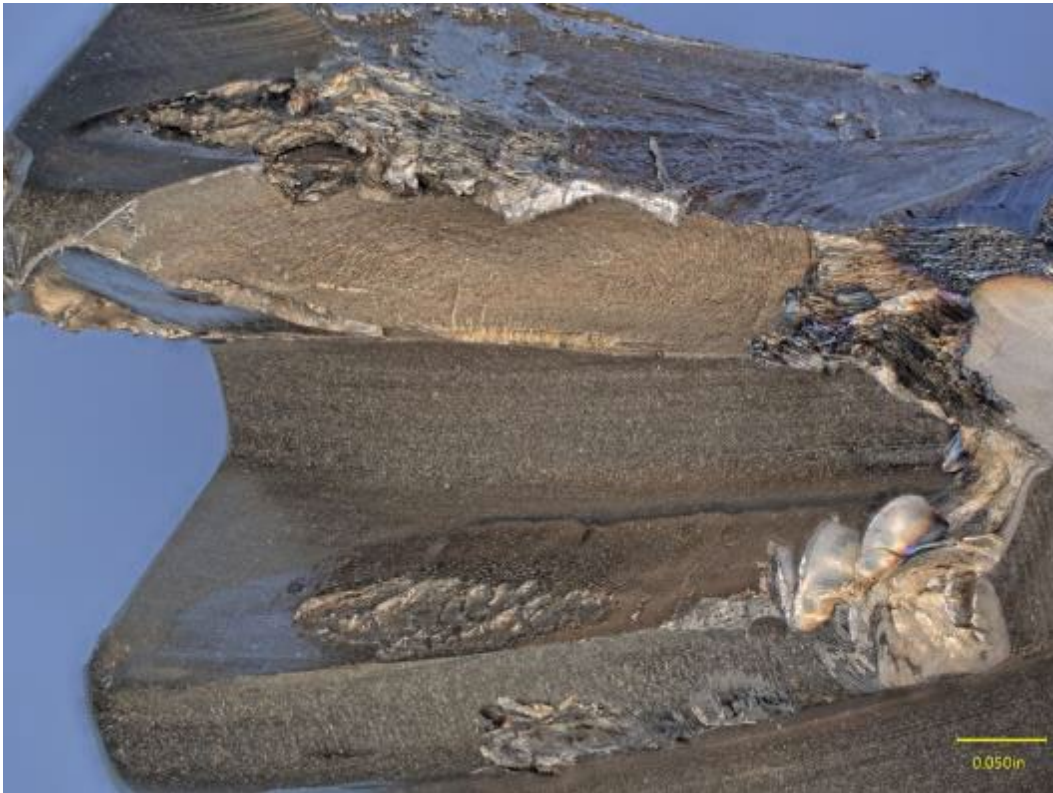
PHOTO 36: EXAMPLE OF ADDITIONAL FATIGUE CRACKING
