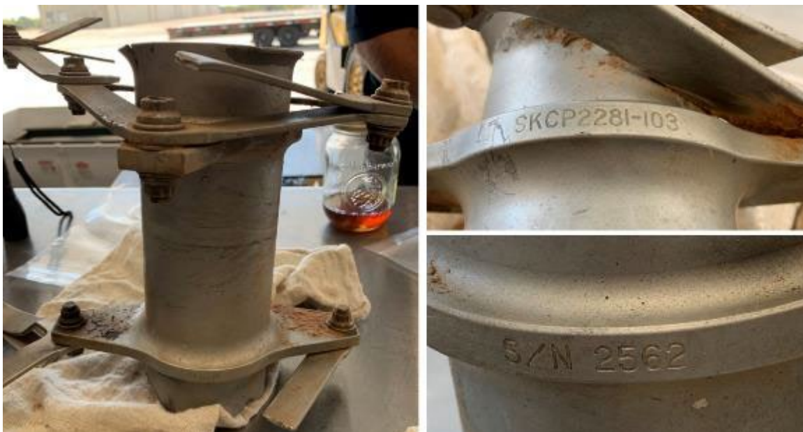
PHOTO 10: KAFLEX DRIVESHAFT COUPLING INTERCONNECT SHAFT, WITH P/N AND S/N
