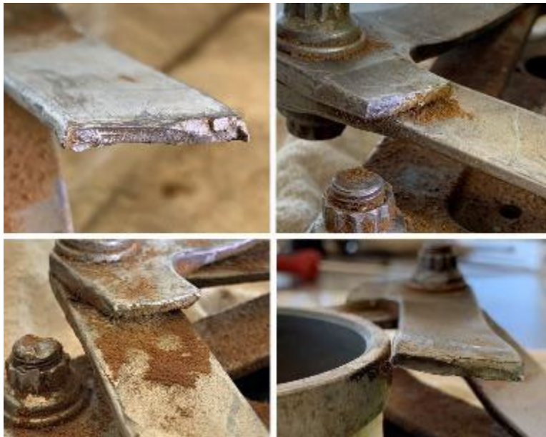
PHOTO 14: BROKEN FLEX FRAMES ATTACHED TO THE ENGINE END FITTING
