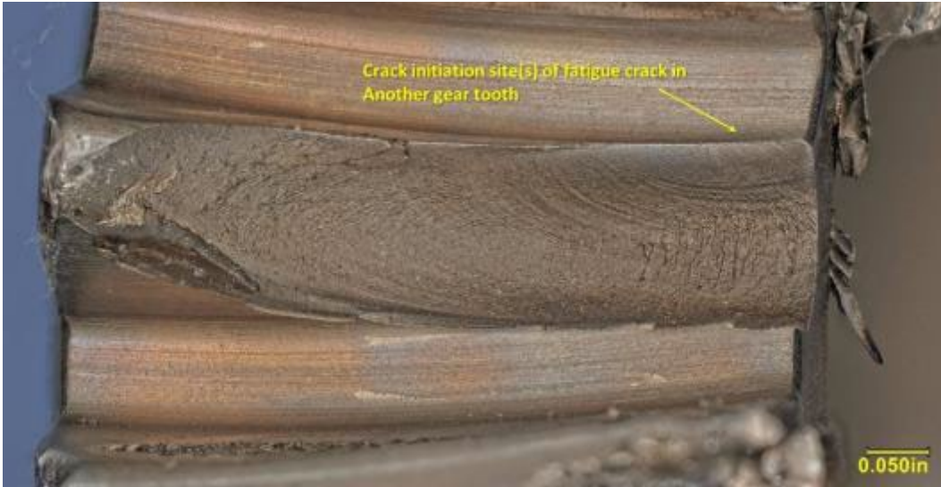
PHOTO 35: GOUGING ON ZEROL GEAR TOOTH
