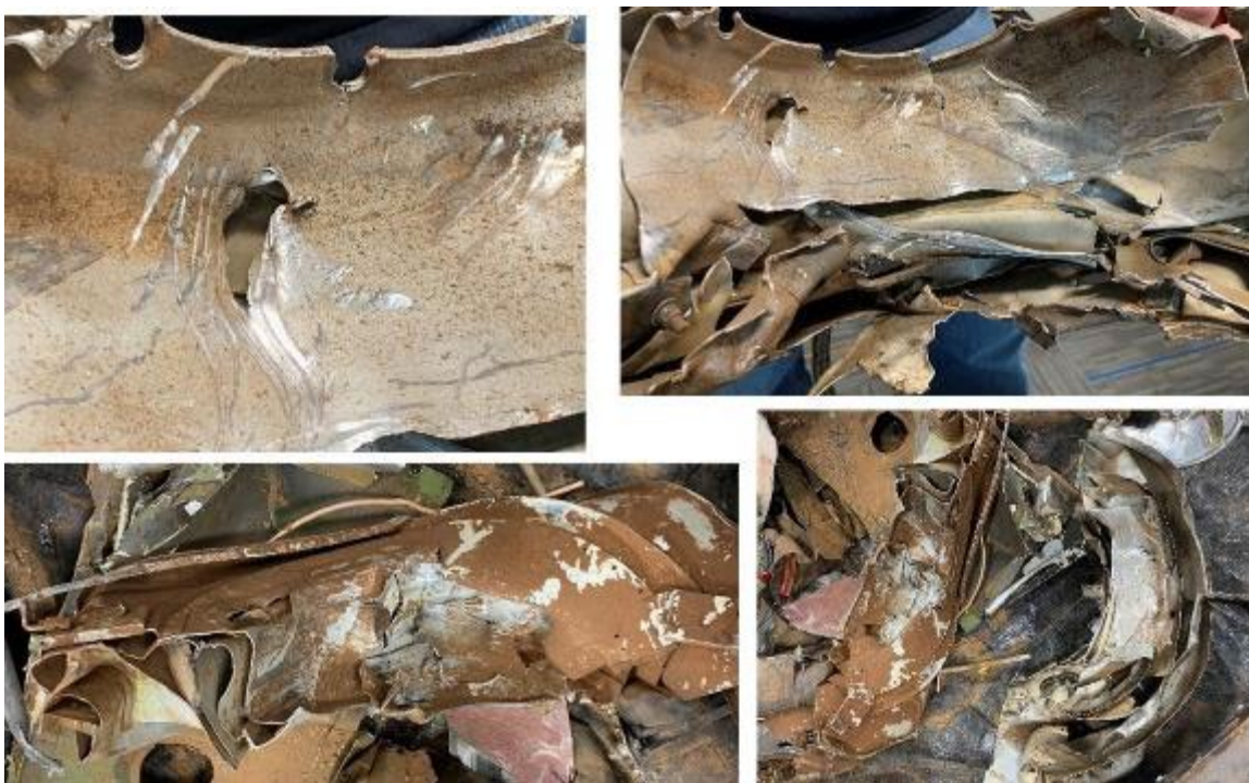
PHOTO 20: AIRFRAME COWLING AROUND THE PARTICLE SEPARATOR AND DRIVESHAFT
