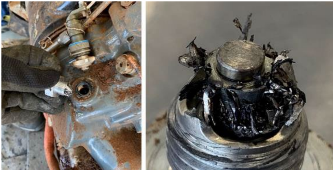
PHOTO 6: N1 AGB CHIP DETECTOR WITH DEBRIS
