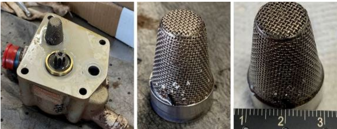
PHOTO 8: SCAVENGE FUEL PUMP (LEFT) AND STRAINER W/DEBRIS (CENTER, RIGHT)
