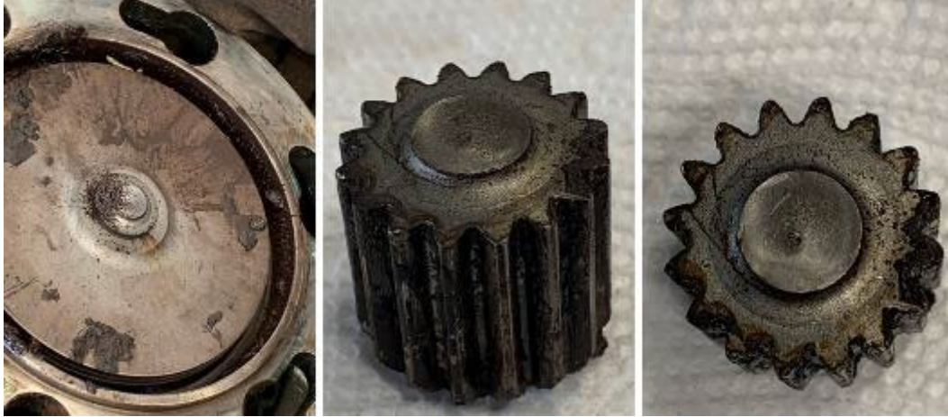
Photo 5: Sheared Starter-Generator Driveshaft
