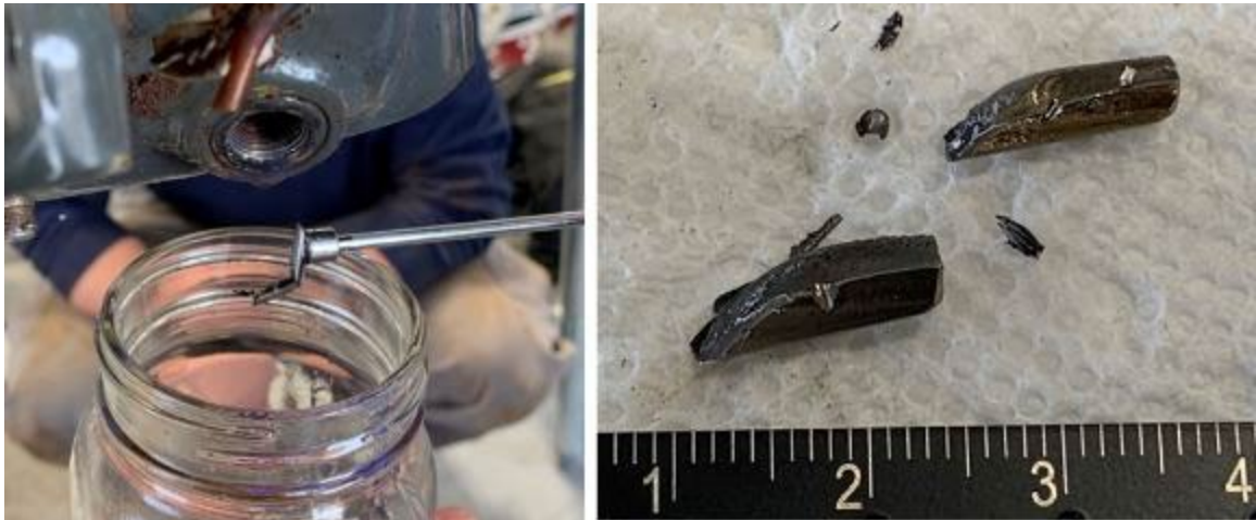
PHOTO 9: GEAR TEETH FOUND IN THE N1 AGB
