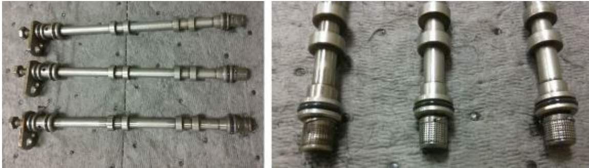
PHOTO 22: RGB ACR INDUSTRIES INC OIL TRANSFER TUBES AND FILTERS
