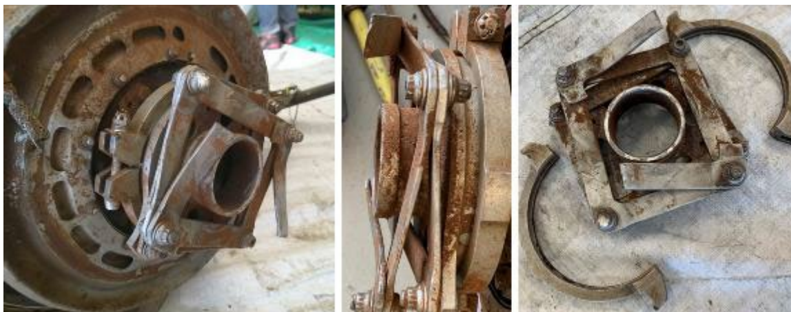
PHOTO 11: ENGINE-SIDE END FITTING (LEFT), FLEX FRAMES (CENTER), AND RETAINING CLAMP (RIGHT)
