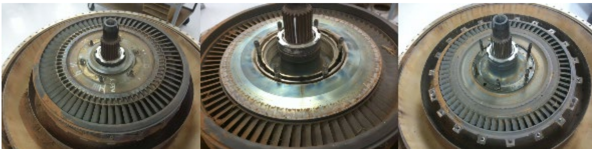
PHOTO 30: 2 ND STAGE GP ROTOR (L), 2 ND STAGE NOZZLE (C), 1 ST STAGE ROTOR (R)
