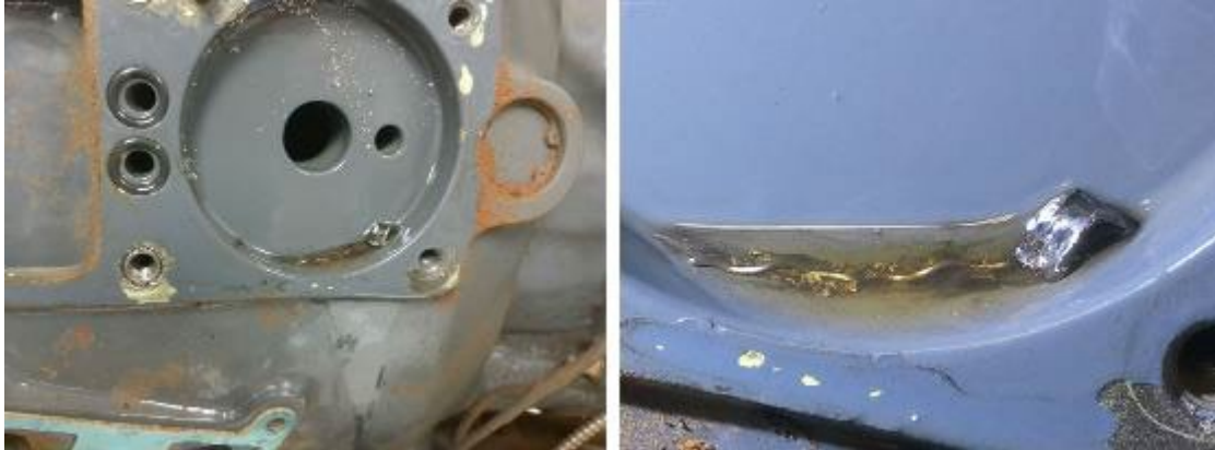
PHOTO 25: METALLIC FRAGMENTS ON THE N2 OVERSPEED GOVERNOR MOUNT PAD
