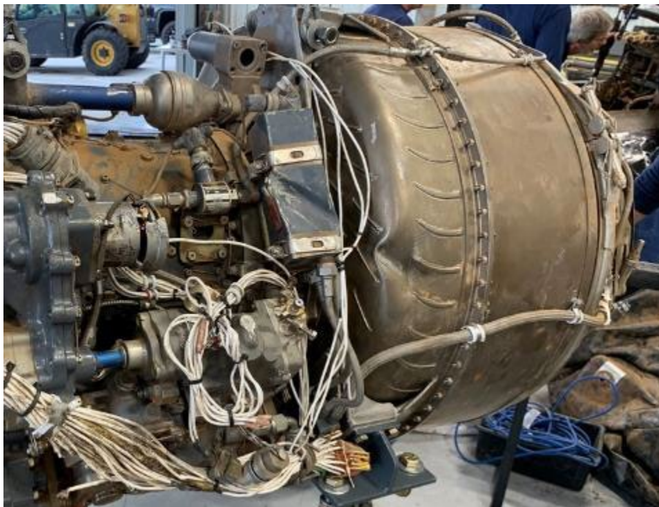
PHOTO 4: DENT ON THE IGNITER AND AIR DIFFUSER
