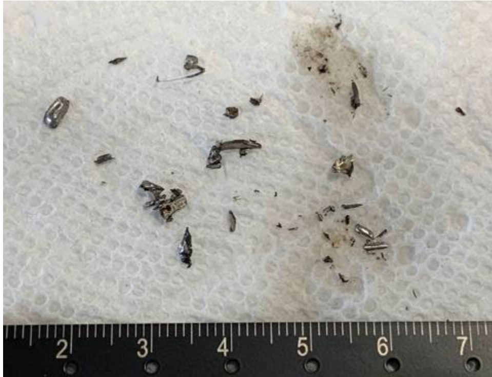
PHOTO 7: DEBRIS FROM THE N1 AGB
