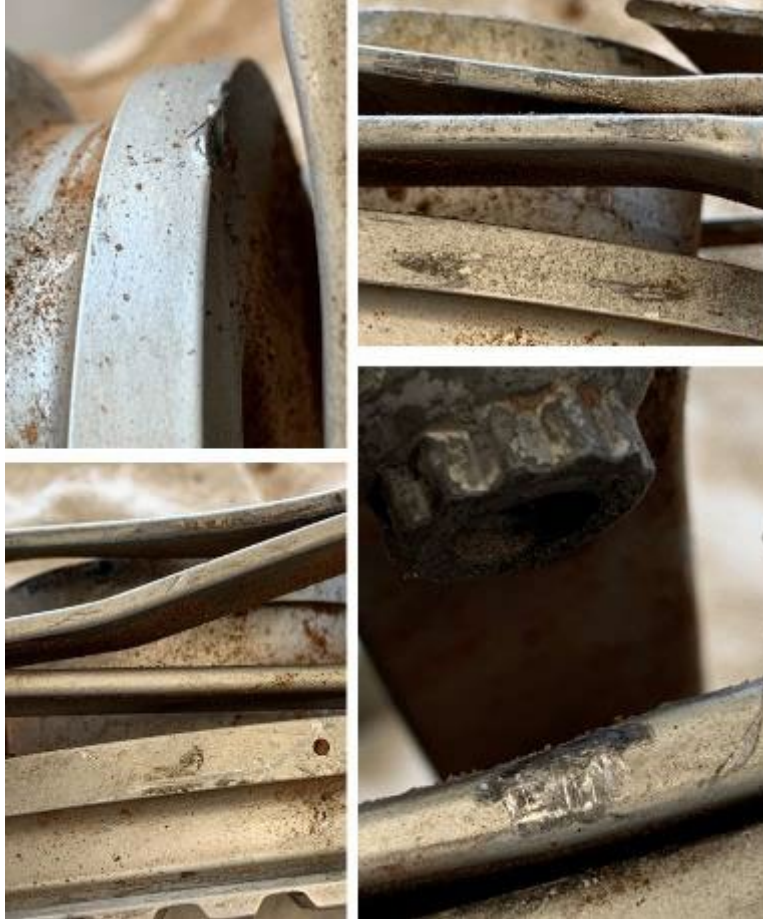
PHOTO 13: CONTACT DAMAGE ON THE ENGINE END FITTING FLEX FRAMES
