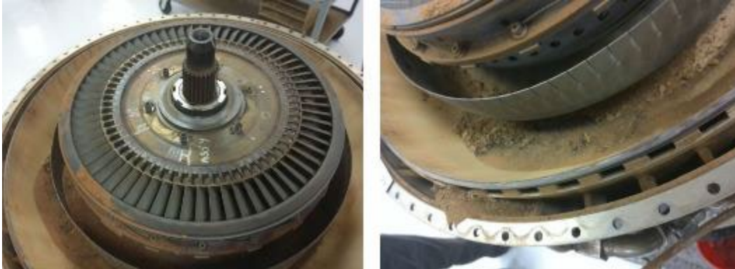
PHOTO 29: COMBUSTION CHAMBER DEFLECTOR, WITH DIRT BUILD-UP AT THE 6:00 O'CLOCK POSITION
