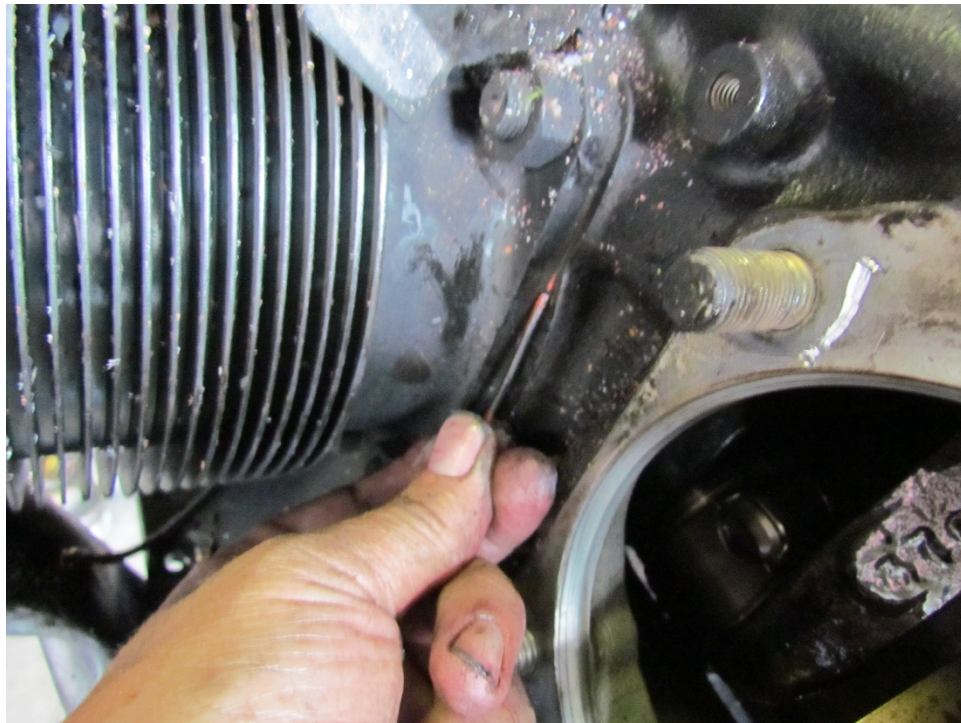
Figure 19: Extruding O-ring on Number 5 cylinder
