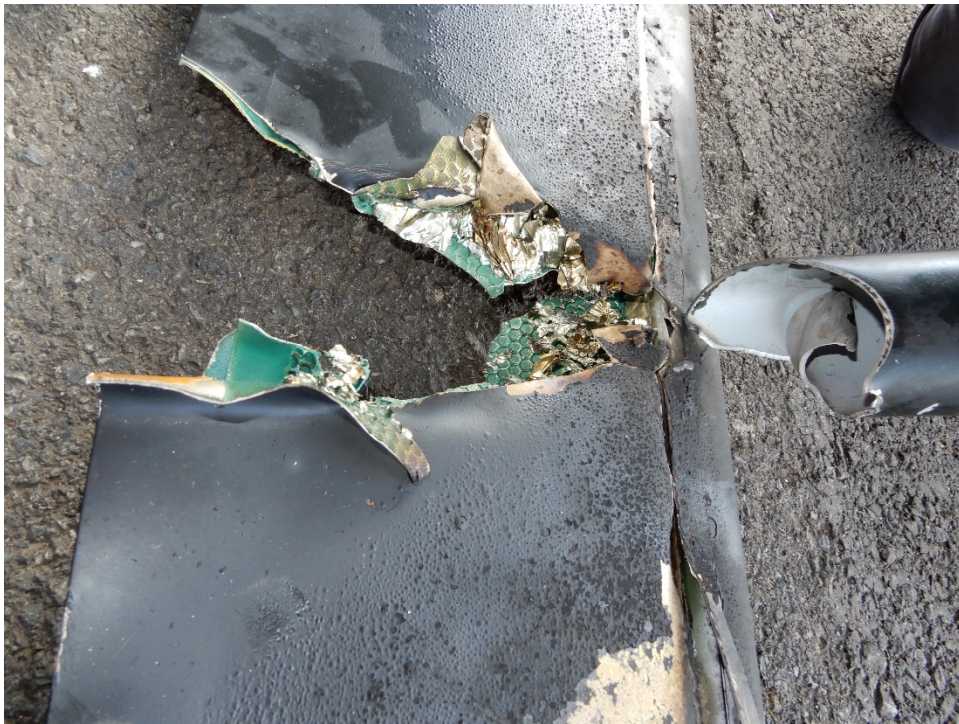
Figure 3: Afterbody damage to the Blue Blade Compared to the Left Skid Toe
