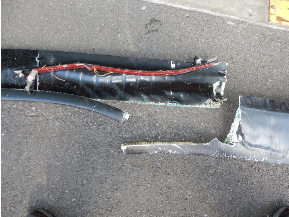
Figure 2: Rotational Scoring in the Red Blade
