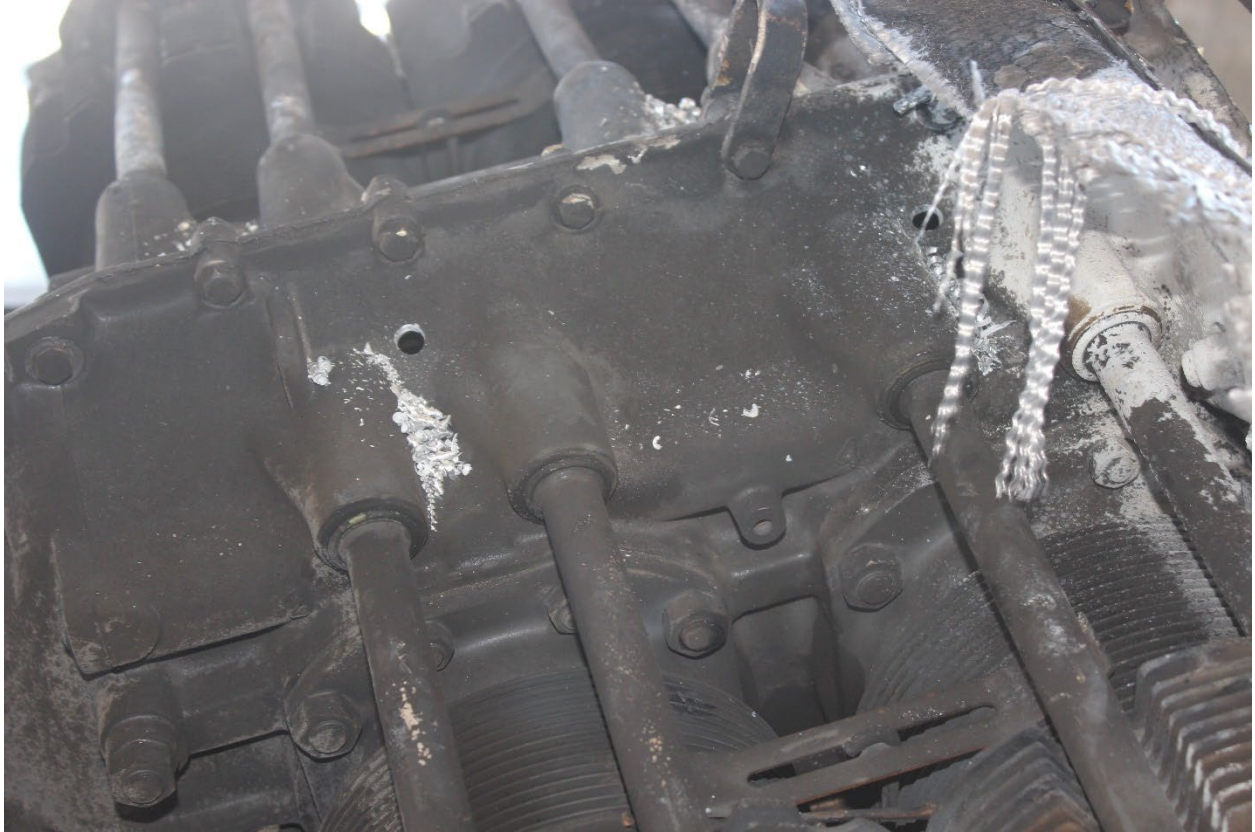
Figure 29. Two of four holes drilled into cases. Photo Lycoming.
