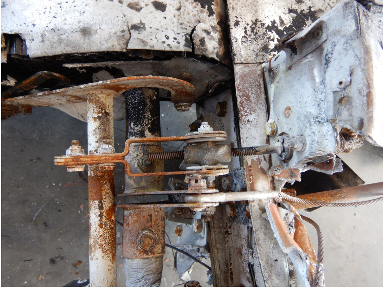
Figure 14. Center section of the elevators.
