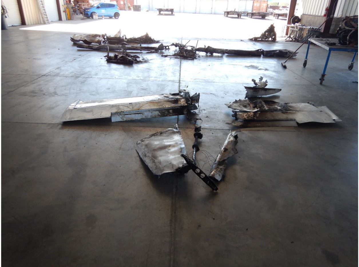
Figure 13. Rear view of the empennage, showing the rudder and vertical stabilizer.
