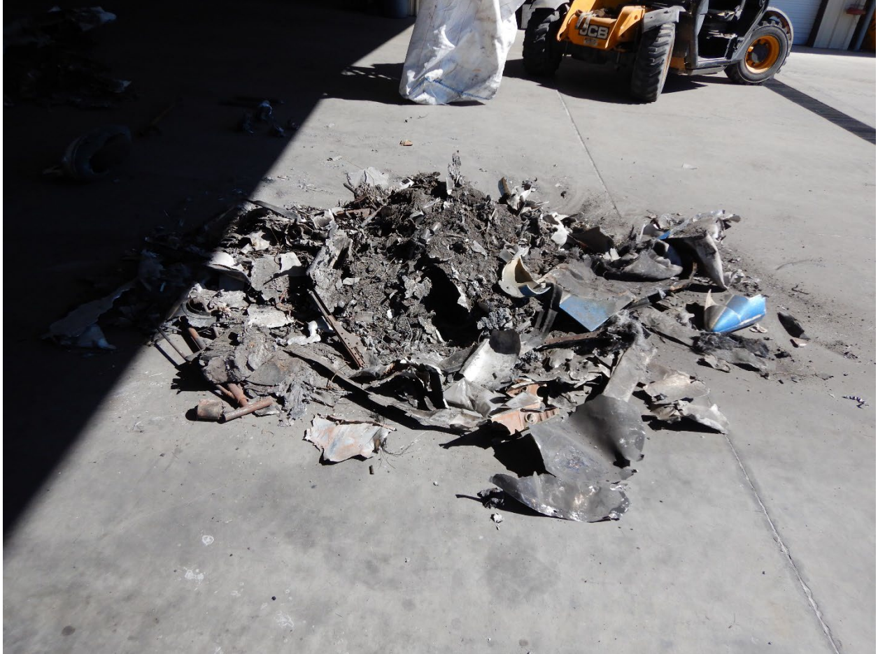
Figure 16. Second bag containing wreckage debris including, nose wheel, and main landing gear brake assemblies.
