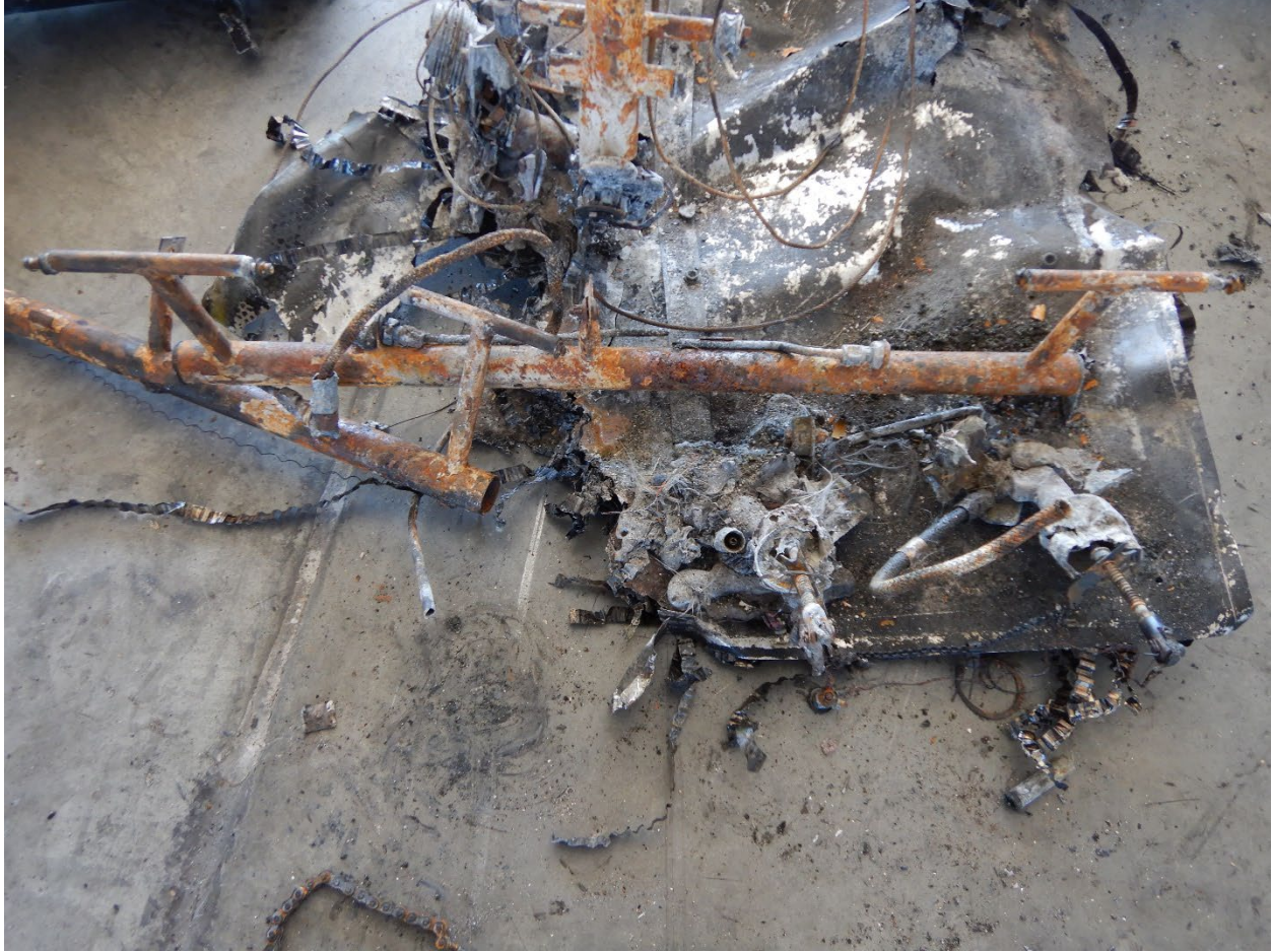
Figure 9. Rudder pedal assembly with control cables attached.
