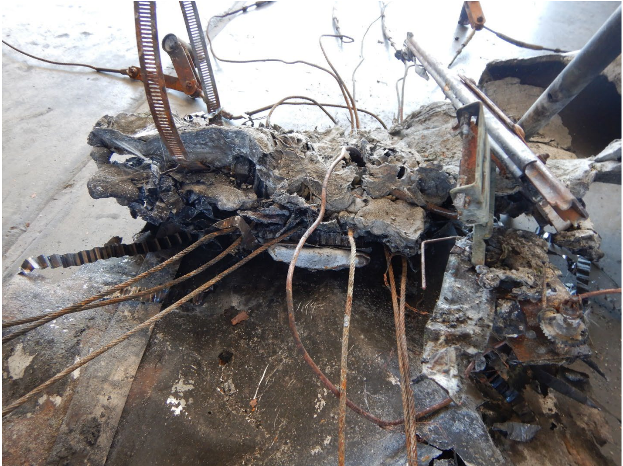
Figure 10. Flight control cables from the control yoke and the rudder pedals running through solidified aluminum.
