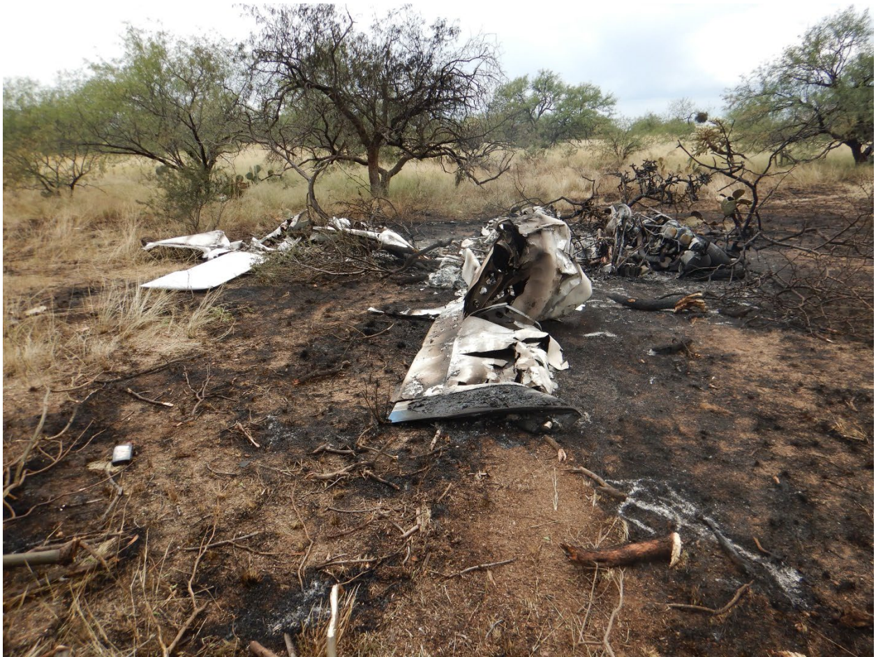
Figure 1. View of N74349 at the accident site, showing the right wing, aileron, flap, the right side of the empennage and the right side of the engine.
