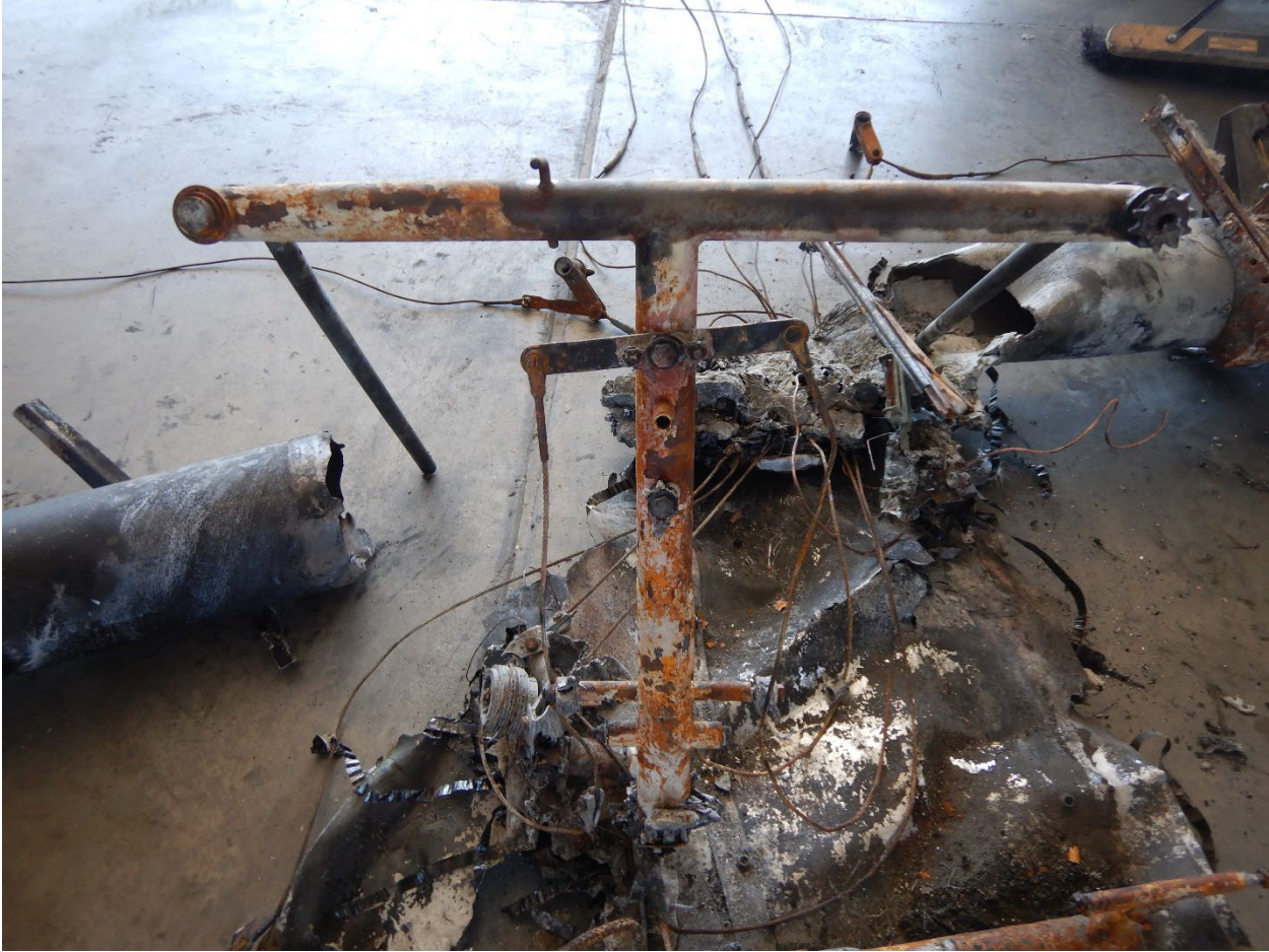
Figure 4. Control yoke assembly with control cables attached.
