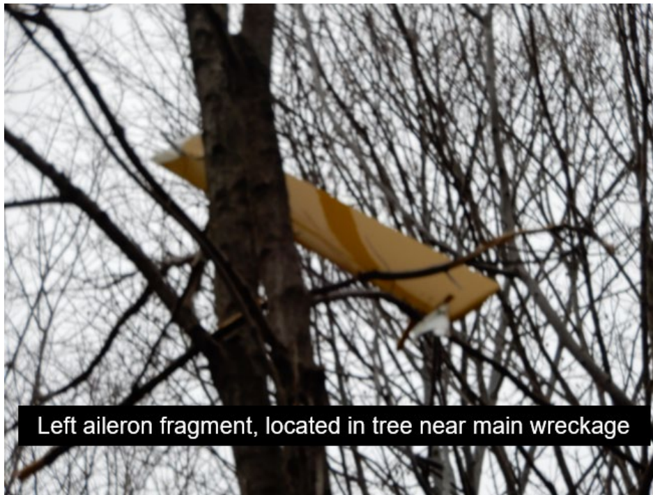
Figure 2: View of an aileron fragment lodged in a tree near the main wreckage (NTSB Photo)
