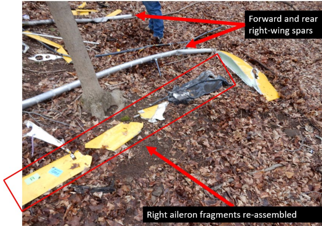
Figure 11: The right-wing aileron fragments laid out at the accident site (NTSB Photo)
