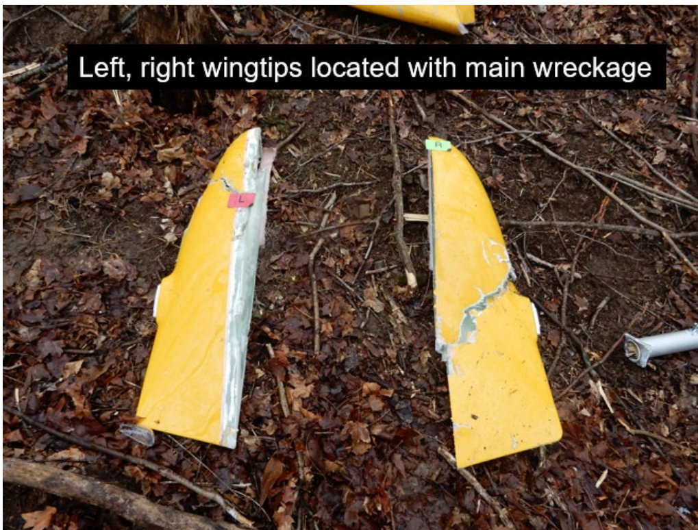
Figure 4: View of the left and right wingtips laid out at the accident site (NTSB Photo)
