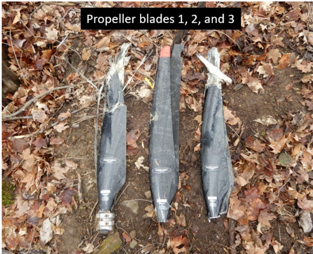
Figure 12: View of all three propeller blades laid out at the accident site (NTSB Photo)
