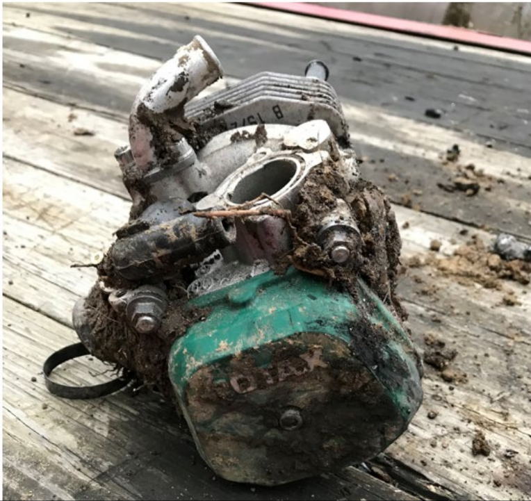
No. 2 Engine Cylinder, Separated from Engine
