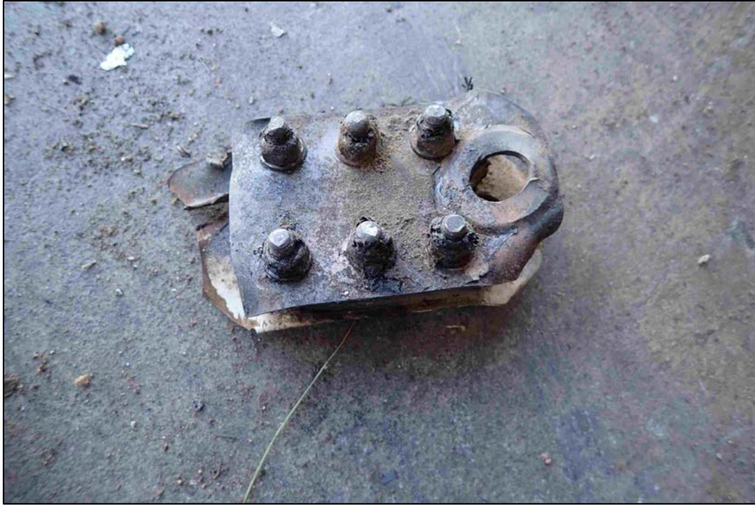
Photo 22 – Left Aft Attachment Lug
