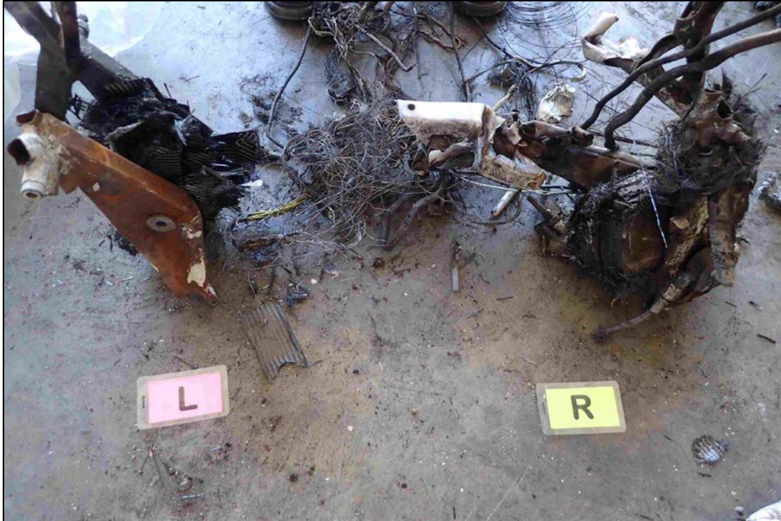
Photo 20 – Wing Main Spar Flanges
