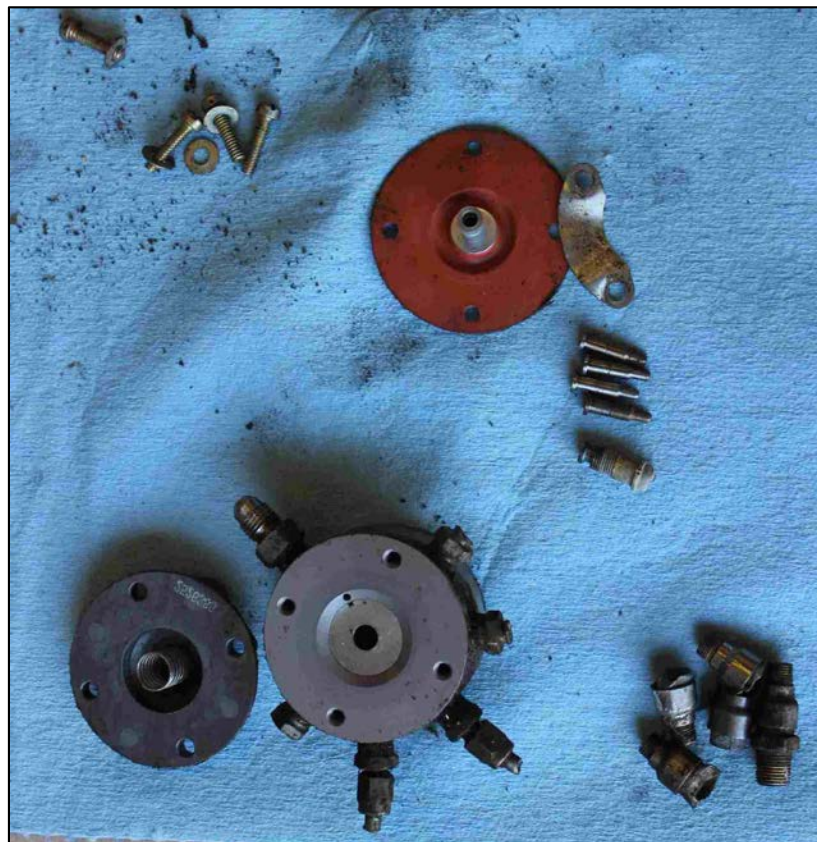
Photo 44 – Fuel Flow Divider Components
