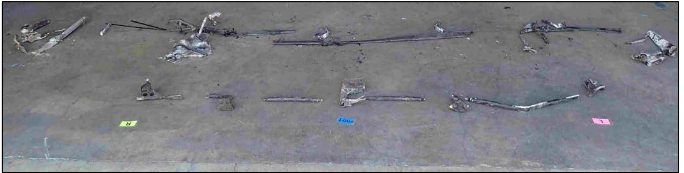
Photo 15 – Aileron Control System Remnants
