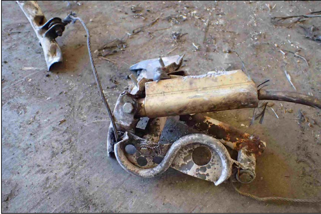
Photo 10 – Left Rudder Cable
