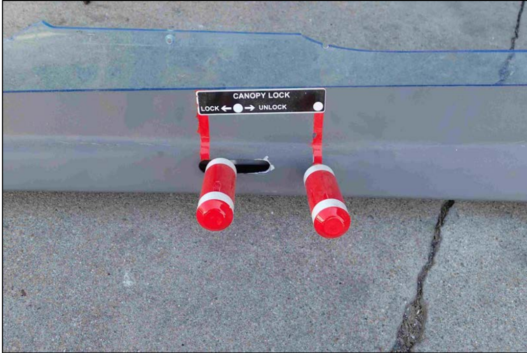
Photo 36 – Left Rear Locking Handles
