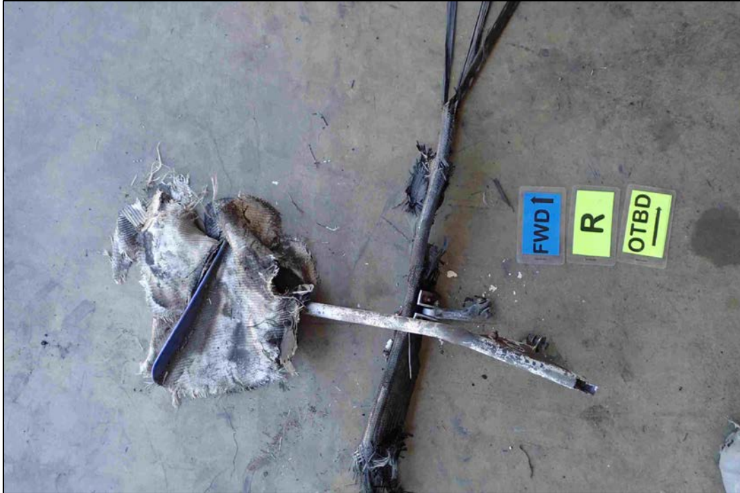
Photo 16 – Right Aileron Spade
