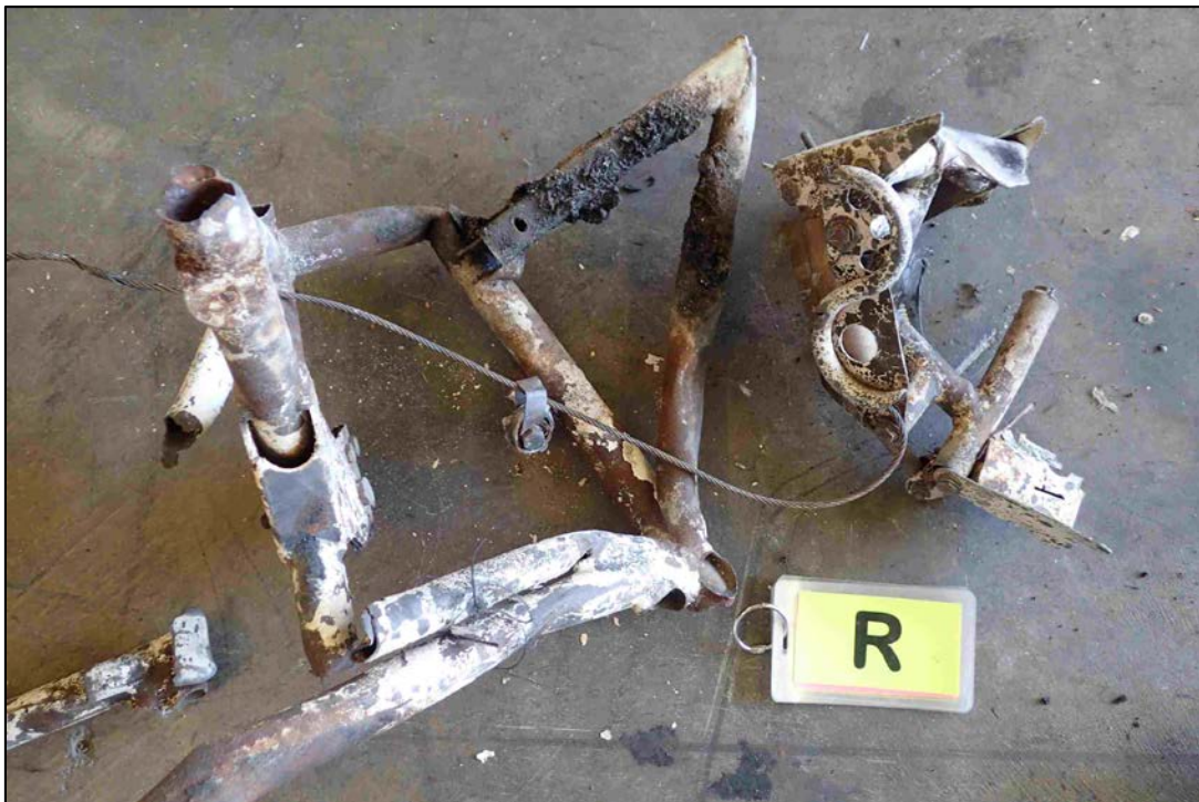
Photo 9 – Right Rudder Cable
