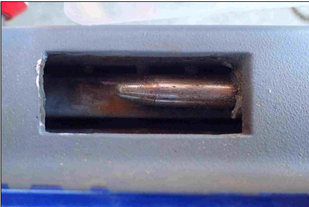
Photo 33 – Canopy Center Locking Pin
