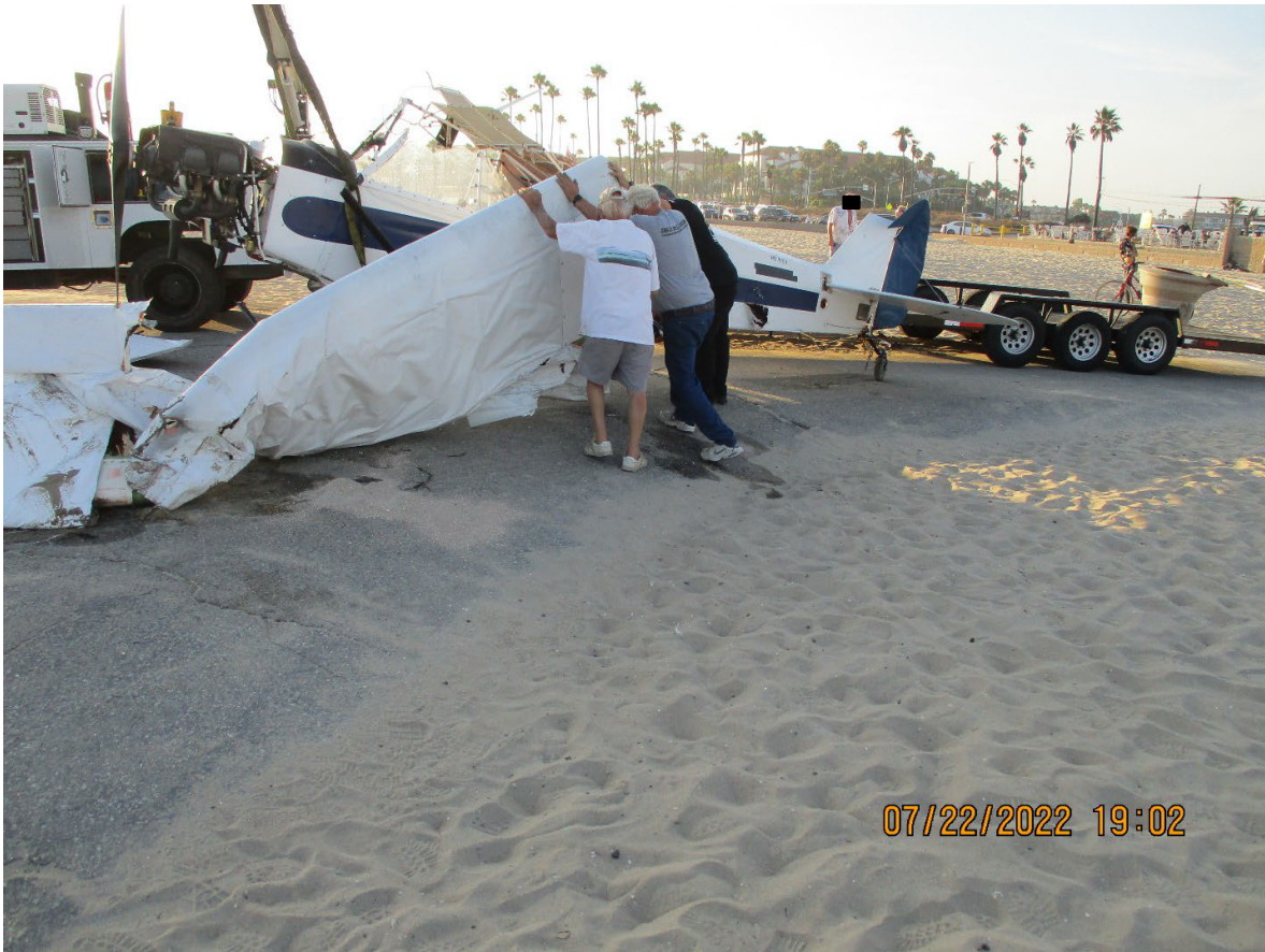
Figure 3. Left wing damage. Photo FAA.
