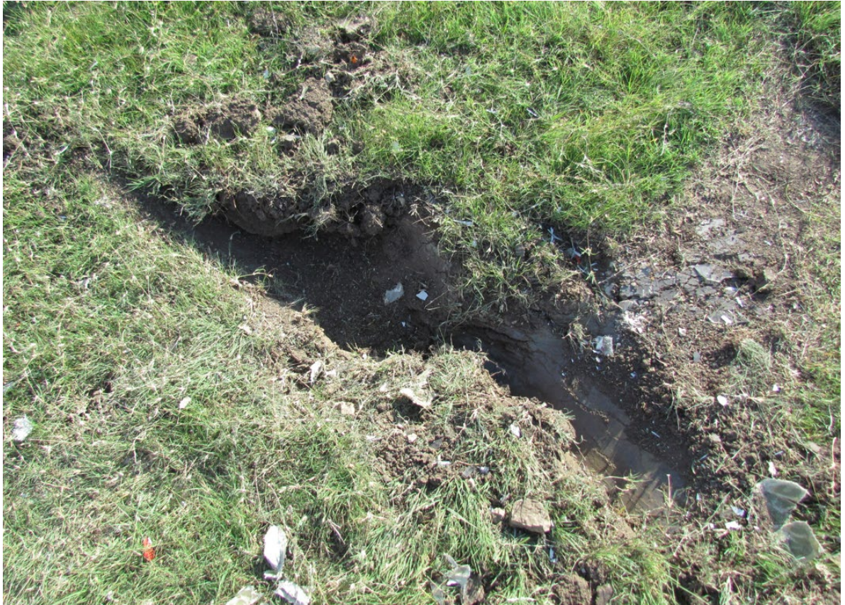
Photo 2 – Propeller Ground Scar After Wreckage Debris was Removed
