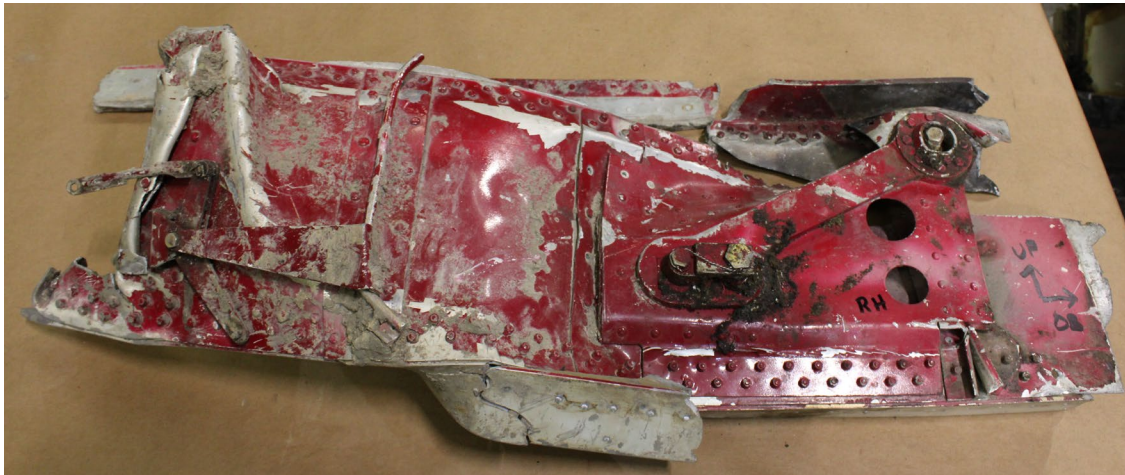
Figure 7 – Right wing main spar aft side, wing station 26 to 57 (NTSB photo)
