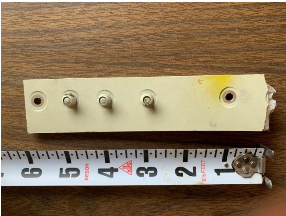
Figure 4 - Section of the upper cap splice plate of the main wing spar (NTSB Photo)
