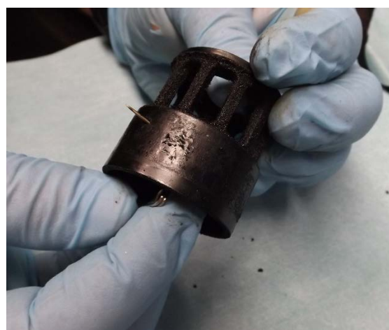
PHOTO 14: NO. 1 ENGINE REAR BEARING SUPPORT CAGE OIL PASSAGE CLEAR
