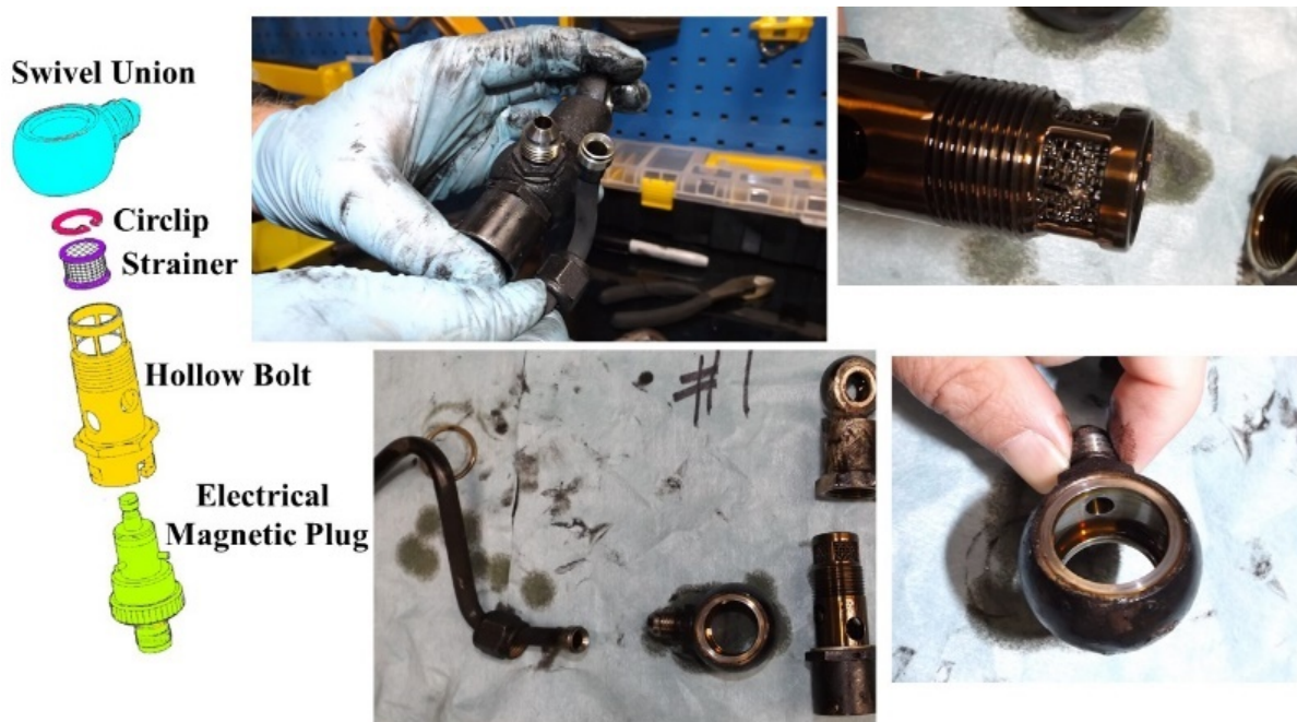
PHOTO 15: NO. 1 ENGINE REAR BEARING SCAVENGE
