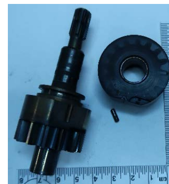
PHOTO 26: FUEL PUMP GEAR UNDAMAGED
