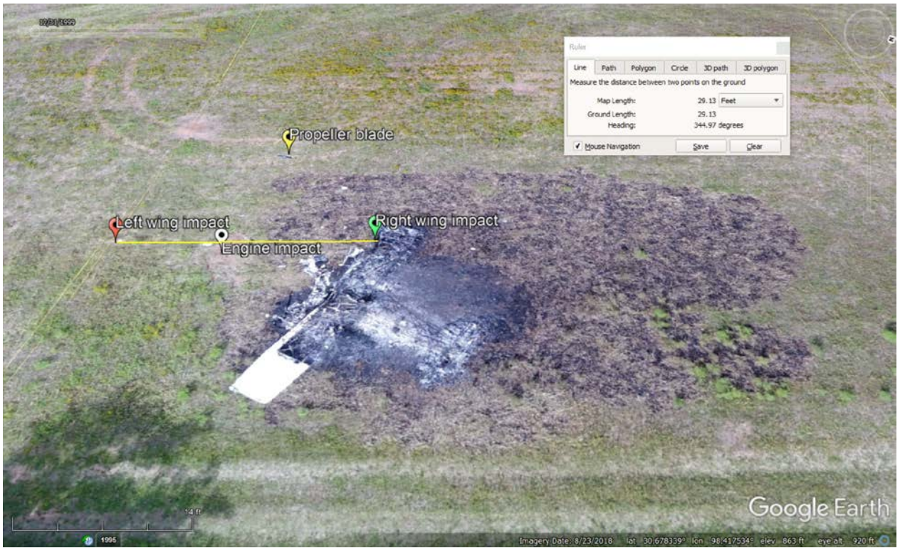
Figure 4 – Google Earth of wreckage with impact measurement
