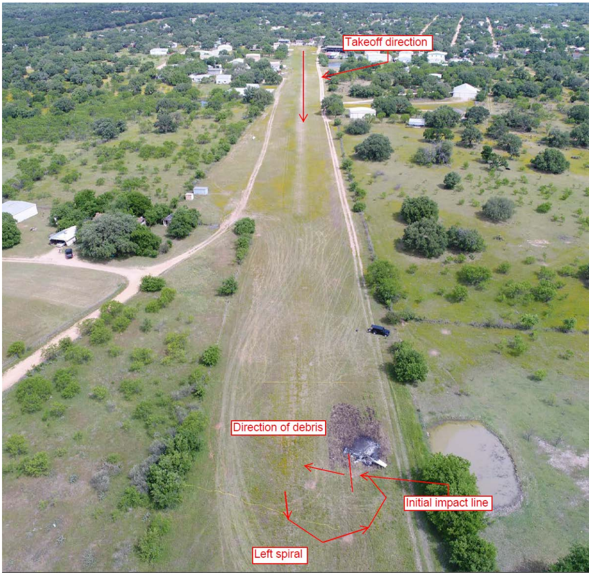
Figure 3 – Aerial runway view from south with notation. Wreckage on the lower right side
