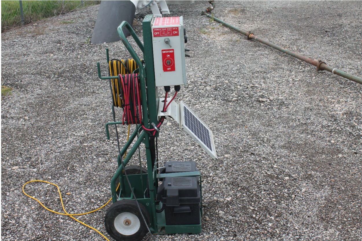
Figure 6. Ignitor - Side View (7/2/21 at 3:43PM)
