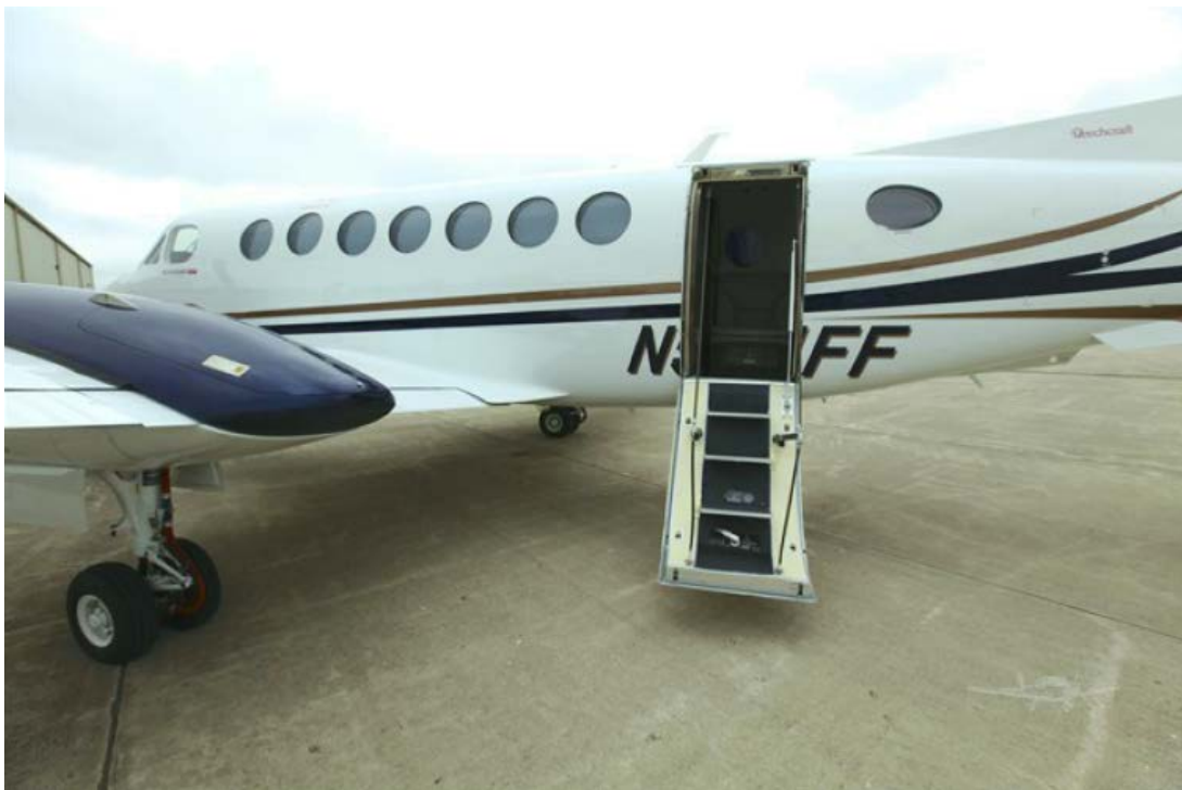
Photo 2. Left-side overwing exit (second cabin window behind cockpit) and aft entry door.
