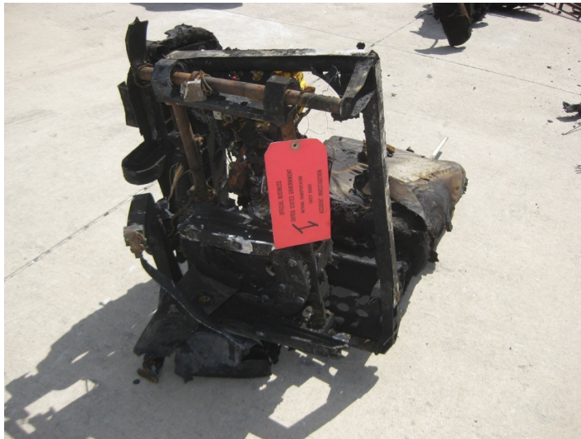
Photo 15. Damaged and charred passenger seat.
