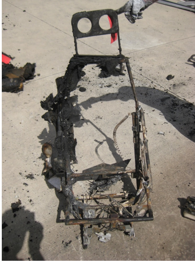
Photo 17. Fire-consumed crew seat.
