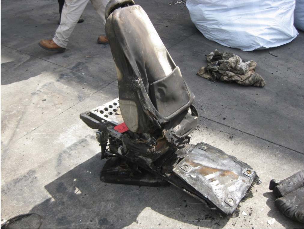
Photo 19. Damaged passenger seat still attached to a section of cabin flooring.
