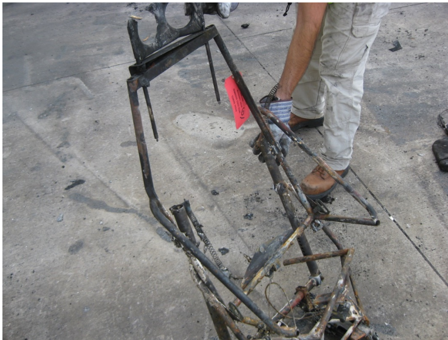
Photo 18. Fire-consumed crew seat with fractured seatpan tubes.
