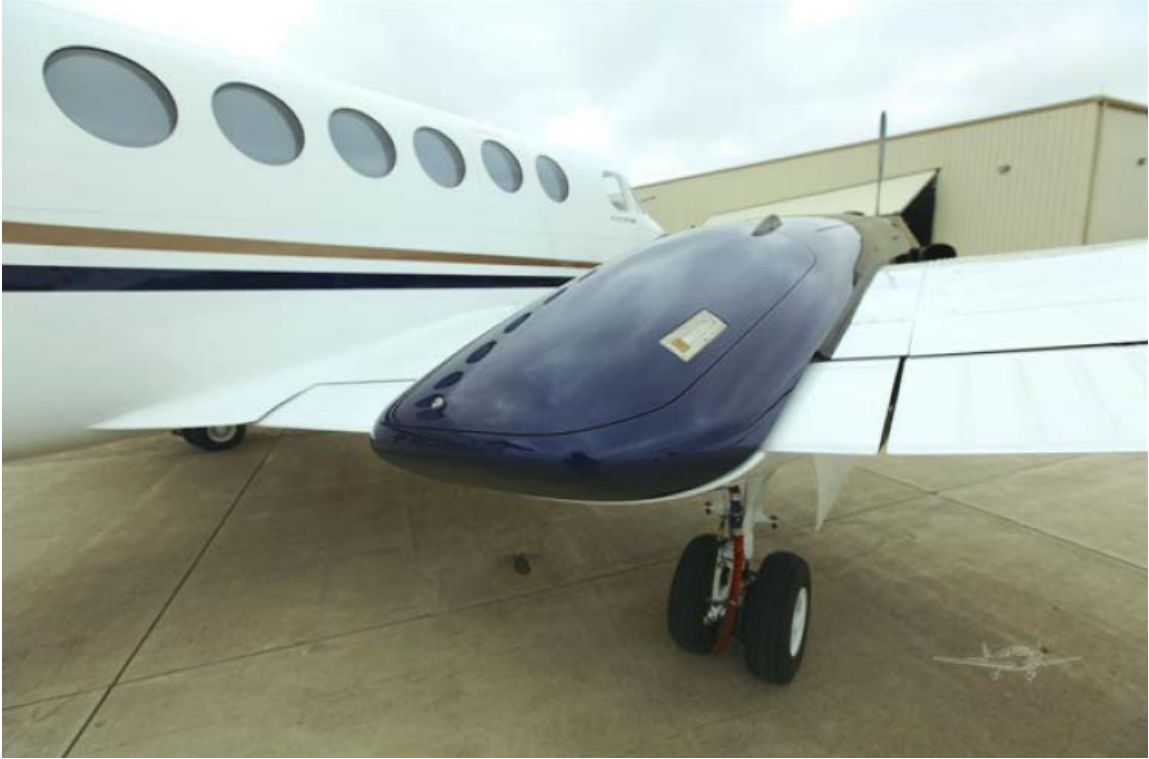
Photo 3. The right-side overwing exit (second cabin window behind cockpit).
