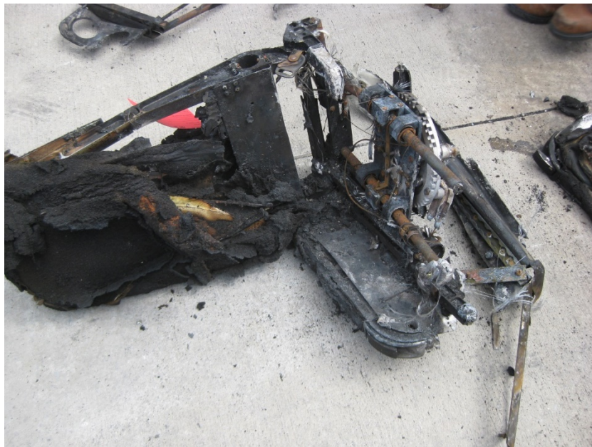
Photo 16. Damaged and charred passenger seat still attached to some seat track.
