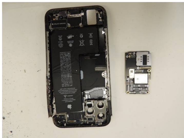
Figure 2: Motherboard of Apple iPhone 11 Pro in deformed condition.
