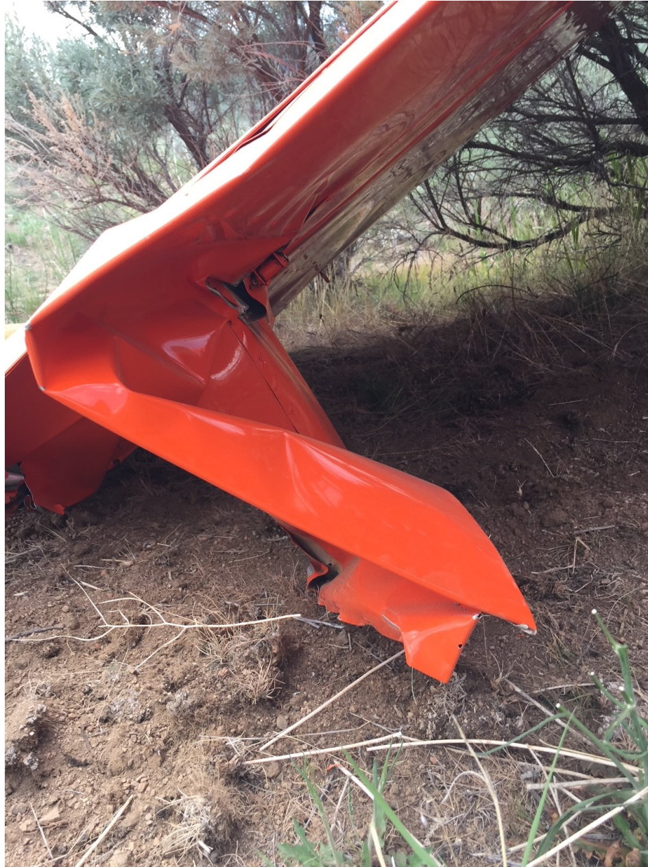
Photo 2 - View of left wing damage (photo courtesy of the pilot)
