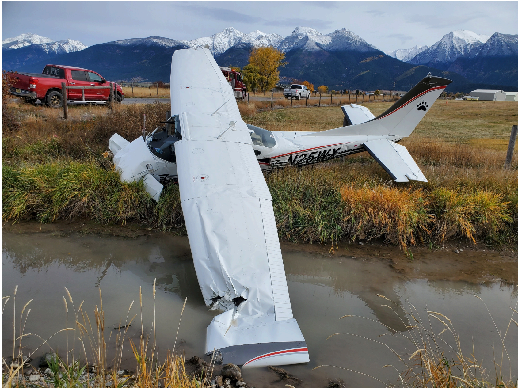
Photo 1 – View of left wing and aft fuselage damage (photo courtesy of local law enforcement)
