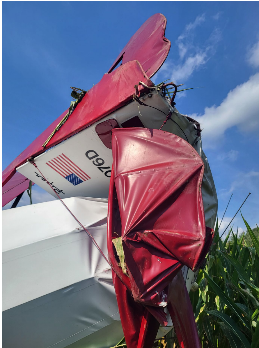
Photo 2 – View of empennage damage to elevator and rudder. (Courtesy of FAA)
