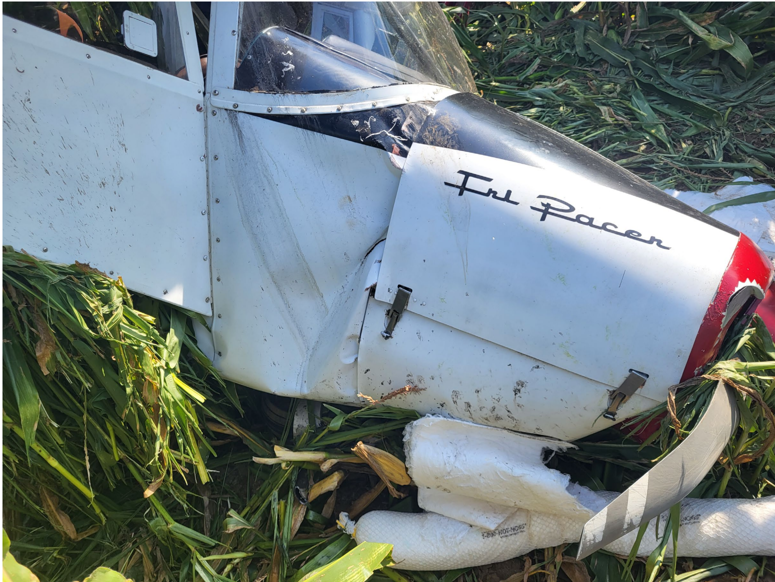
Photo 3 – Right side view of fuselage damage. (Courtesy of FAA)
