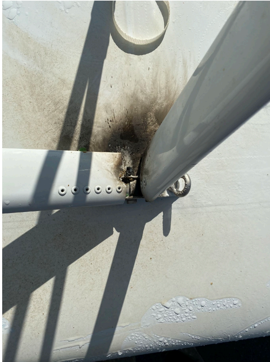
Photograph 3 - Electrical arcing damage to wing strut. (Courtesy of FAA)
