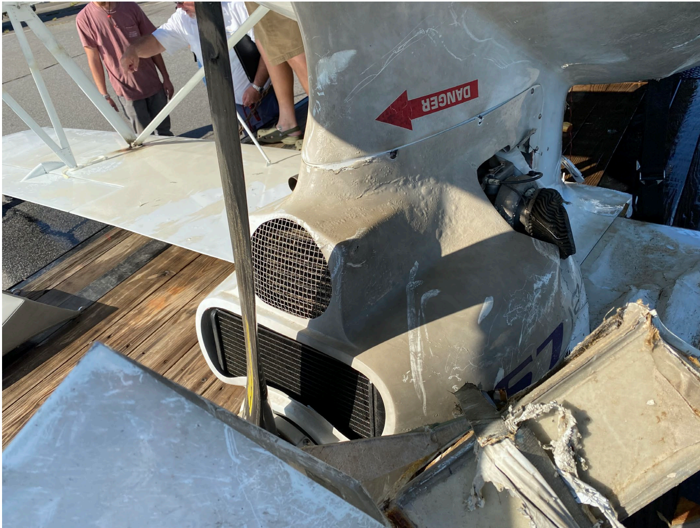
Photograph 2 - View of thermal damage to engine cowling. (Courtesy of FAA)
