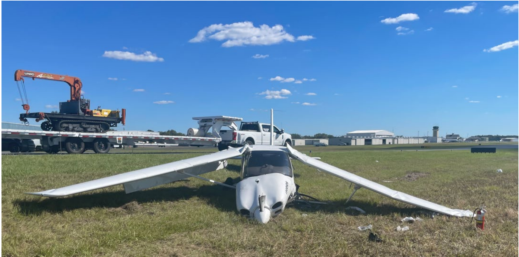
Photograph 2 - Forward view of airplane damage. Note both wings broken downwards. (Courtesy of FAA)
