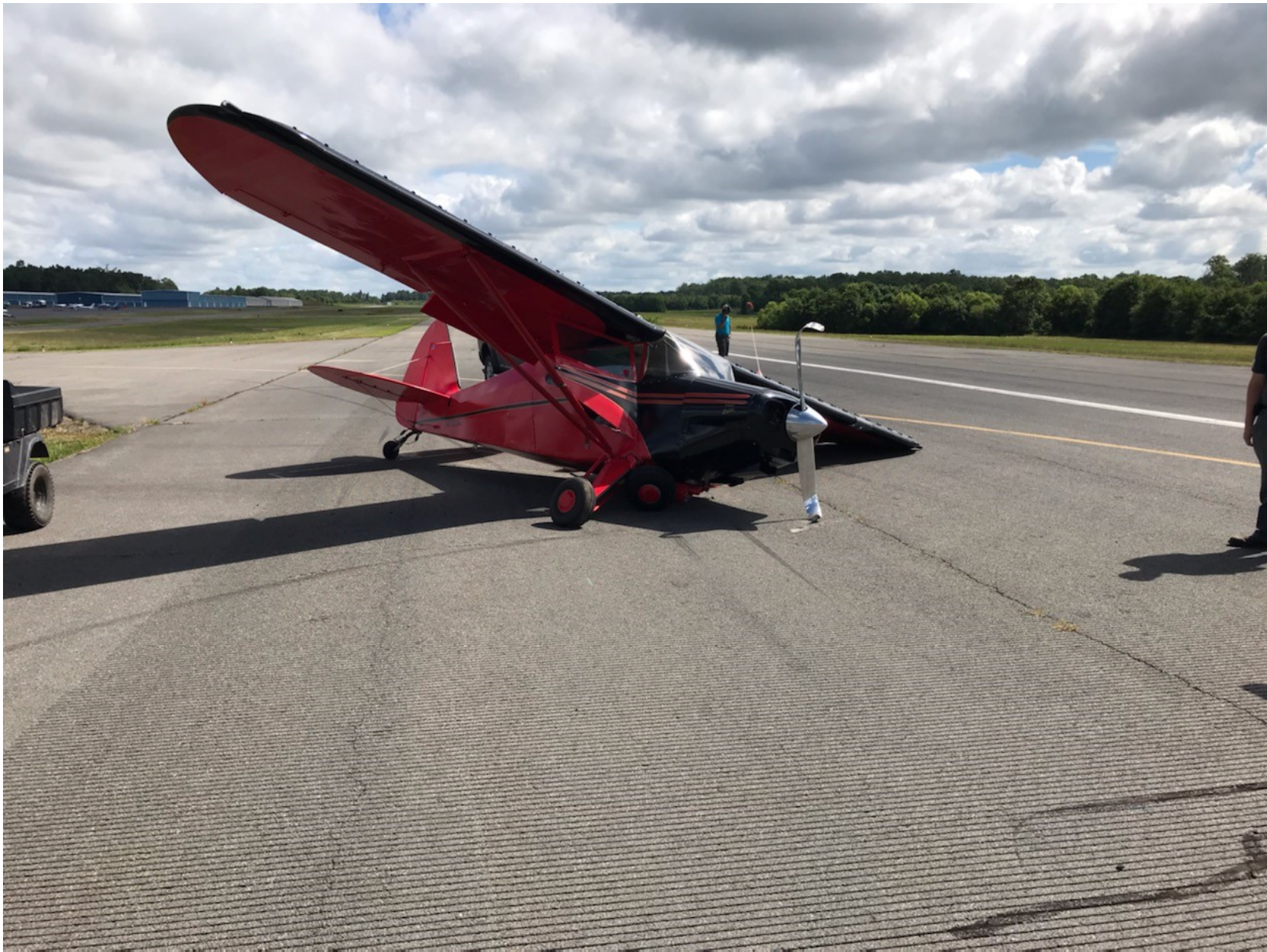
Photo 1 – View of airplane and damage as it sits on the runway. Note the fuselage wrinkles and the left landing gear bent under the fuselage. (Courtesy of CJR Airport)
