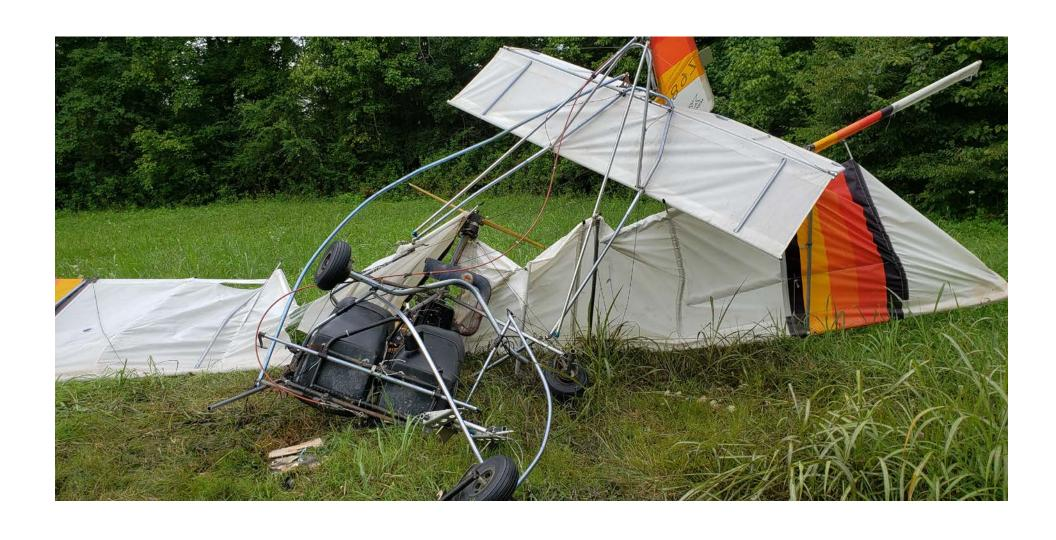
Photo 2 – View of underside of wreckage at the accident site showing the cockpit, fuselage, engine and wings.
