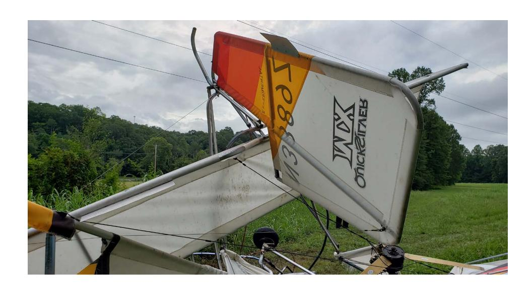
Photo 3 – Close up view of rudder and elevator. Note the bent rudder trim tab.
