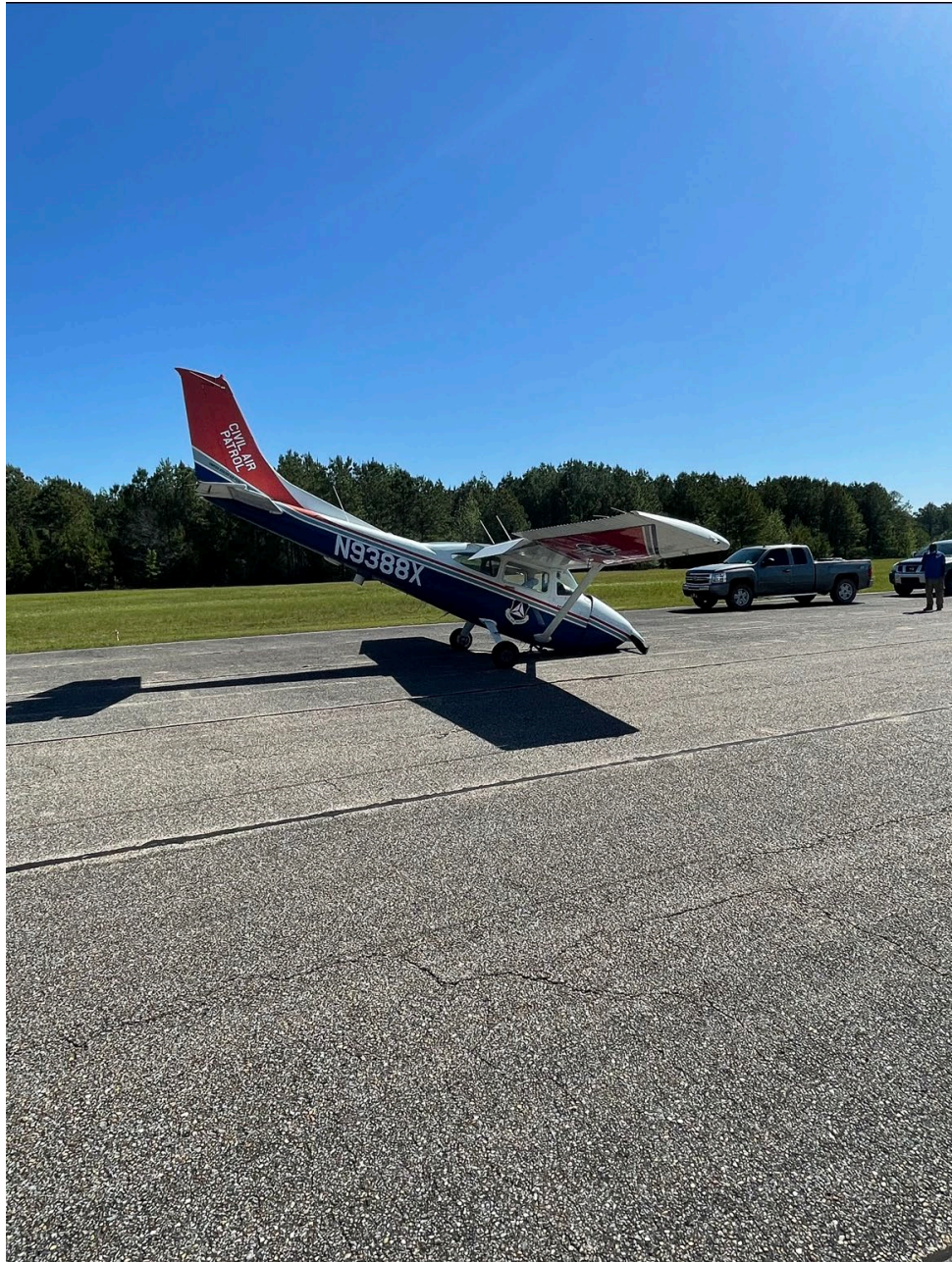
Photo 3 – View of right side of the airplane as it rests on the runway. Note damaged engine compartment. (Courtesy of the FAA)
