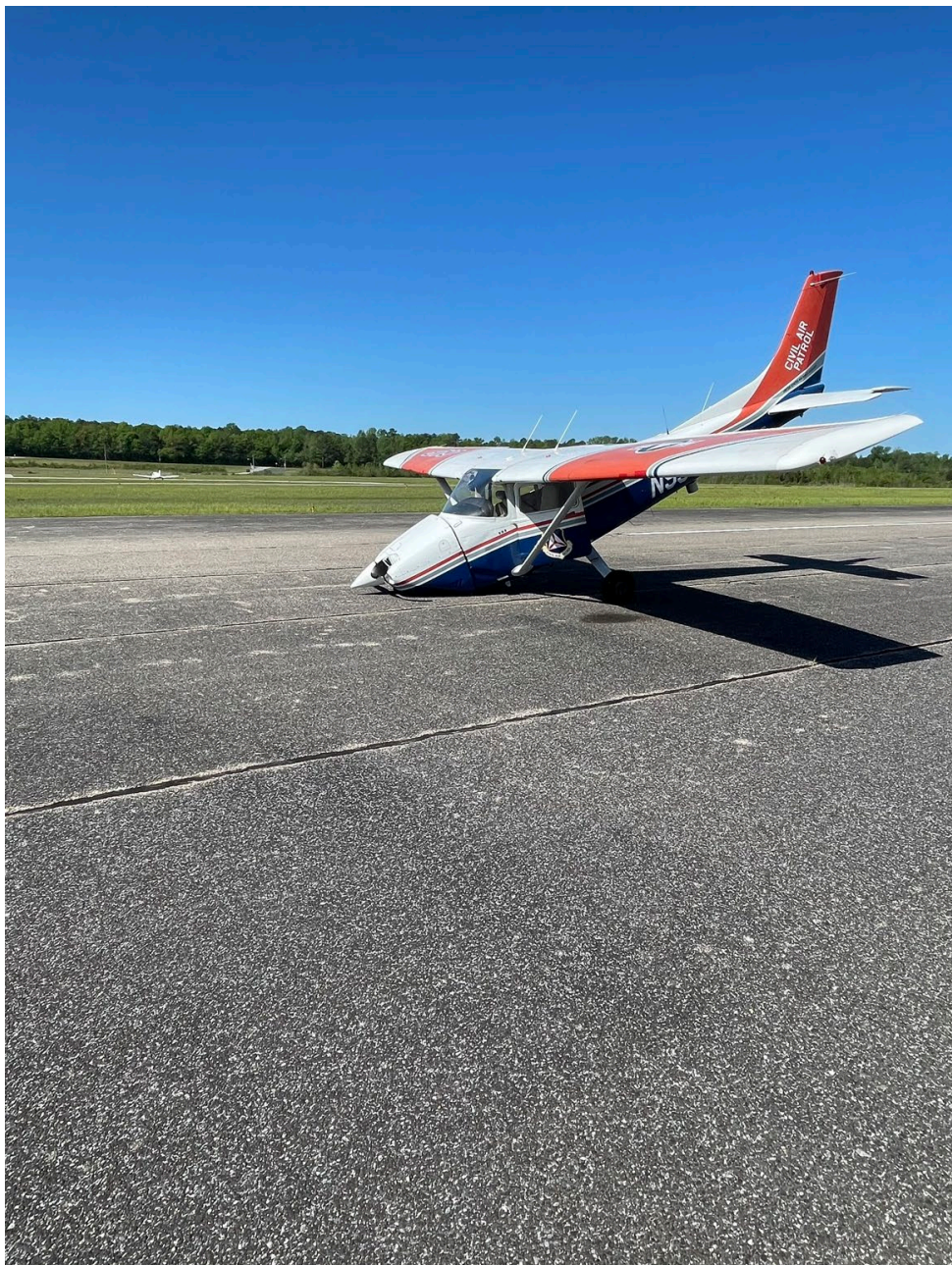
Photo 1 – View of left front quarter of the airplane as it rests on the runway. Note damaged engine compartment. (Courtesy of the FAA)
