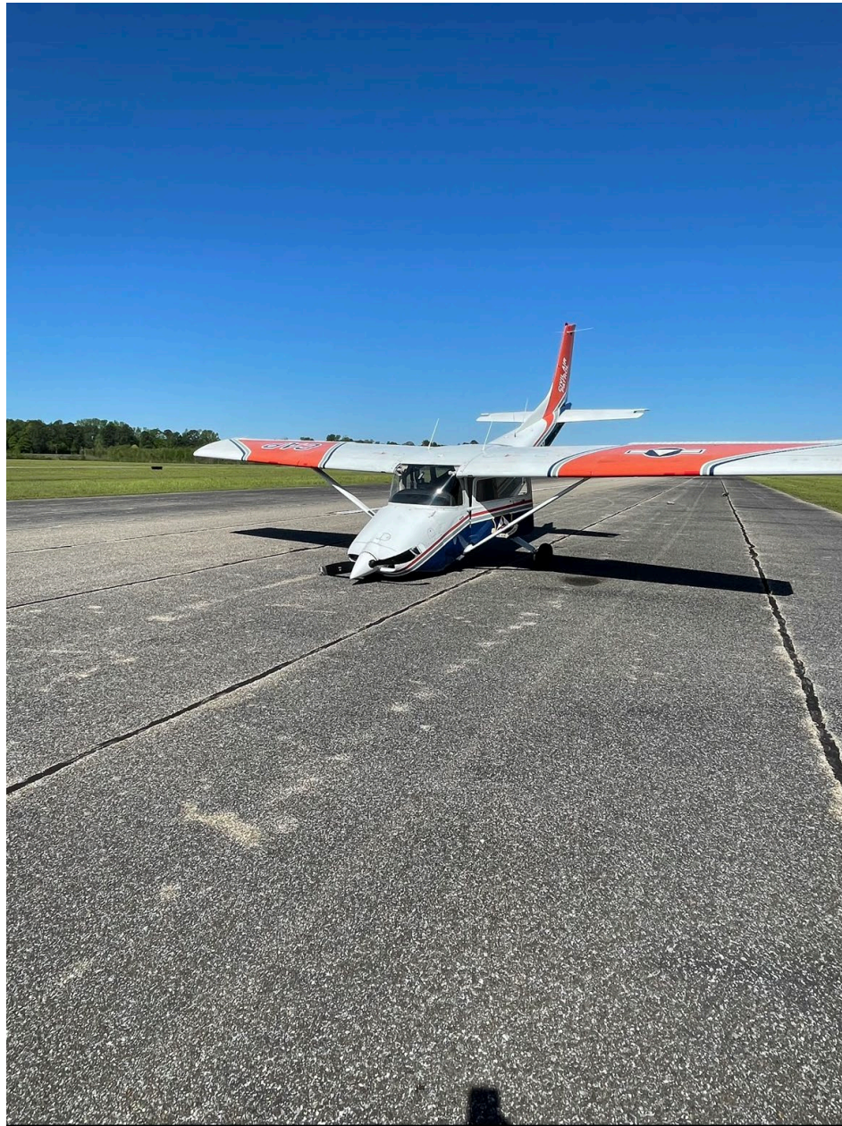
Photo 2 – View of front of the airplane as it rests on the runway. Note damaged engine compartment. (Courtesy of the FAA)
