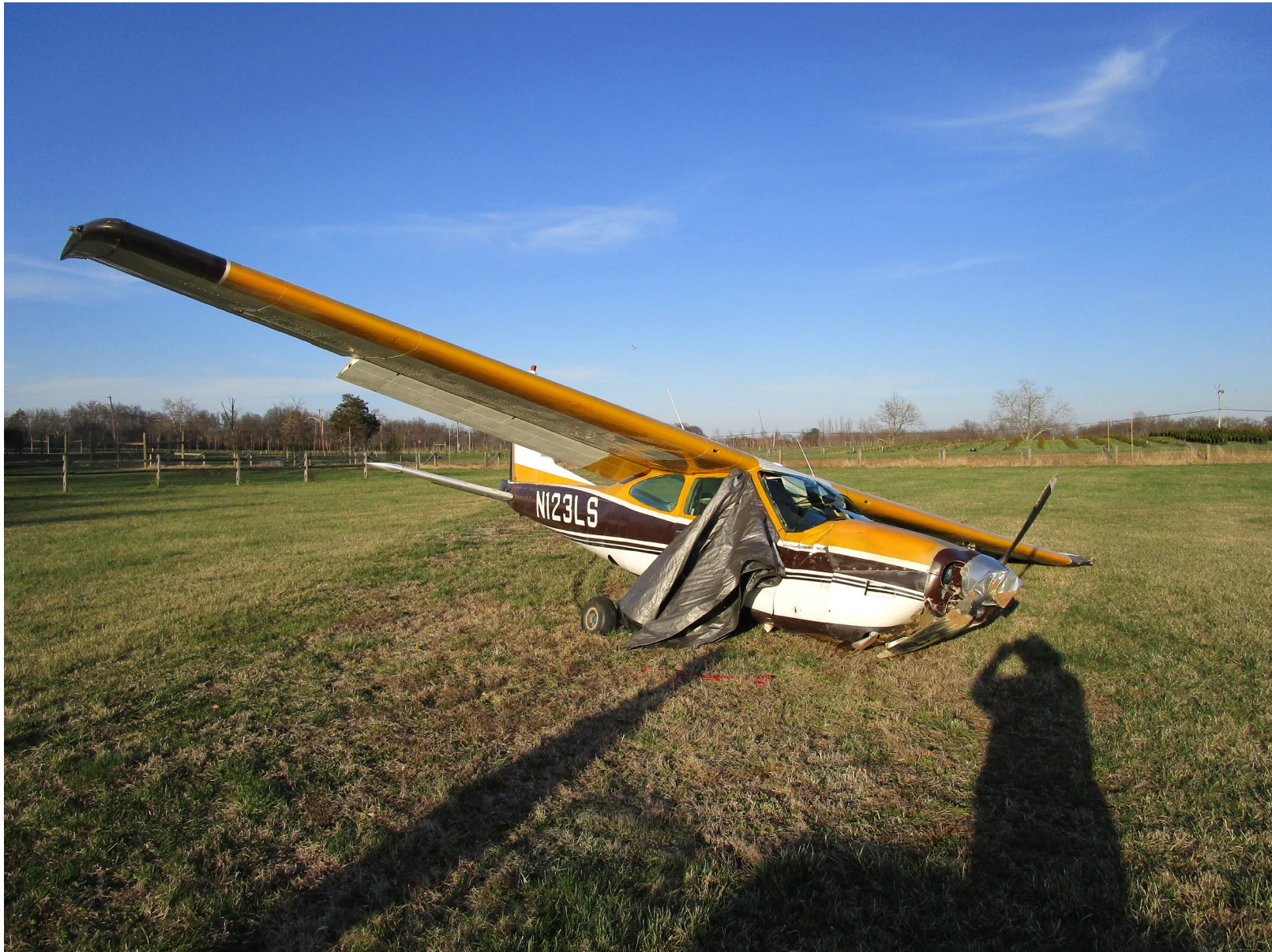
Photo 1 – Overall view of airplane damage. (Courtesy of FAA)
