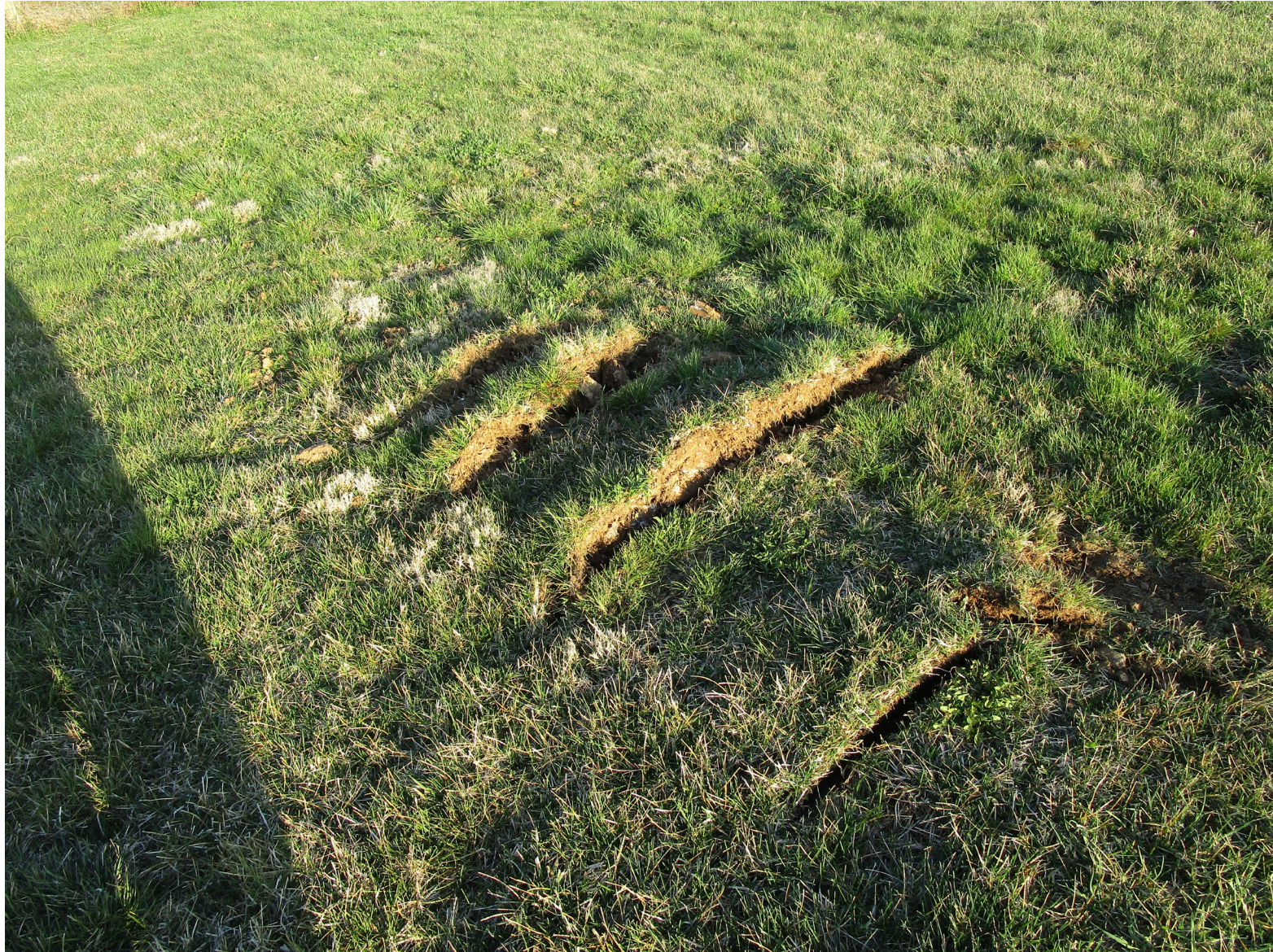
Photo 3 – View of propeller strike marks in the ground. (Courtesy of FAA)
