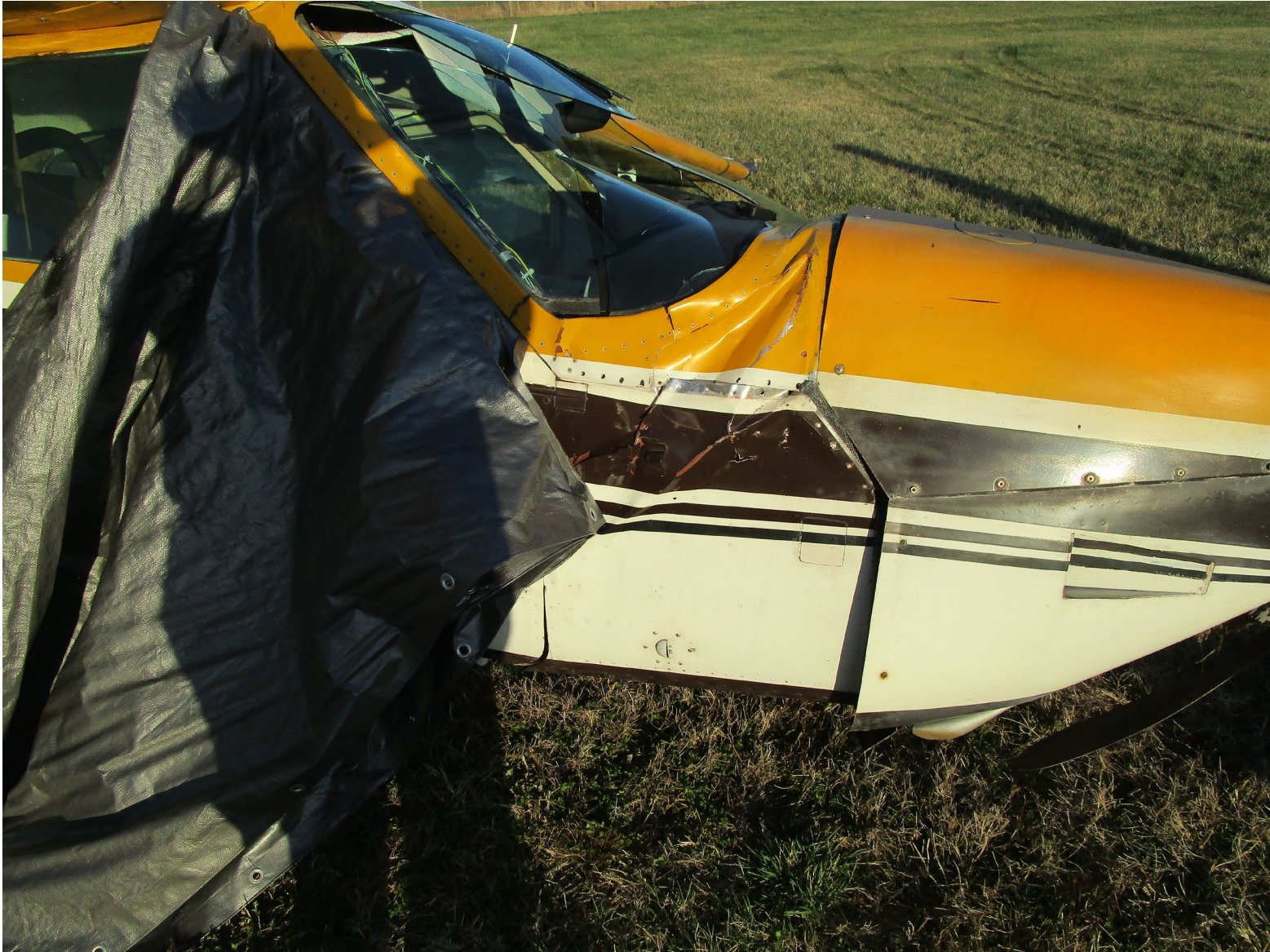
Photo 2 – Closeup of engine compartment and airframe damage. (Courtesy of FAA)
