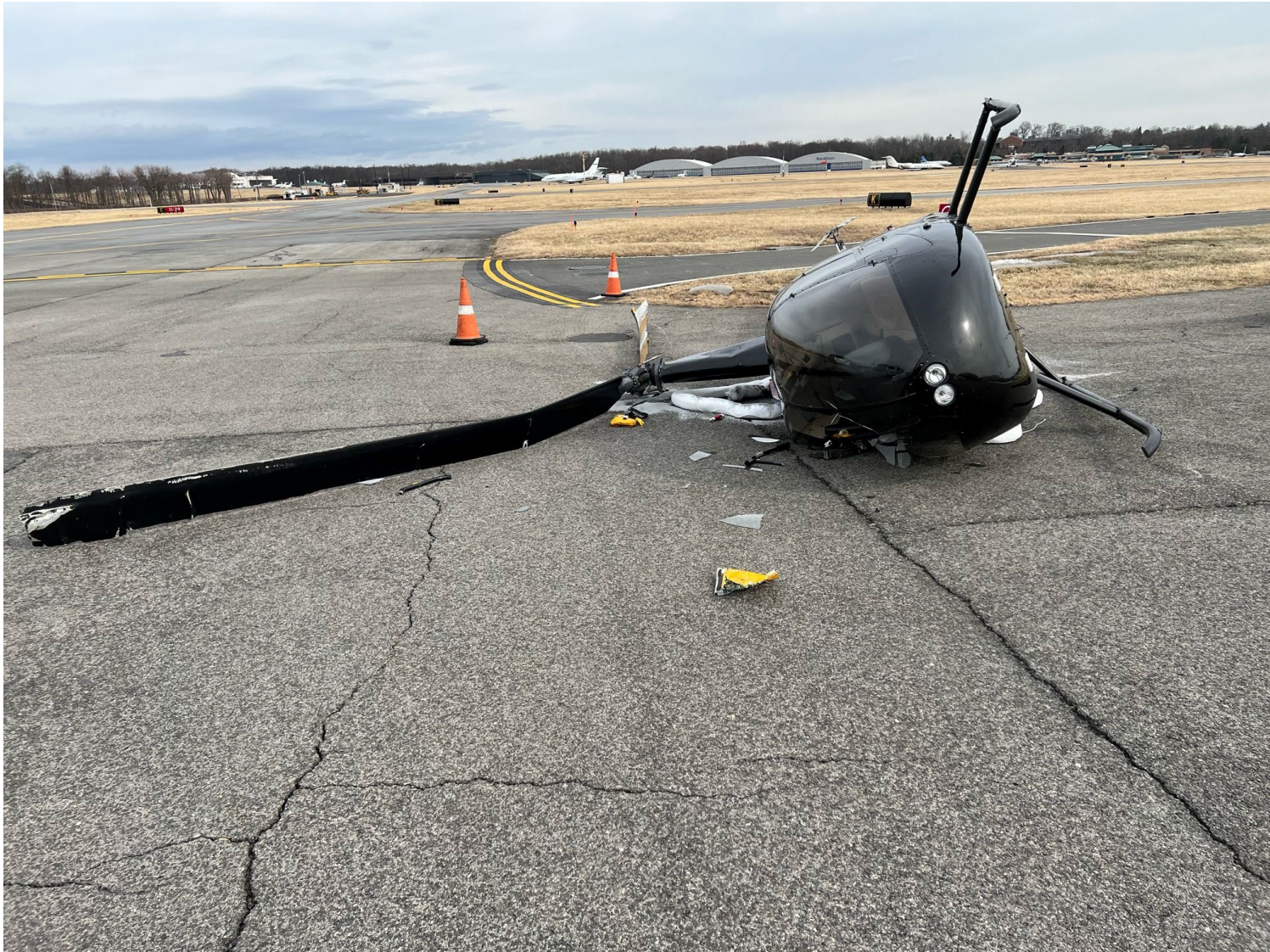
Photo 1 – View of helicopter as it rests on its right side. Note damage to rotor blades, mast, and cockpit. (Courtesy of FAA)
