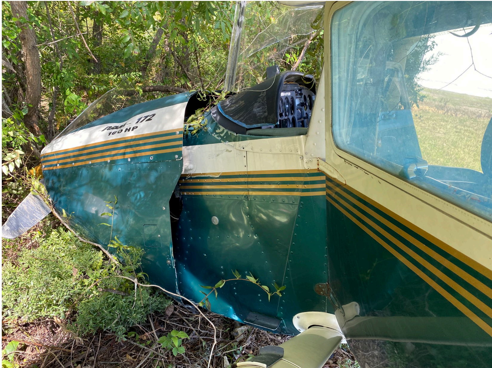
Photo 1 – Closeup view left side of cockpit showing fuselage and engine compartment damage. (Courtesy of FAA)
