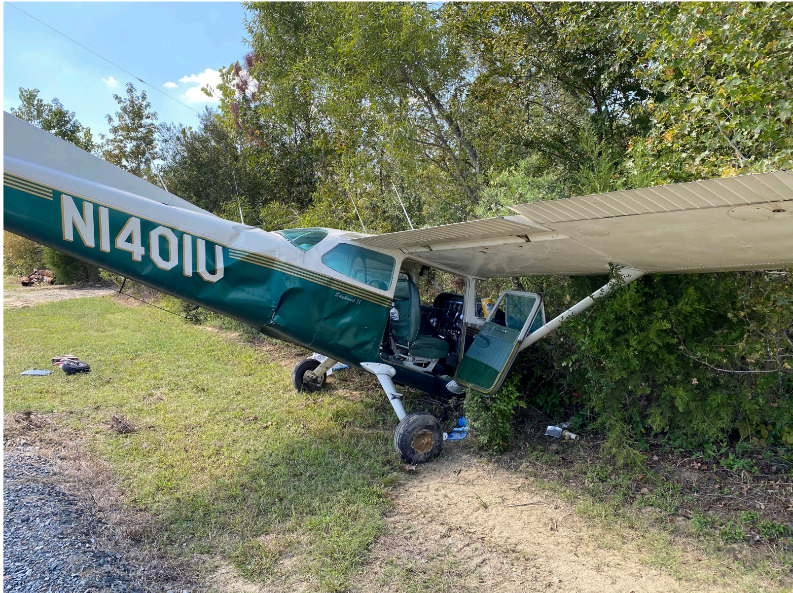
Photo 2 – Right side profile view of airplane damage. Note crumpled fuselage. (Courtesy of FAA)
