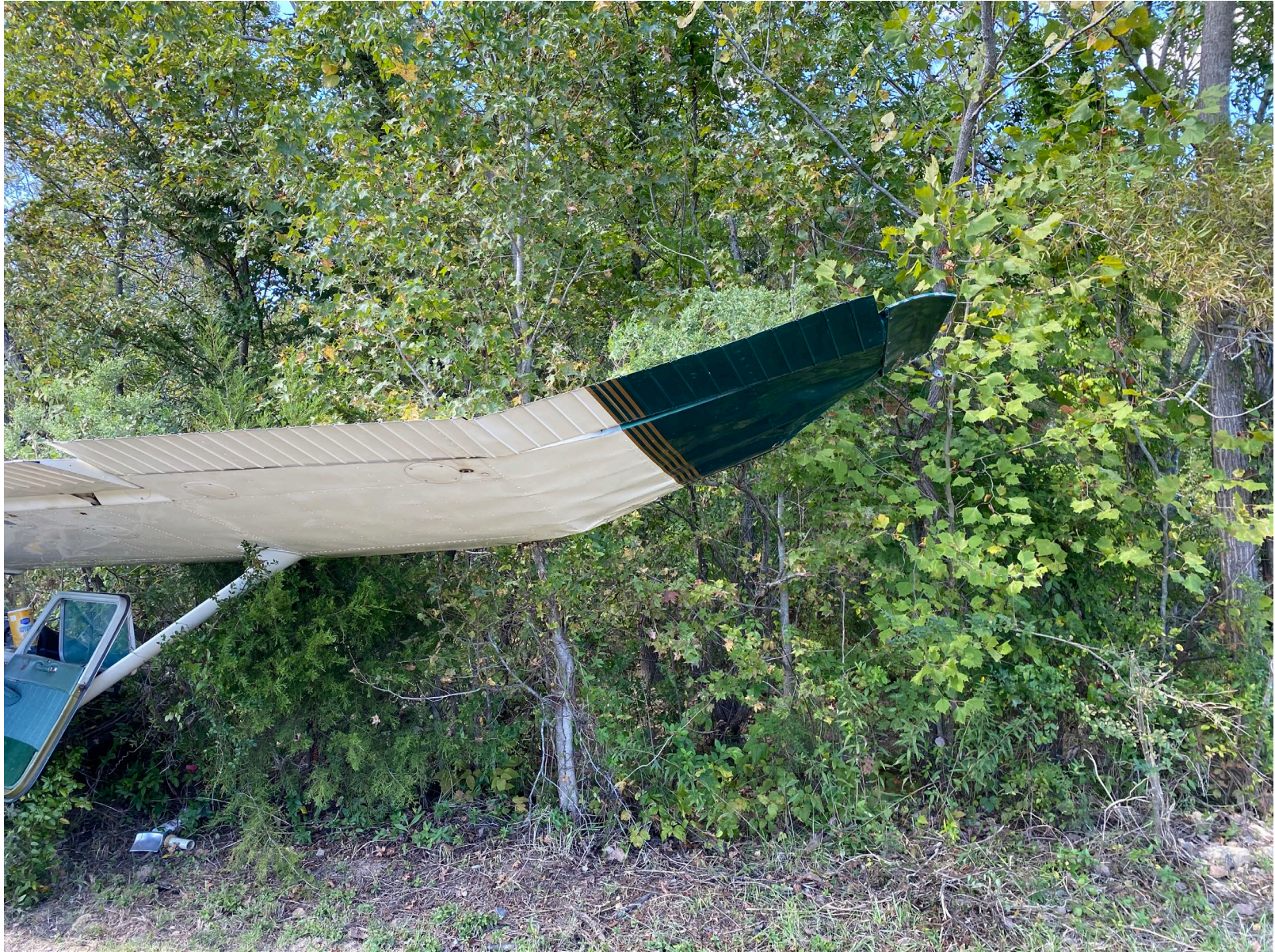
Photo 3 – Closeup photo of right wing bend upwards. (Courtesy of FAA)
