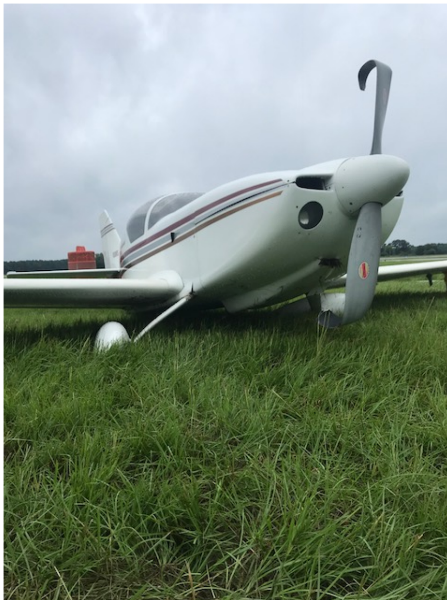
Photo 3 – View of collapsed landing gear and propeller damage. (Courtesy of FAA)
