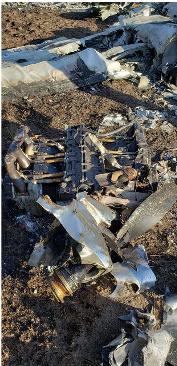
Photo 8 – View of Right Engine and Propeller Damage; Note the Engine is Detached and Upside Down.
