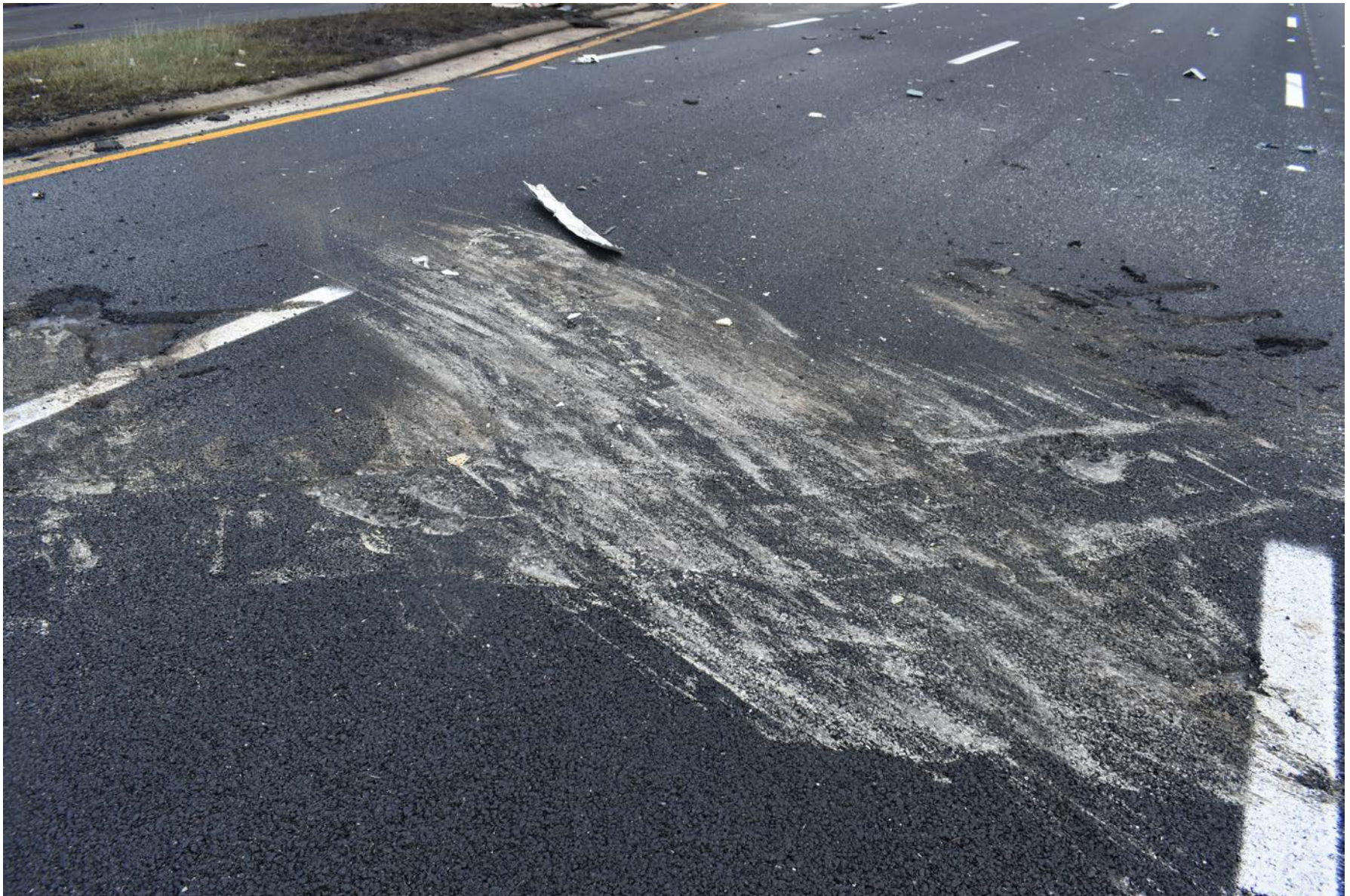
Photo 2 – Imprint of Airplane on Highway. Note Left and Right Propeller Marks in Asphalt. (Courtesy of Ocala Police)
