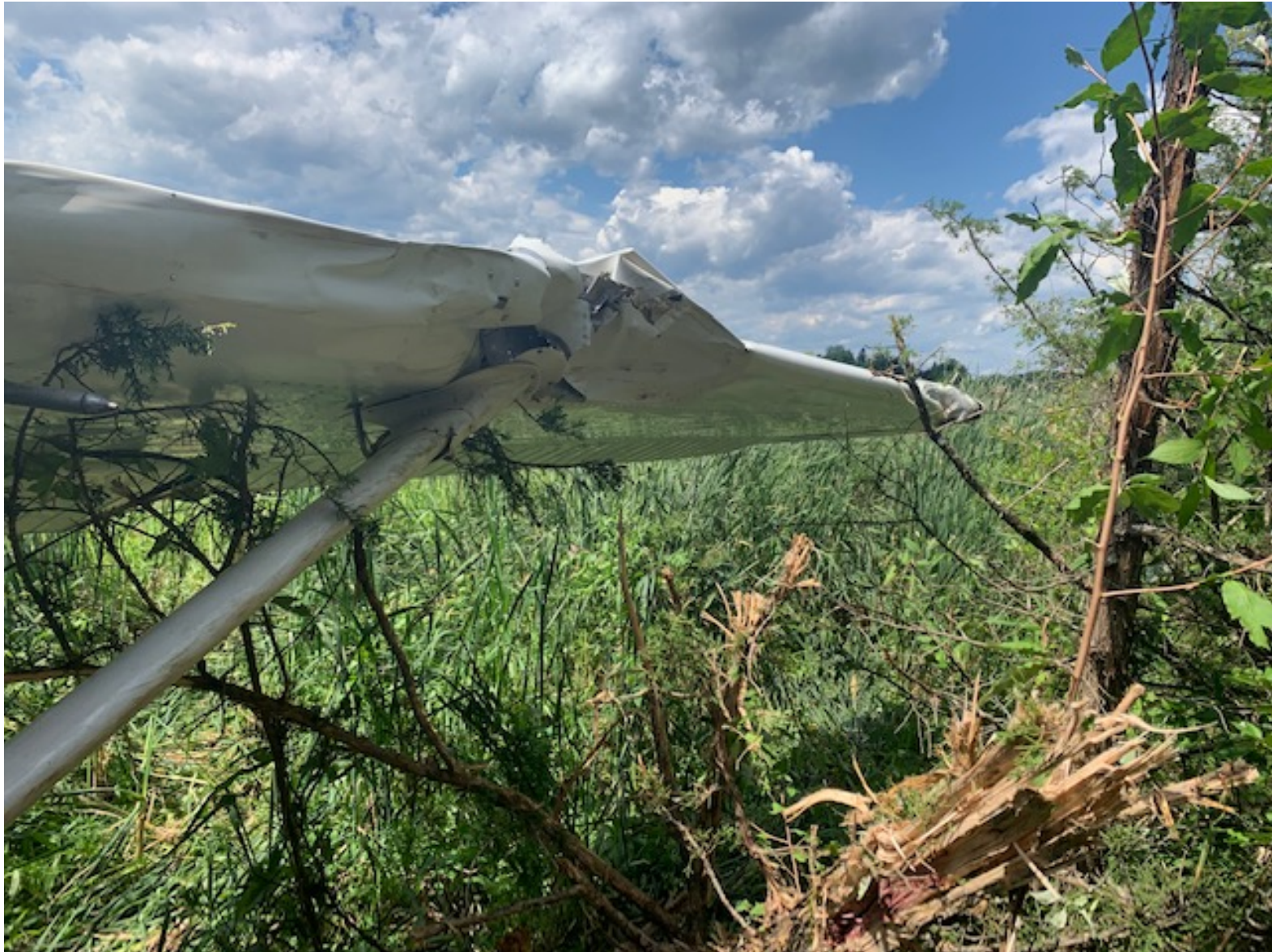
Photo 3 – Left wing leading edge and strut damage. (Courtesy of FAA)
