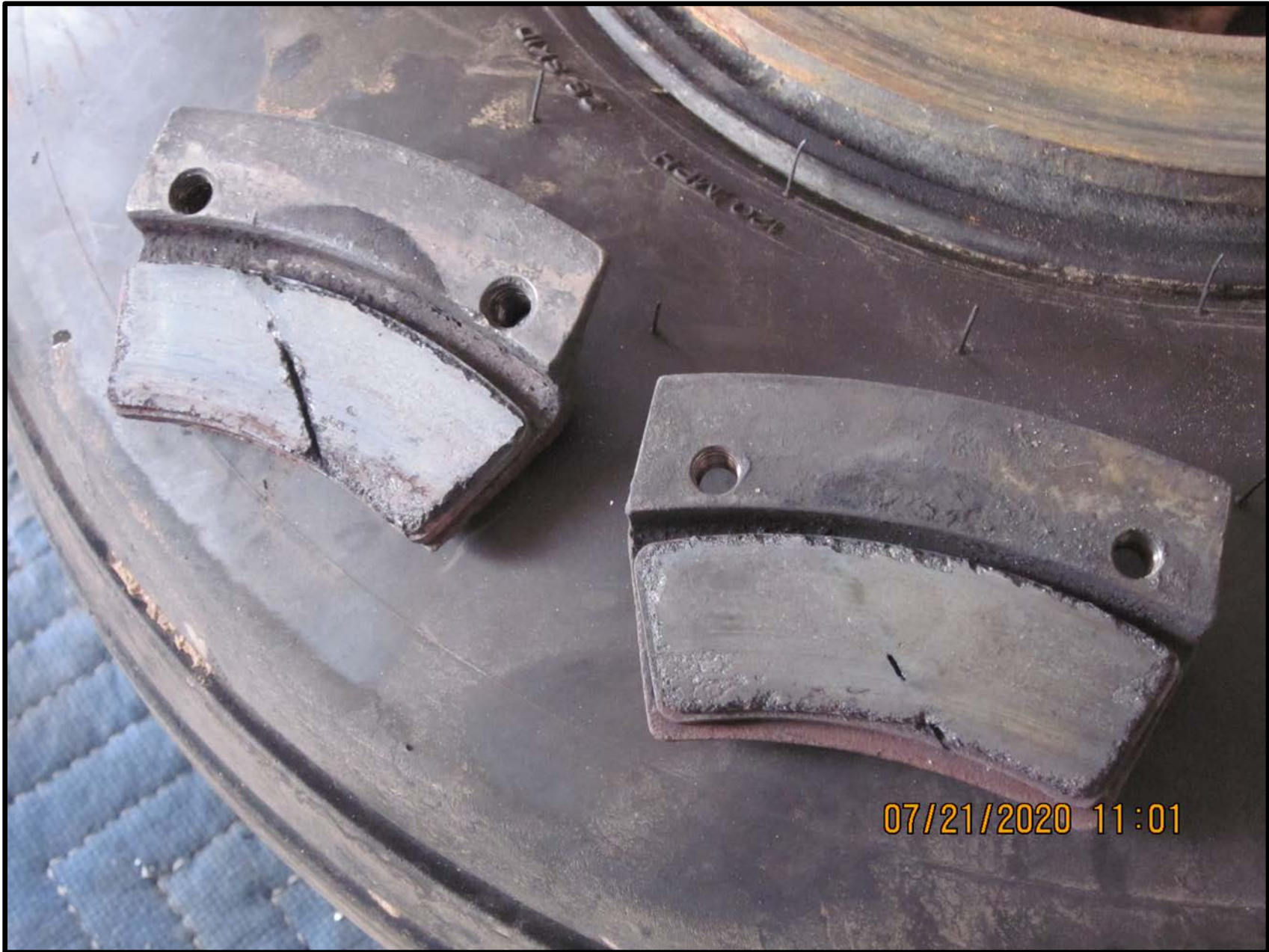
Photo 6 – Left Brake Pads (FAA Photo)
