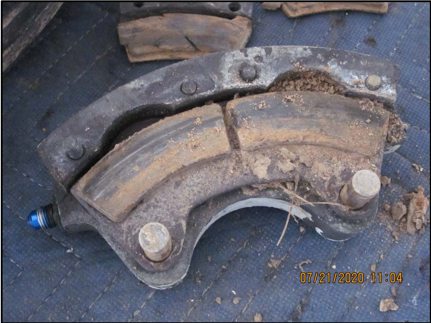
Photo 7 – Right Brake Pads (FAA Photo)
