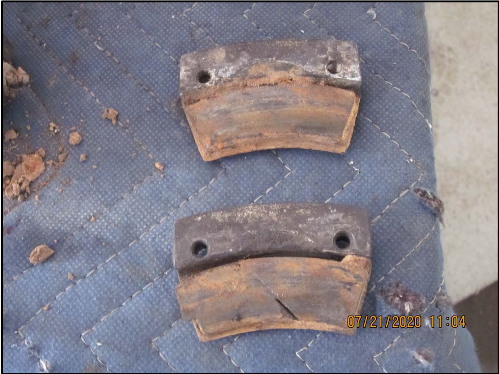
Photo 8 – Right Brake Pads (FAA Photo)
