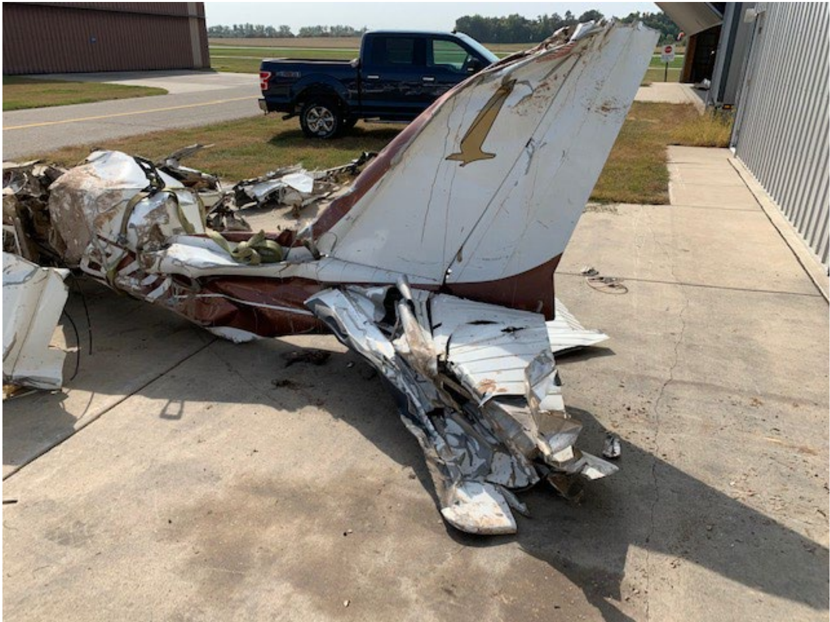
Photo 4 - Main Wreckage Layout - Empennage, Left Side (Provided by FAA)
