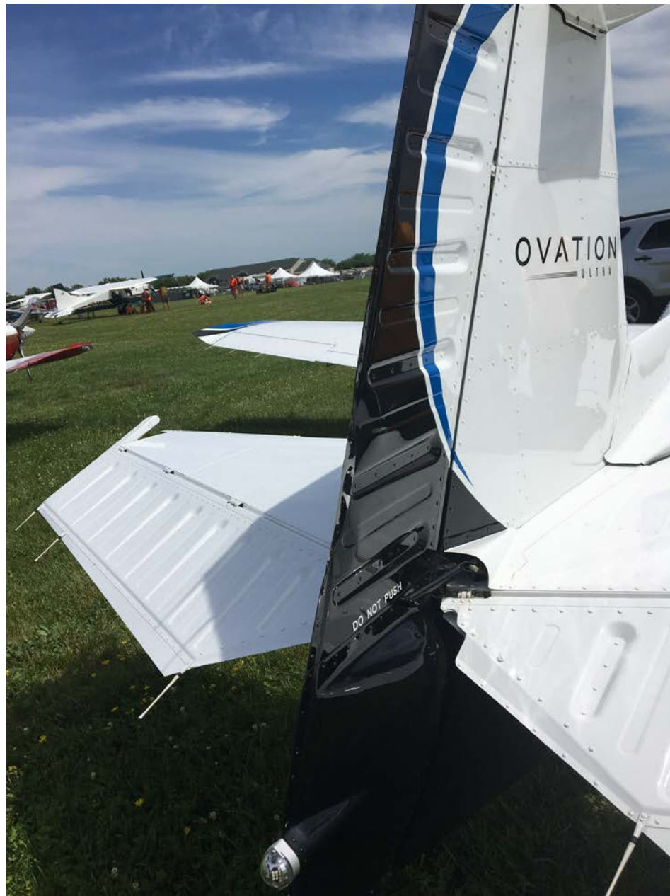
Photo 2 – Rudder damage to N197CV
